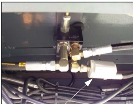
90 Micron In-Line Filter (Shown with Screen Cover removed) -Typical View
