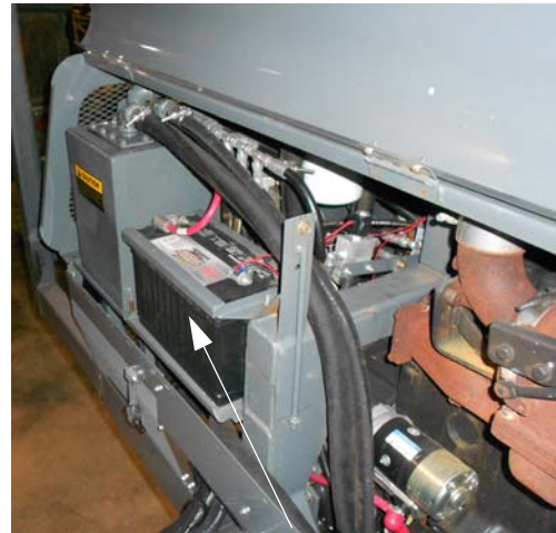
Battery Access (Located behind rear right-hand side panel) -Typical installation shown
