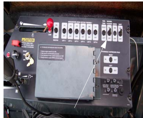
Hazard Flasher Switch (Located on side console) -Typical View
