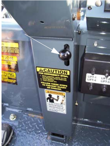
Steering Column Tilt Lock Lever (Located in center of steering column) -Typical View
