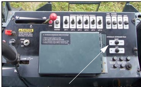
Right/Left Hydraulic Outrigger Fold Valve Switches (Located on side console) -Typical View
