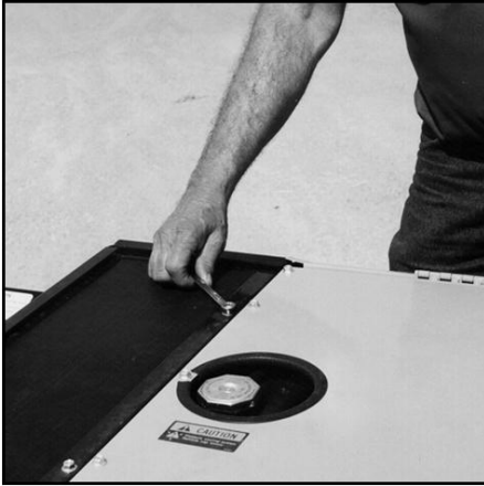
Top Grille Screen (Remove two radiator panel bolts/panel to access) -Typical View
