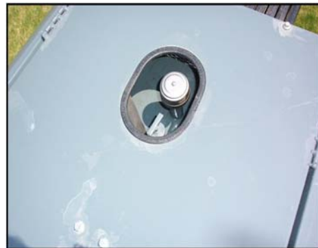
Hydraulic Oil Dipstick (Located on top of Hydraulic Oil Reservoir) -Typical View
