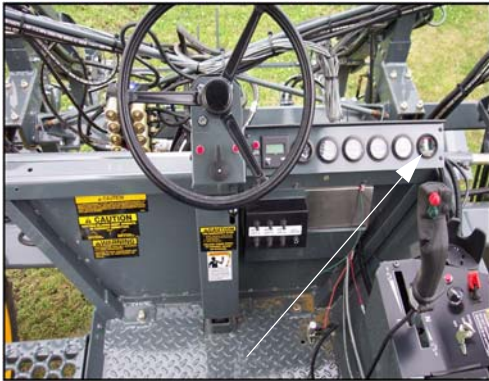
Filter Minder (Located near the operator's station) -Typical View
