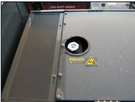
Radiator Cap (Located behind the rear of the operator's station) -Typical View
