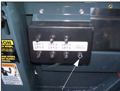
Depth Command Fuse (Located on Lift Switch Panel) -Typical View
