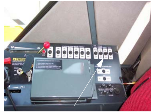
Windshield Wiper Switch (Located on side console) -Typical View
