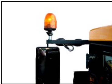
Rotating Beacon -Typical View
