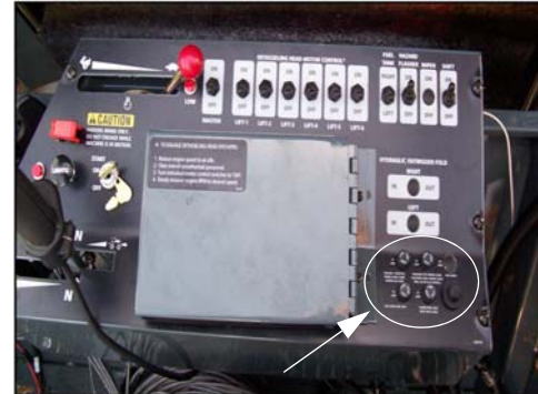
Fuses (Located on the side console) -Typical View
