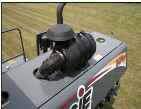
Engine Air Intake Filter (Remove air cleaner end cap to access) -Typical View
