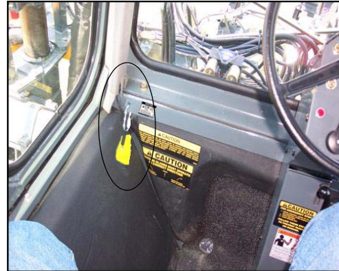
Res-Q-Me Tool (Located on left-hand side of cab) -Typical installation shown
