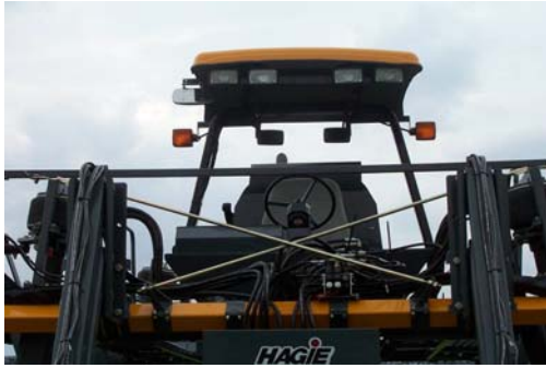
Work Lights (Located on the front and rear of the canopy or cab) -Typical View
