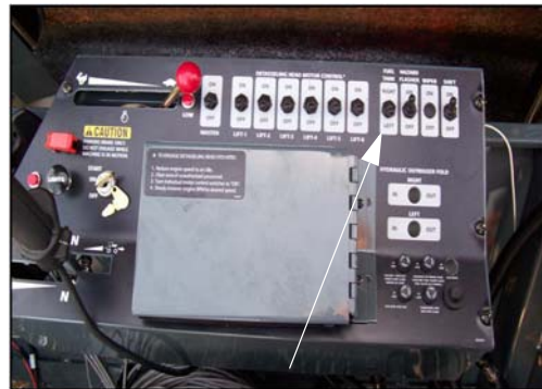
Fuel Tank Selector Switch (Located on side console) -Typical View
