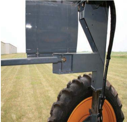
Rear Lock Nut (Located on leg brace) -Typical View
