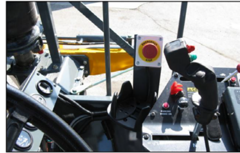
E-Stop Switch (Located near the side console) -Typical View
