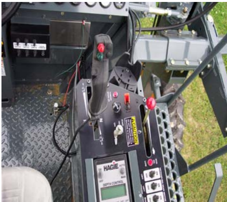
Work Lights Switch (Located on side console) -Typical View
