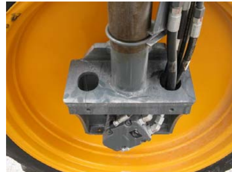
Tow Point -Typical View
