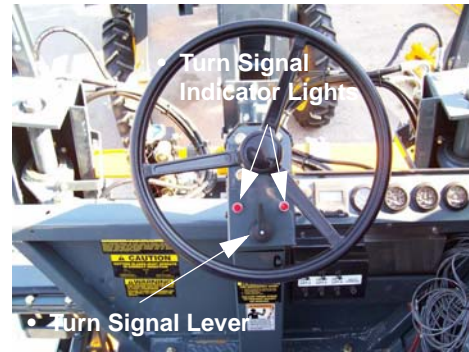
Turn Signal Lever and Indicator Lights (Located on steering column) -Typical View
