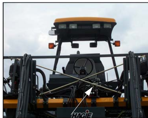
Hydraulic Fold Valve (Located on center toolbar)
