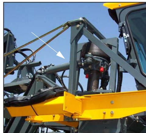
Steering Cylinders (Mounted to both of the front steering arms and outer leg weldments) -Typical View
