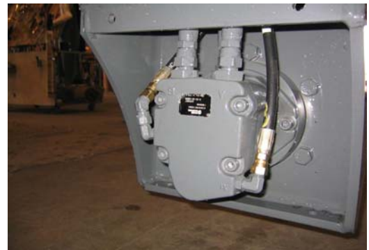
Right Rear Wheel Motor (w/Sensor)
