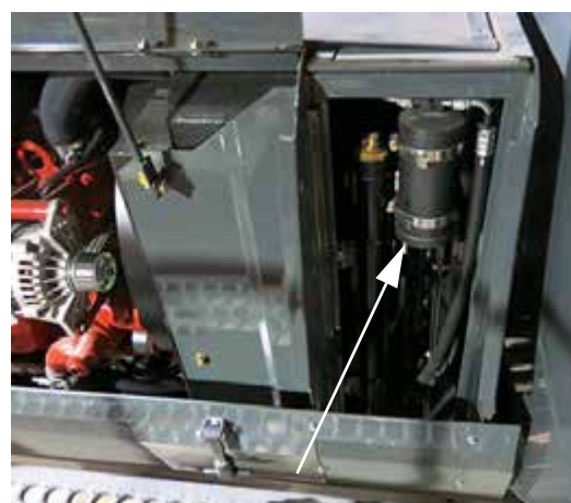
A/C System Receiver/Drier (Located behind cab near the radiator - remove radiator screens to access) -Typical View
