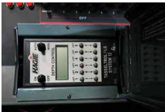
Tasselrol/LS System 12 Control Panel (Located on the side console - lift cover to access) -Typical View
