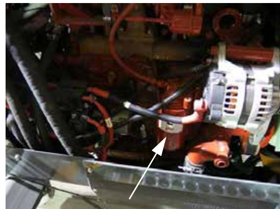
Engine Oil Filter (Located on the right-hand side of engine - open hood to access) -Typical View
