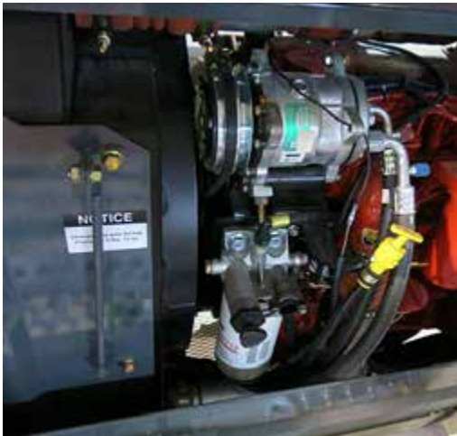
A/C Charge Port (Located on the left-hand side of machine - open hood to access) -Typical View
