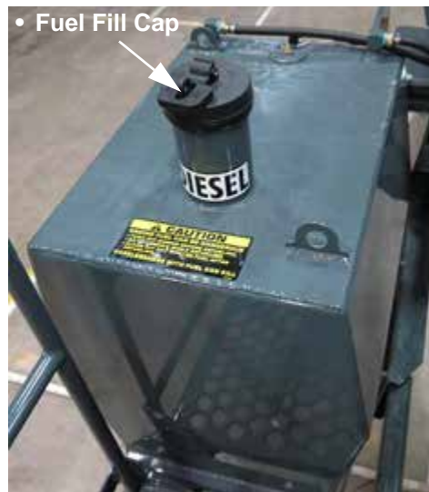
Engine Fuel Fill (Located on top of fuel tank on each side of machine) -Typical View
