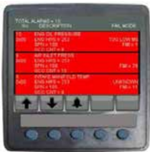
Active Alarm Screen -Typical View
