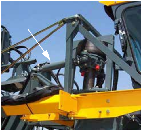
Steering Cylinders (Located on both of the front steering arms and outer leg weldments) -Typical View
