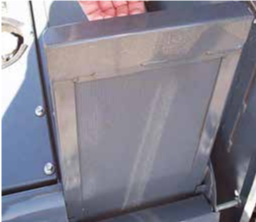
Side Grille Screen (Slide out of radiator housing to remove) -Typical View
