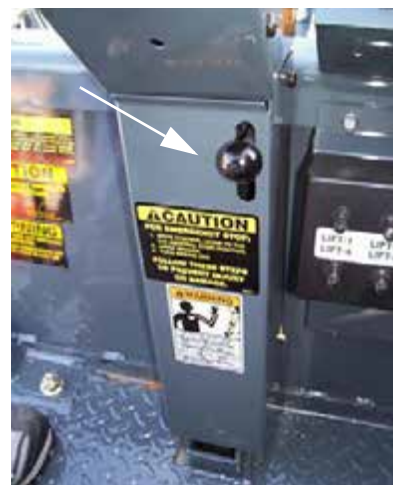
Steering Column Tilt Lock Lever (Located near center of steering column) -Typical View
