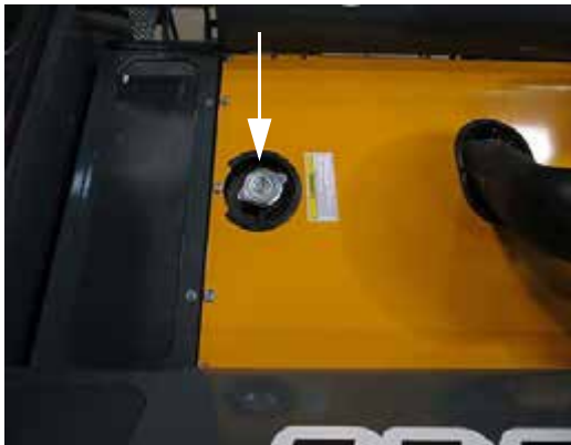
Radiator Cap (Located behind the operator’s station) -Typical View
