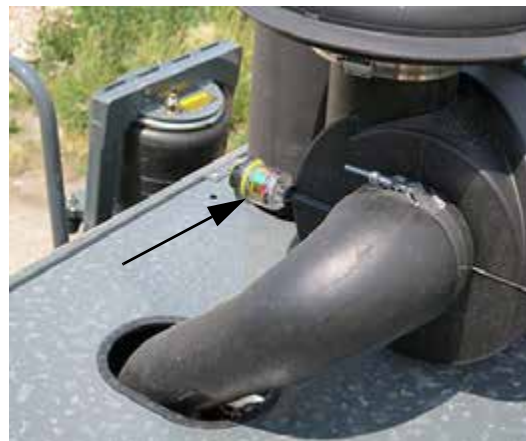
Filter Minder (Located near engine air intake filter housing) -Typical View
