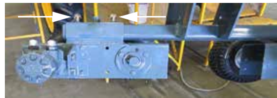
Quad Puller Bolts (Located on each Quad Puller Mounting Tube) -Typical View
