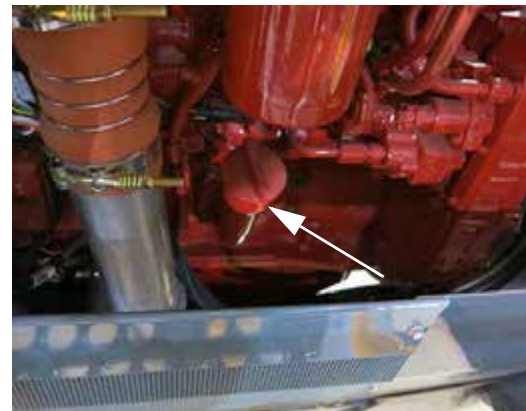
Remote Engine Oil Fill Port (Located on the left-hand side of engine - open hood to access) -Typical View
