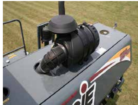
Engine Air Intake Filter (Located near rear of machine - remove air cleaner end cap to access) -Typical View
