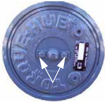
Cap Bolts -Typical View
