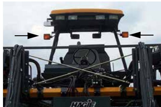
Highway Running Lights (Located on each side of operator's station) -Typical View
