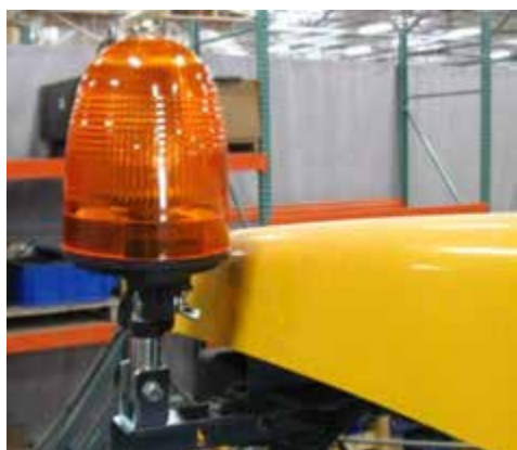
Rotating Beacon (Located on the left-hand side of the operator’s station) -Typical View
