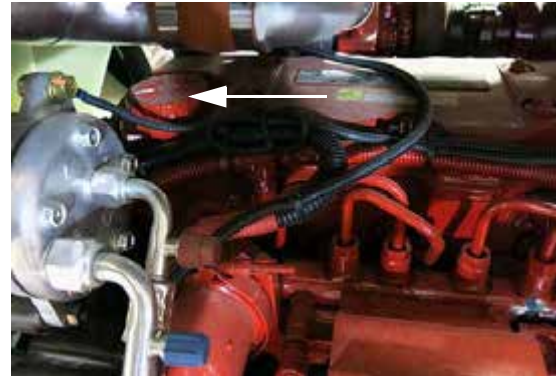
Engine Oil Fill Port (Located on the left-hand side of engine - open hood to access) -Typical View
