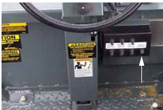
Depth Command Fuse (Located on the Depth Command Switch Panel near front of operator’s station) -Typical View
