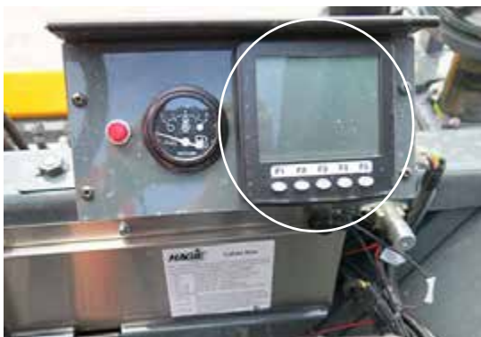
Engine Monitor Display (Located near the front of operator's station) -Typical View
