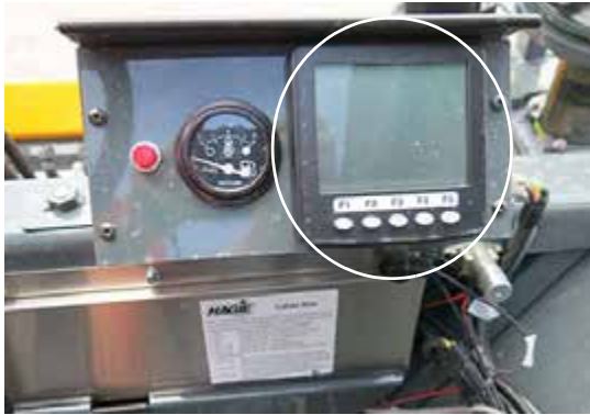
Engine Monitor (Located near the front of operator's station) -Typical View
