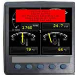
Active Fault Warning -Typical View
