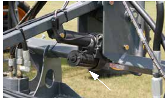
Depth Command Actuator (Located on the tool bar lift head tube) -Typical View
