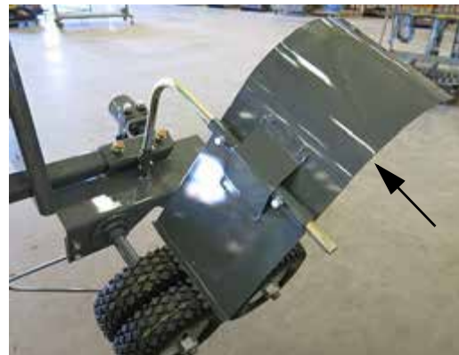
Deflector Shield -Typical View
