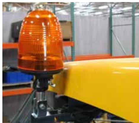
Rotating Beacon (Located on the left-hand side of the operator’s station) -Typical View
