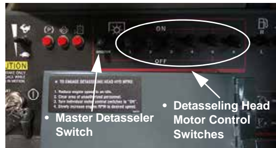
Master Detasseler and Detasseling Head Motor Control Switches (Located on the side console) -Typical View
