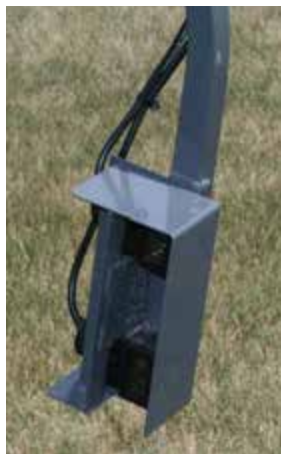
Photo Light Sensor -Typical View
