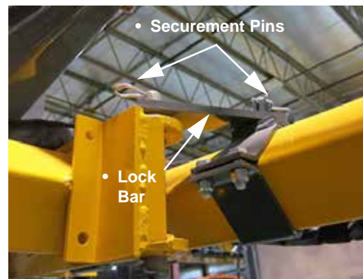
Securement Pin/Lock Bar Assembly (Located between the outrigger and center tool bar) -Typical View
