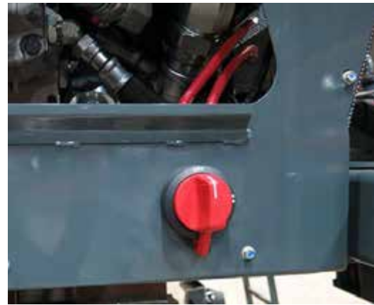
Battery Disconnect Switch (Located on the rear frame) -Typical View
