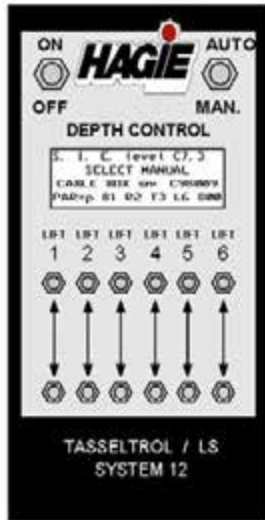
Tasselrol Control Panel (Located on the side console - lift panel to access) -Typical View
