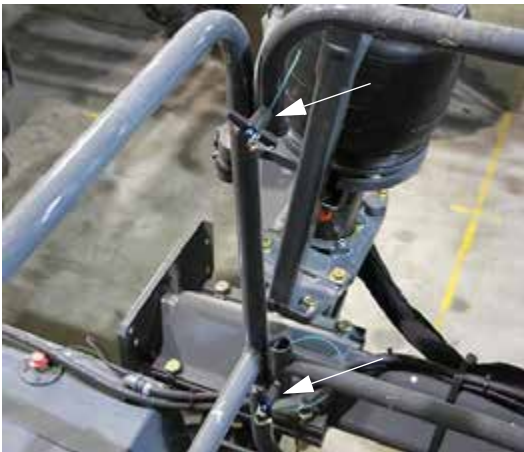
Handrail Pins (Located on the top and bottom of handrail extension) -Typical View
