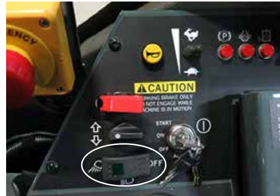
Lights Switch (Located on the side console) -Typical View
