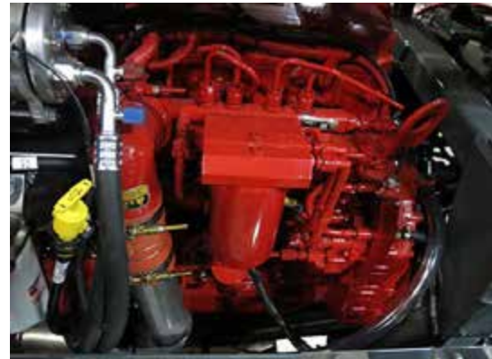
A/C Charge Ports (Located on the left-hand side of machine - open hood panel to access) -Typical View
