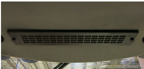
Fresh Air Cab Filter Access (Located in cab headliner) -Typical View
