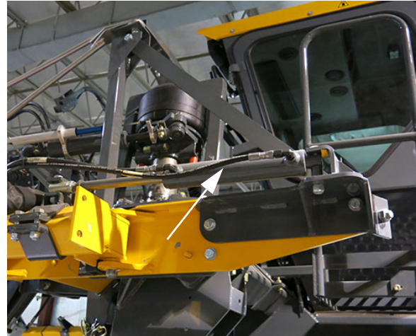
Hydraulic Fold Cylinder (Attached to outrigger and center tool bar) -Typical View
