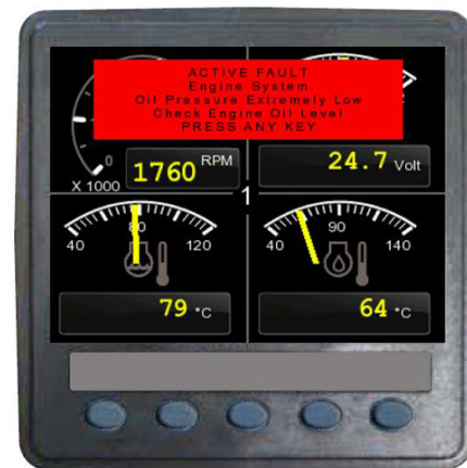
Active Fault Warning -Typical View
