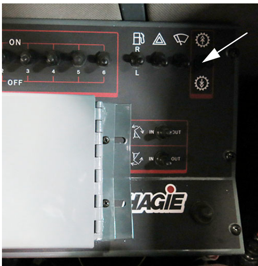
Gear Selector Switch (Located on the side console) -Typical View
