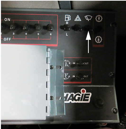
Wiper Switch (Located on the side console) -Typical View
