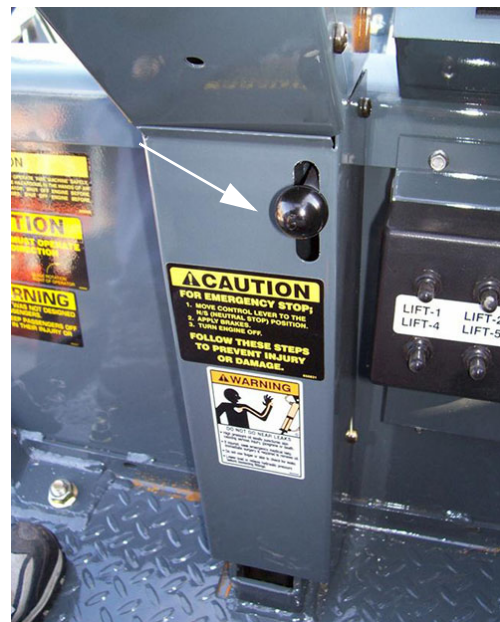
Steering Column Tilt Lock Lever (Located near center of steering column)
