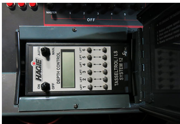
Tasselrol/LS System 12 Control Panel (Located on the side console - lift cover to access) -Typical View
