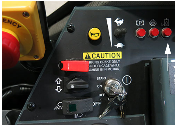
Low Hydraulic Oil Indicator (Located on the side console) -Typical View
