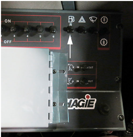
Fuel Tank Selector Switch (Located on the side console) -Typical View
