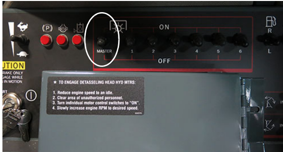
Master Detasseler Switch (Located on the side console) -Typical View
