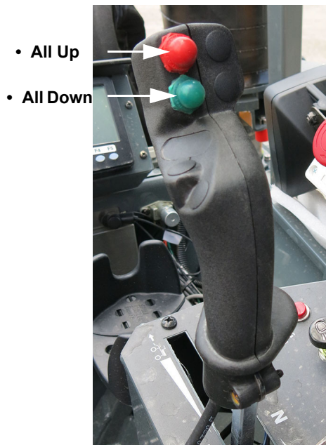
All Up/Down Switches (Located on the Hydrostatic Drive Control Handle) -Typical View
