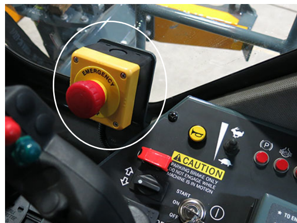
E-Stop Switch (Located near the side console) -Typical View
