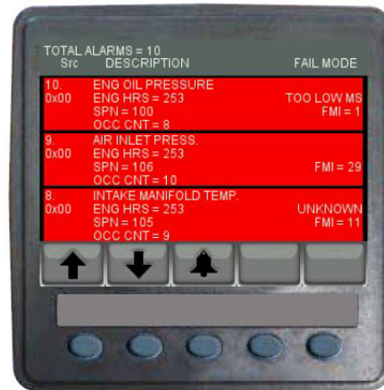
Active Alarm Screen -Typical View
