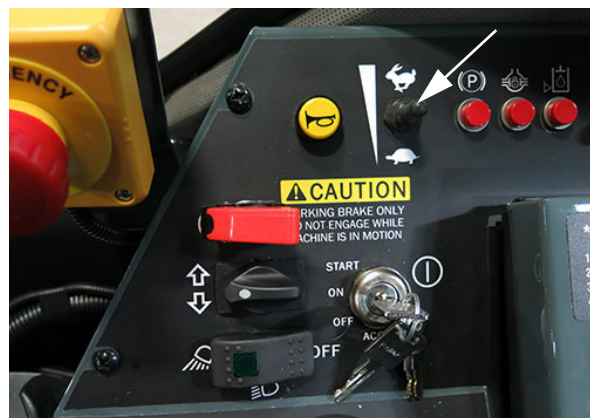
Throttle Switch (Located on the side console) -Typical View
