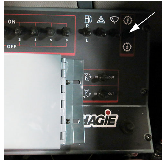
Gear Selector Switch (Located on the side console) -Typical View
