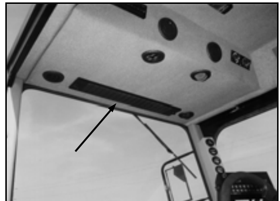
CAB FILTER LOCATION FIG 8.32
