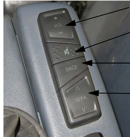
Remote Stereo Controls (Located near the Hydrostatic Drive Control Handle) -Typical View
