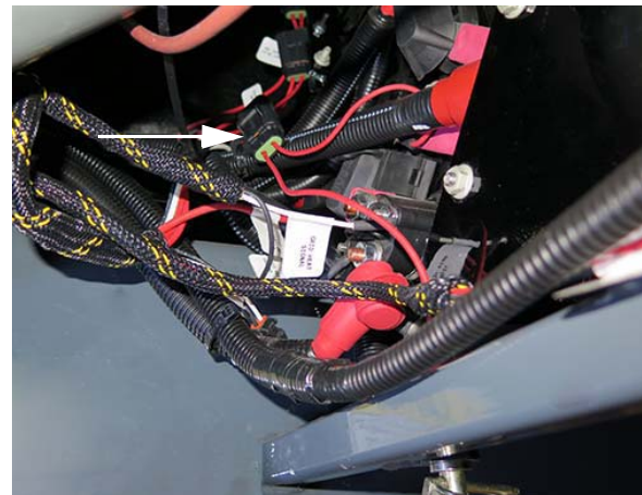
Hood Actuator Fuse (Located beneath rear right-hand side of machine) -Typical View Remove rear panel and brush curtain to access if equipped with Tall Crop Package
