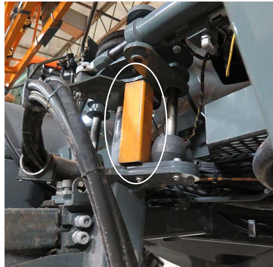
Steel Tube Installed Beneath Air Bag Mounting Plate -Typical View
