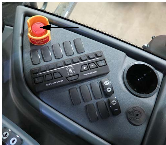
E-Stop Switch (Located on the side console) -Typical View
