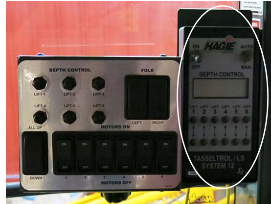
Tasselrol/LS System 12 Control Panel -Typical View
