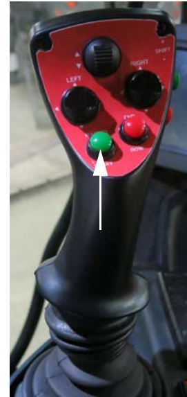
Main Control Switch (Located on the Hydrostatic Drive Control Handle) -Typical View
