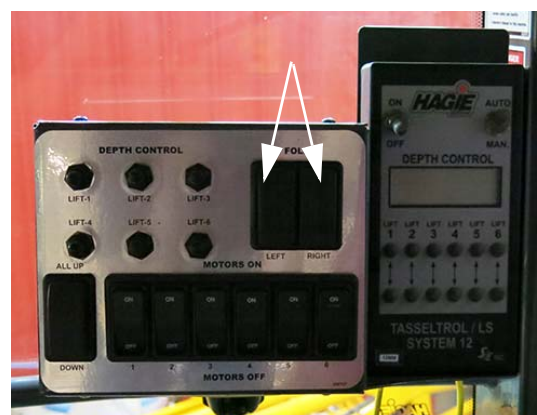
Out-igger Fold Switches - Left/Right (Located on the detasseling control panel) -Typical View
