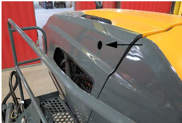
Coolant Sight Gauge (Located on the right-hand side of hood) -Typical View
