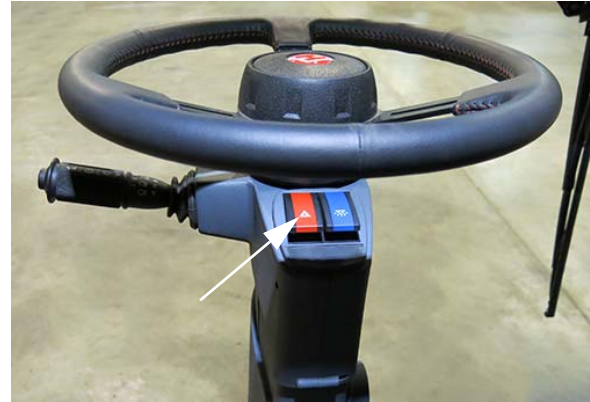
Hazard/Warning Lights Switch (Located on steering column) -Typical View
