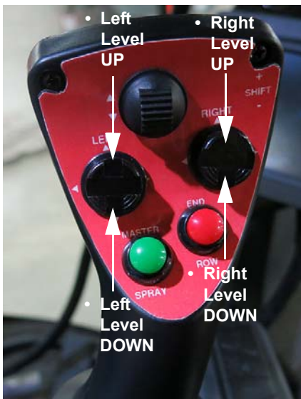
Level Switches - Left/Right (Located on the Hydrostatic Drive Control Handle) -Typical View
