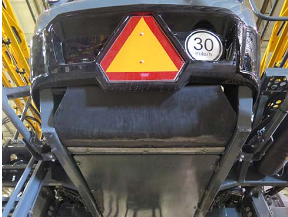
Brush Curtain Installation -Typical View
