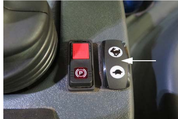
Throttle Switch (Located near the Hydrostatic Drive Control Handle) -Typical View
