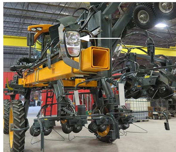
Highway Running Lights (2) -Typical View
