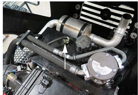
Level/Temp Sensor (Located on top of hydraulic oil reservoir - open hood to access) -Typical View
