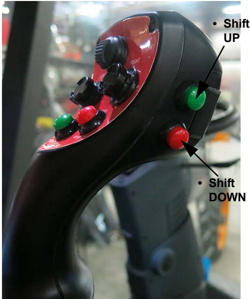
Shift Up/Down Switches (Located on the side of the Hydrostatic Drive Control Handle) -Typical View
