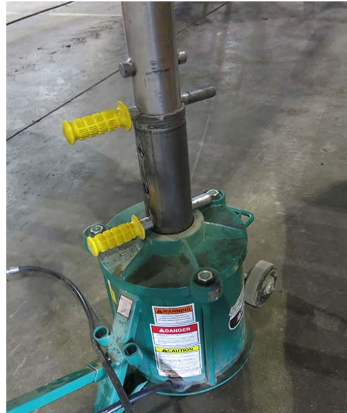
Lock Pin Installation -Typical View
