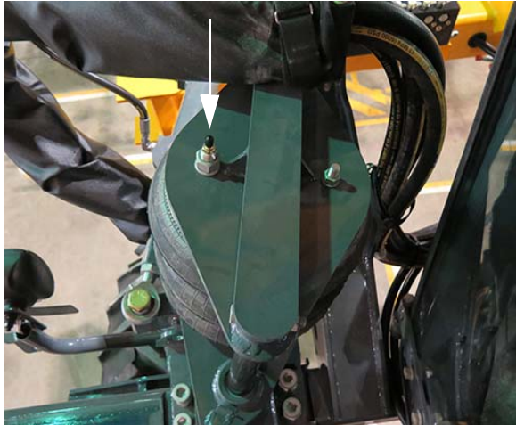
Air Bag Valve Stem (Located on top of each air bag) -Typical View
