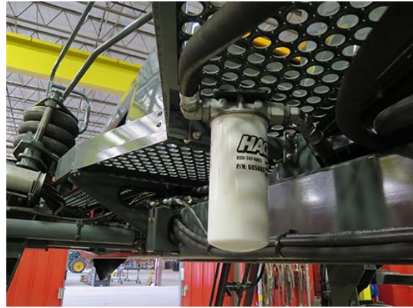
Return Filter 2 (Located beneath platform on right-hand side of machine) -Typical View
