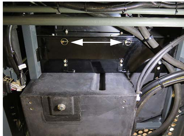
Spring Clips (2) - Access Panel (Located on the Hydraulic Oil Cooler Screen Access Panel beneath center of machine) -Typical View
