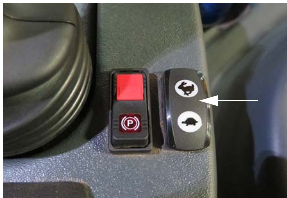
Throttle Switch (Located near the Hydrostatic Drive Control Handle) -Typical View
