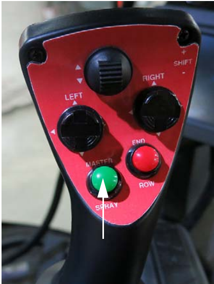
Main Control Switch (Located on the Hydrostatic Drive Control Handle) -Typical View
