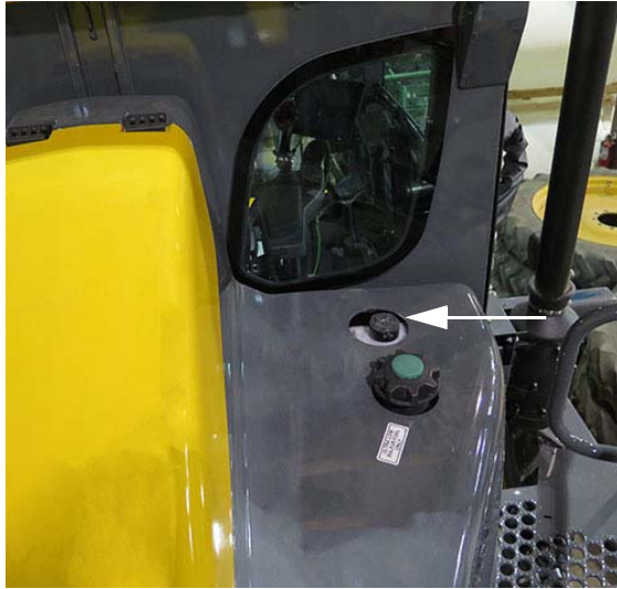
Windshield Washer Fluid Reservoir Fill (Located on top of the right-hand FRM) -Typical View
