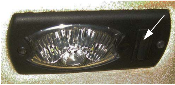
Interior Work Light Switch -Typical View
