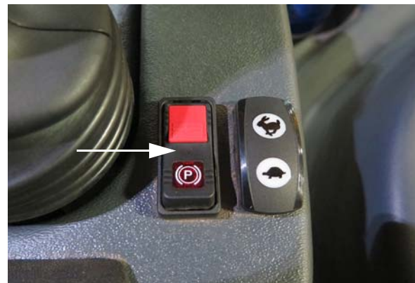
Parking Brake Switch (Located near the Hydrostatic Drive Control Handle) -Typical View
