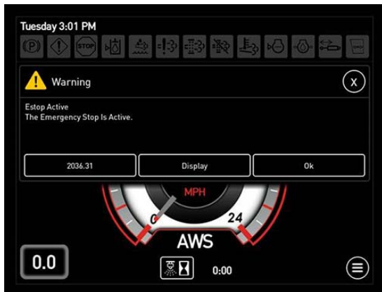
E-Stop Active Warning Message (Located on the Machine Display)
