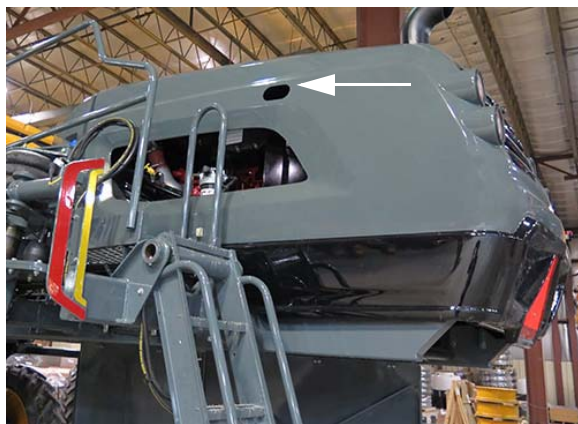
Hydraulic Oil Reservoir Sight Gauge (Located near the rear left-hand side of machine) -Typical View
