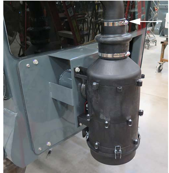
Flange Clamp - Top (Located near the top of the RESPA filtration unit) -Typical View
