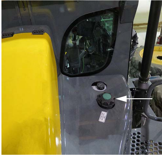
Fuel Fill Cap (Located on top of fuel-rinse module) -Typical View
