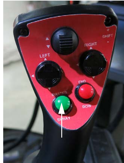
Main Control Switch (Located on the Hydrostatic Drive Control Handle) -Typical View
