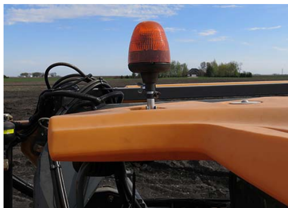
Rotating Beacon (Located on front roof cap) -Typical View
