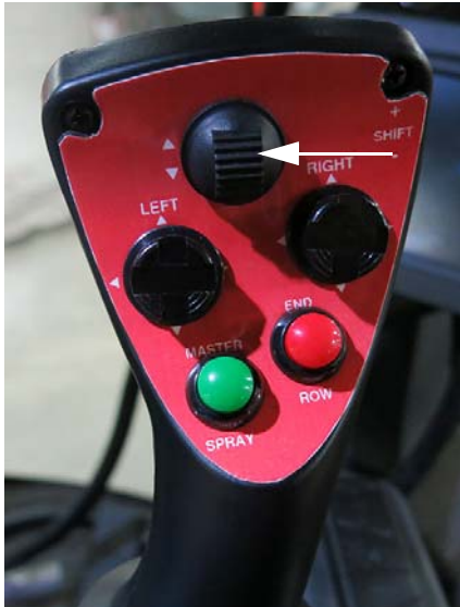
All Up/Down Switch (Located on the Hydrostatic Drive Control Handle) -Typical View
