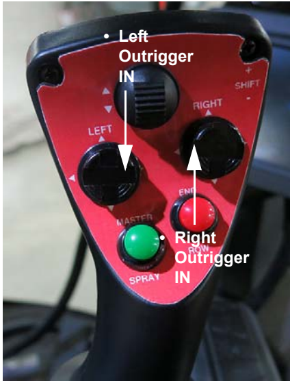
Outrigger Fold Switches - Left/Right (Located on the Hydrostatic Drive Control Handle) -Typical View
