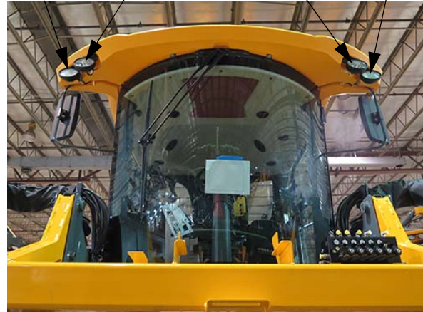
Field Lights (4) (Located on the front of cab) -Typical View
