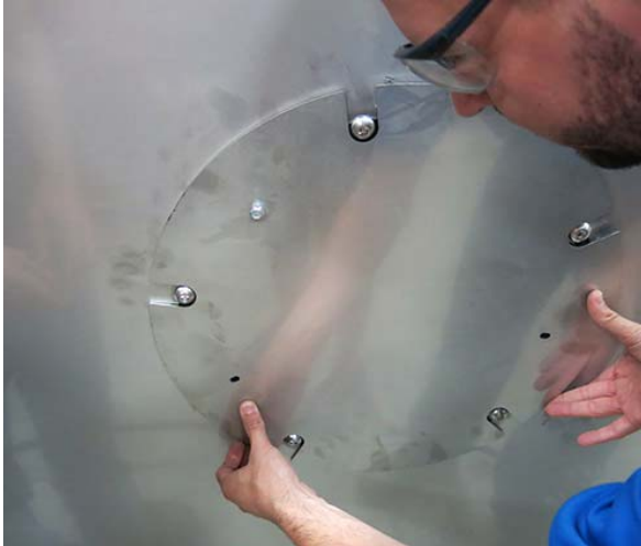
Hub Cap Access Panel -Typical View
