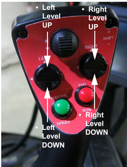
Level Switches - Left/Right (Located on the Hydrostatic Drive Control Handle) -Typical View
