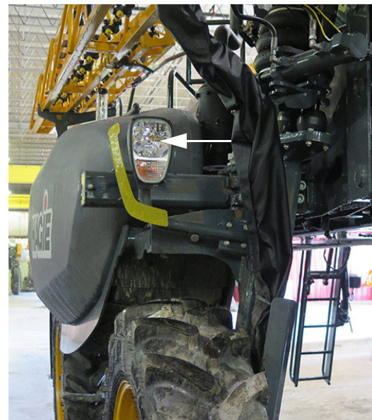
Highway Running Lights (2) -Typical View
