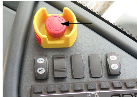
E-Stop Switch (Located on the side console) -Typical View
