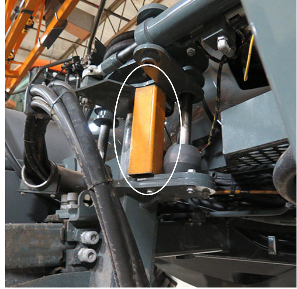
Steel Tube Installed Beneath Air Bag Mounting Plate -Typical View
