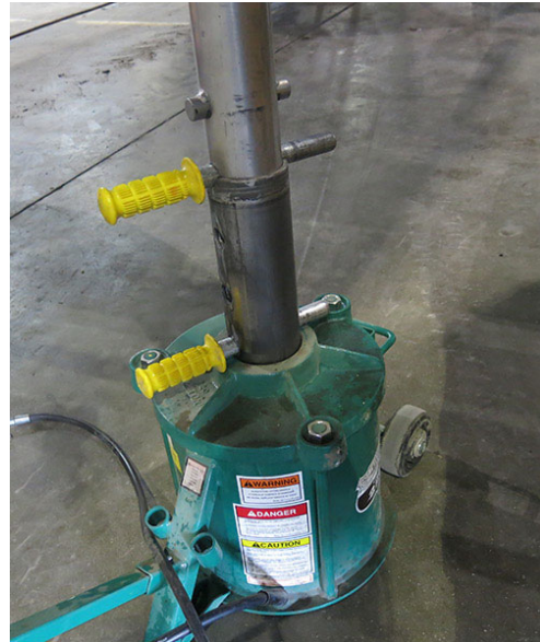
Lock Pin Installation -Typical View
