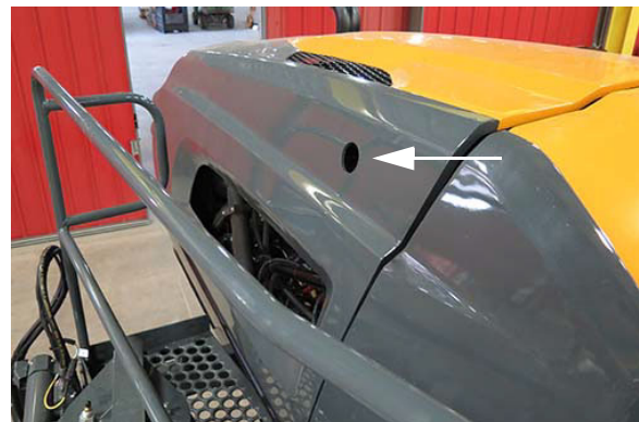
Coolant Level Sight Gauge (Located on the rear right-hand side of machine) -Typical View
