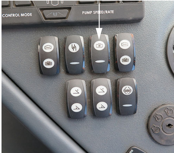
Agitation Valve Switch (Located on the side console) -Typical View
