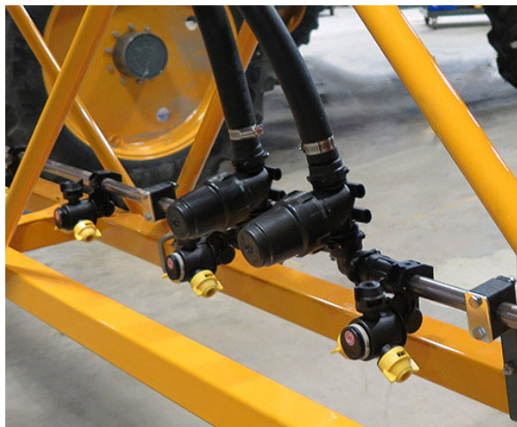
Section Strainers (Located throughout each boom section) -Typical View
