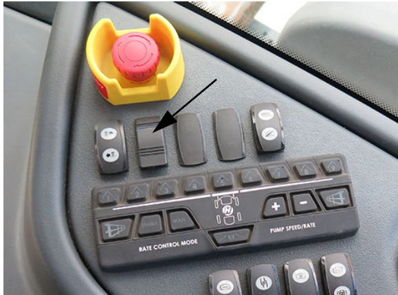
Night Spray Switch (Located on the side console) -Typical View
