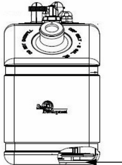
DEF Suction Strainer (Located near bottom of the DEF Tank) -Typical View
