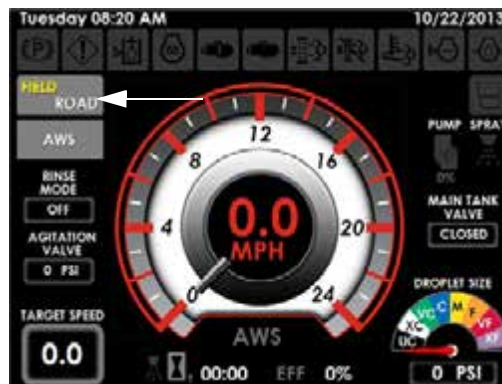
Field/Road Button (Located on the Machine Display Home Page - Road and Field Mode)
