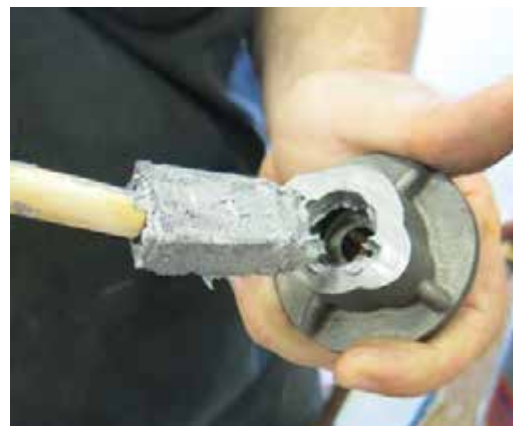
Anti-Seize Lubricant Application -Typical View
