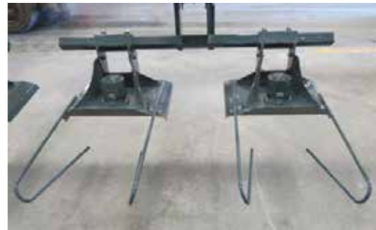
Stalk Guide Installation -Typical View
