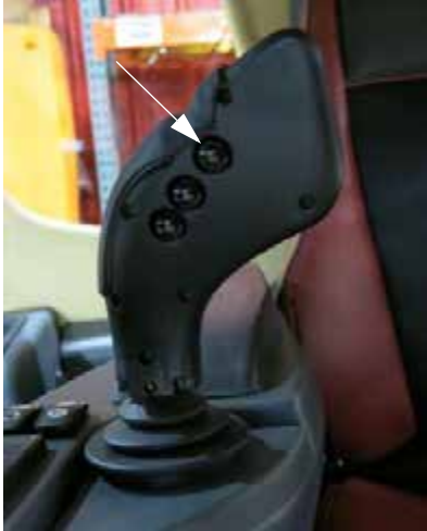
Main Control Switch (Located on the back side of the Hydrostatic Drive Control Handle) -Typical View
