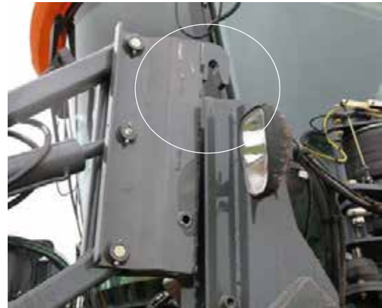
Attachment Clearing Mounting Pin -Typical View
