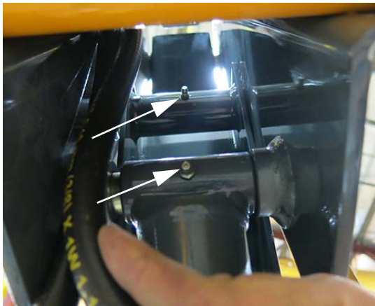
Lift Arm Assembly - Inner Arm -Typical View
