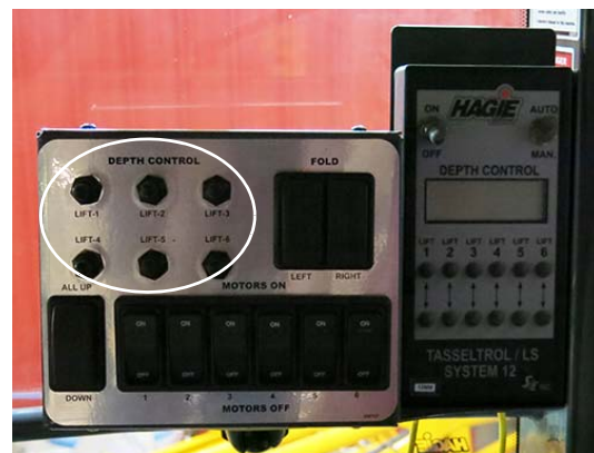
Depth Control Switches (Located on the detasseling control panel) -Typical View
