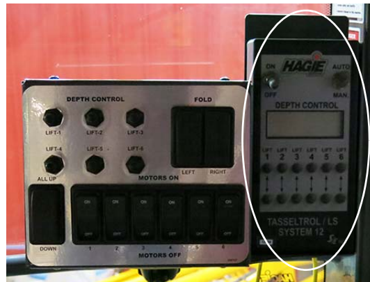
Tasselrol/LS System 12 Control Panel -Typical View
