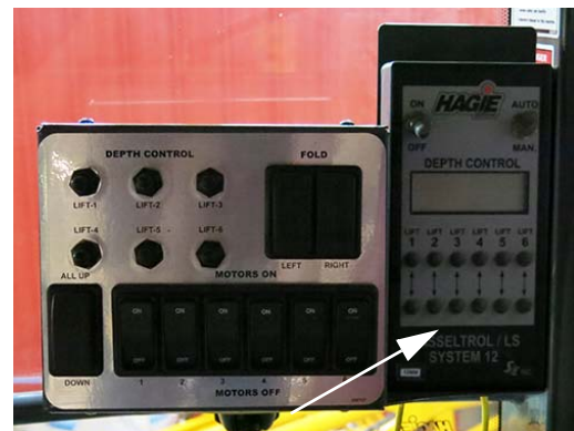
Tasselrol/LS System 12 Control Panel -Typical View
