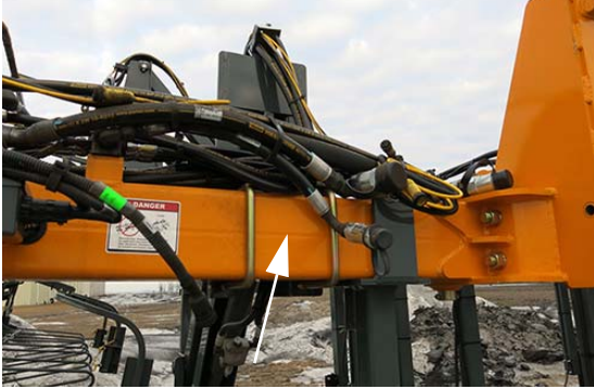
DTB Attachment Serial Number (Located on the main tool bar) -Typical View
