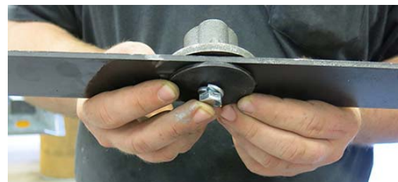
Cutter Blade Assembly -Typical View
