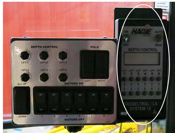
Tasselrol/LS System 12 Control Panel -Typical View
