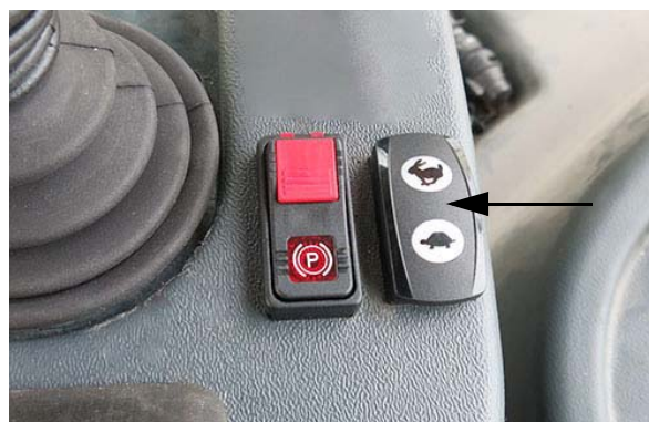
Throttle Switch (Located near the Hydrostatic Drive Control Handle) -Typical View
