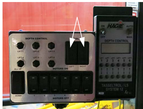
Outrigger Fold Switches - Left/Right (Located on the detasseling control panel) -Typical View
