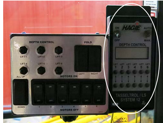
Tasselrol/LS System 12 Control Panel -Typical View
