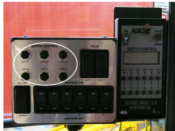
Depth Control Switches (Located on the detasseling control panel) -Typical View
