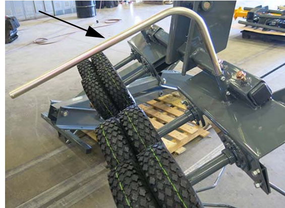
Deflector Shield Mounting Tube -Typical View
