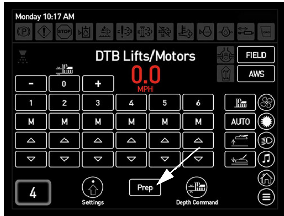
Prep Button (Located on the Machine Display DTB Lifts/Motors Screen or DTB Depth Command Screen)
