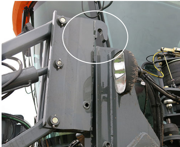
Attachment Clearing Mounting Pin -Typical View
