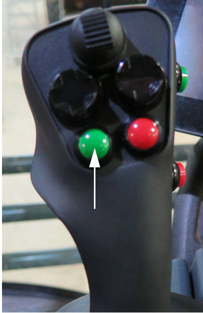
Main Motor Switch (Located on the Hydrostatic Drive Control Handle) -Typical View
