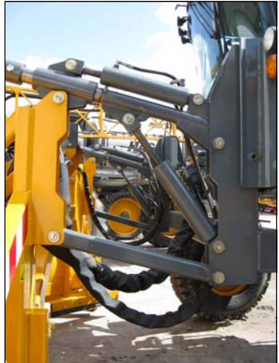
Make sure the hooks are fully engaged
