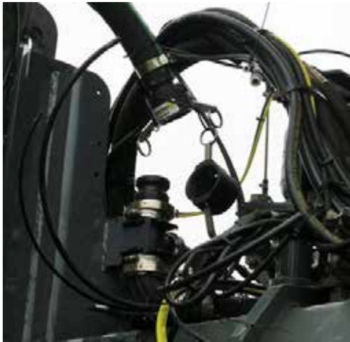
Solution Connection (Located on front right-hand side of machine) -Typical View
