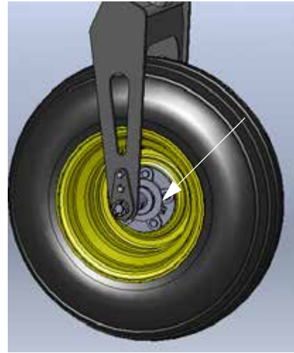
Grease Point F (Left-hand side shown)
