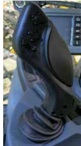
Hydrostatic Drive Control Handle -Typical View
