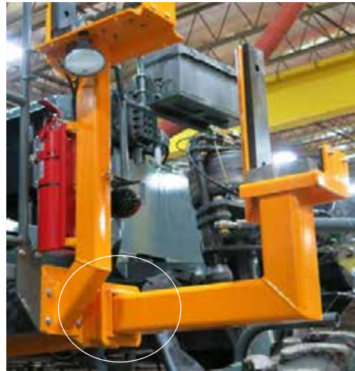
Cradle Receptacle (Located near boom cradle on side of machine) -Typical View
