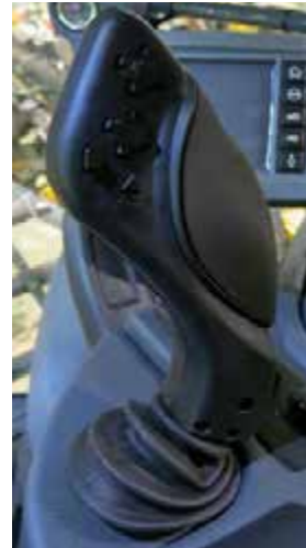
Hydrostatic Drive Control Handle -Typical View
