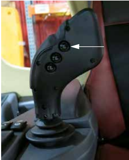
Master Spray Switch (Located on the back side of the Hydrostatic Drive Control Handle) -Typical View
