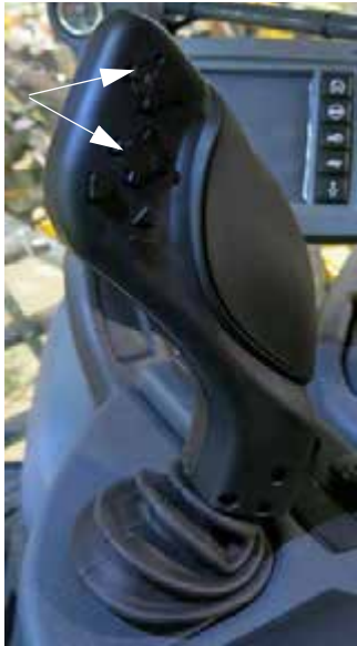
Left and Right Boom/NTB Switches (Located on the Hydrostatic Drive Control Handle) -Typical View
