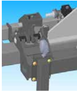
Lock Assembly “Engaged/Locked” Position Shown
