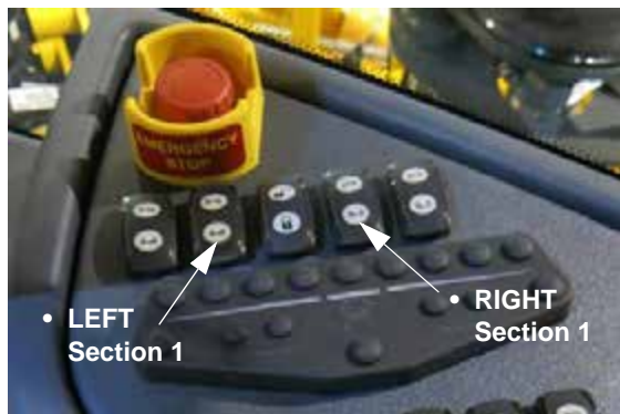
Section 1 Raise/Lower Switches (Located on the side console) -Typical View
