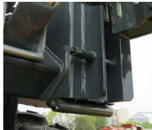
Lock Pin -Typical View * Engaged position shown
