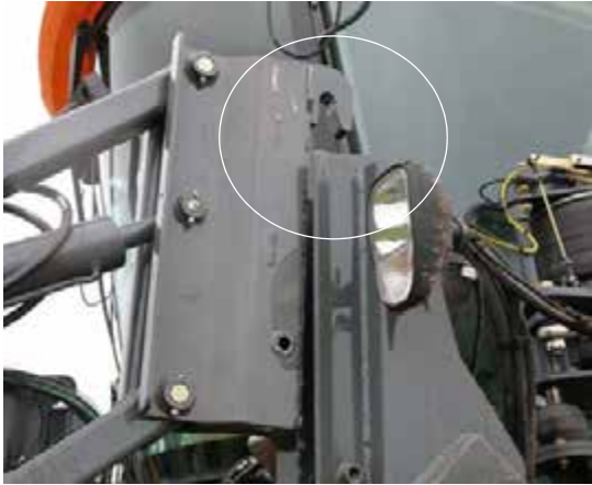
Attachment Clearing Mounting Pin -Typical View
