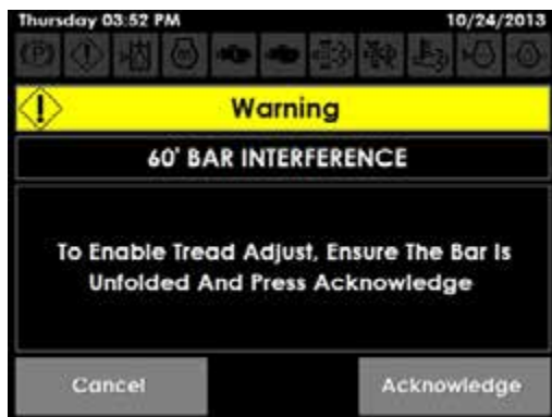
Tread Width Adjustment Warning Message
