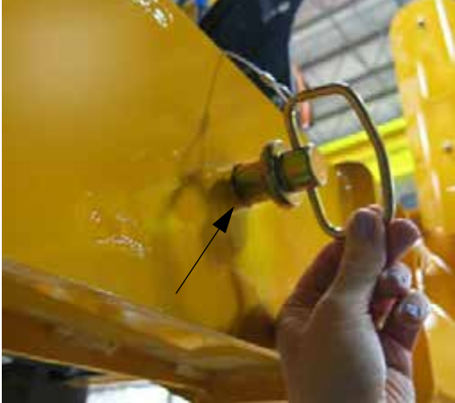
Securement Bolt -Typical View
