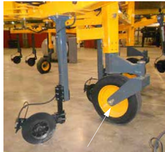
Gauge Wheel (One located on each side of NTB) -Typical View
