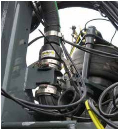
Solution Connection (Located on front right-hand side of machine) -Typical View
