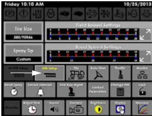
NTB Setup Button (Located on the Machine Display - Settings Page)
