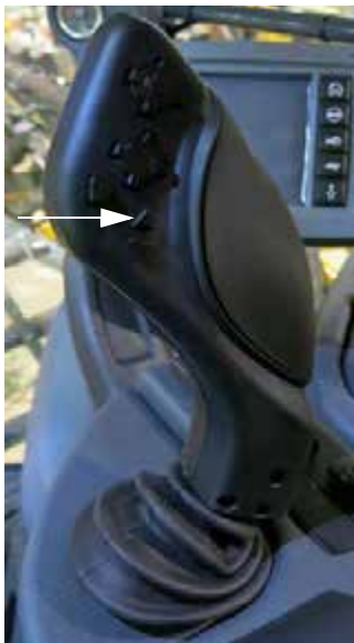
Transom Switch - UP (Located on the Hydrostatic Drive Control Handle) -Typical View
