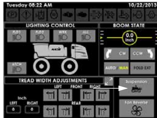
Suspension Button (Located on the Machine Display - Auxiliary Controls Page)
