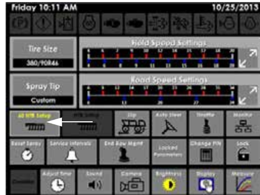
60' NTB Setup Button (Located on the Machine Display - Settings Page)
