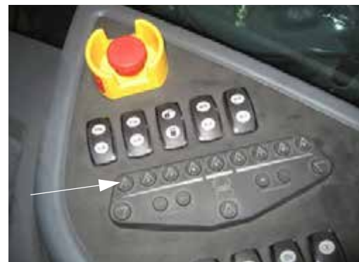
Boom Solution Valve Switches (Located on the side console) -Typical View
