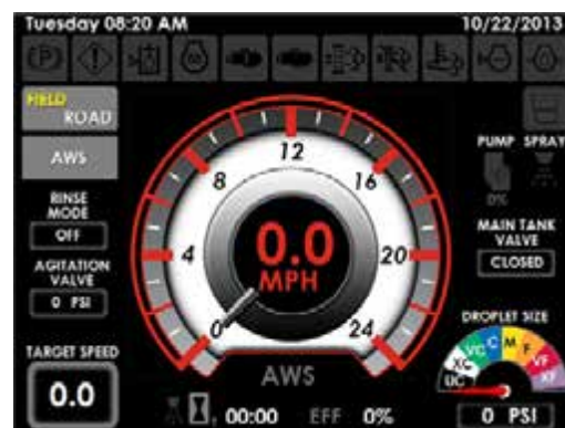
Machine Display - Home Page (Field Mode)
