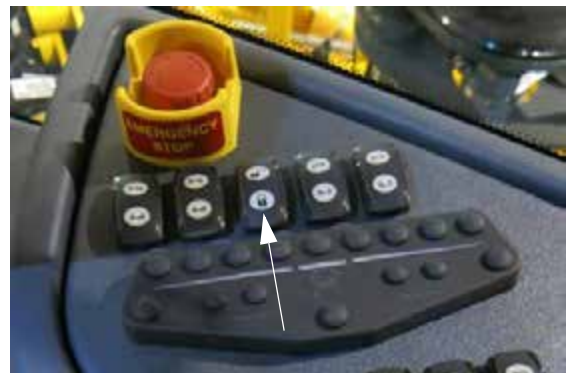
Lock Assembly Switch (Located on the side console) -Typical View
