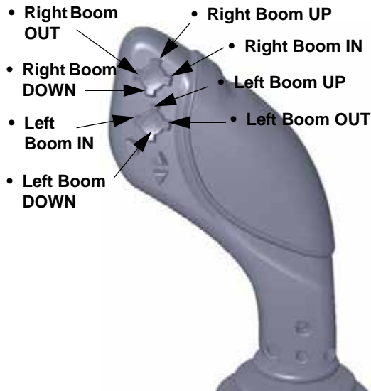
Left and Right Boom/ NTB Switch Orientation -Typical View
