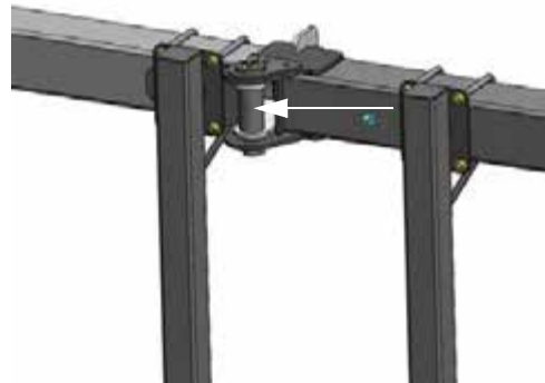
Grease Point C (Outer Fold) * 40-ft. NTB only
