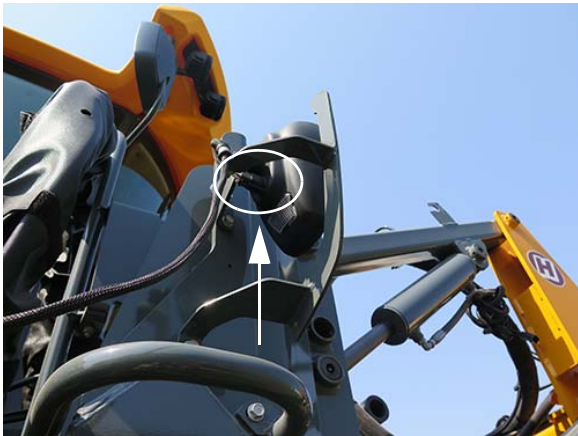
Headlight Wiring Harness Plug - Machine View (Located on the back side of headlight assembly) -Typical View
