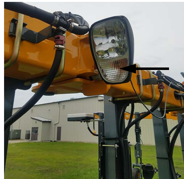
Hazard/Warning Light (2) (Mounted on each side of tool bar) -Typical View
