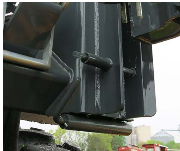
Lock Pin (2) -Typical View * Engaged position shown
