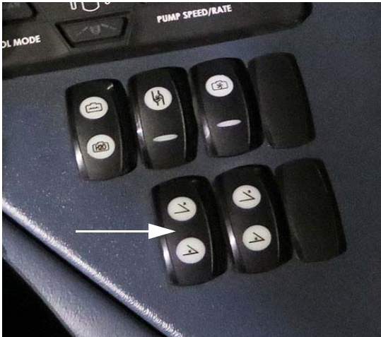
Boom/NTB Extension Switch (Located on the side console) -Typical View
