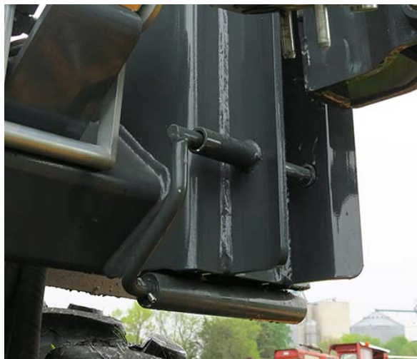
Lock Pin (2) -Typical View * Engaged position shown
