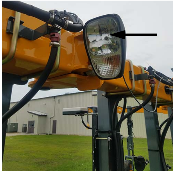
Highway Running Light (2) (Mounted on each side of tool bar) -Typical View
