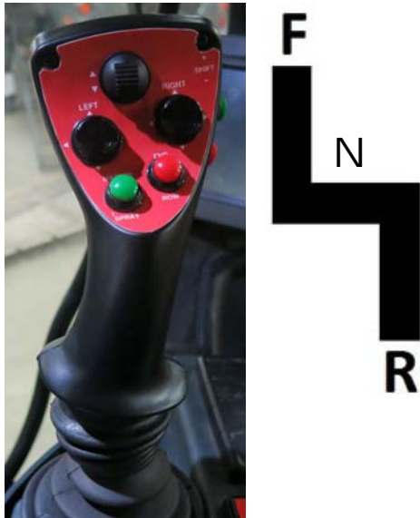
Hydrostatic Drive Control Handle -Typical View
