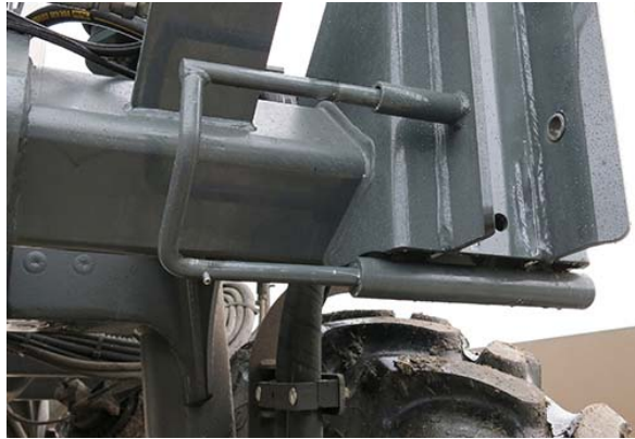
Lock Pin (2) (Located on the front left and right-hand side of machine) -Typical View * Disengaged position shown
