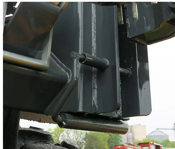
Lock Pin (2) -Typical View * Engaged position shown
