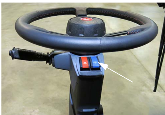
Highway Running Lights Switch (Located on the steering column) -Typical View
