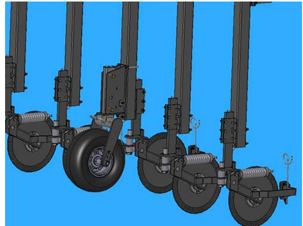
Gauge Wheel (Field position shown) -Typical View
