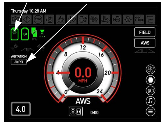
Main Tank and Agitation Valve Pressure Indicators (Located on the Machine Display Home Page - Field Mode)
