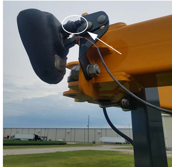
Headlight Mounting Bolt (Located on the back side of headlight assembly) -Typical View
