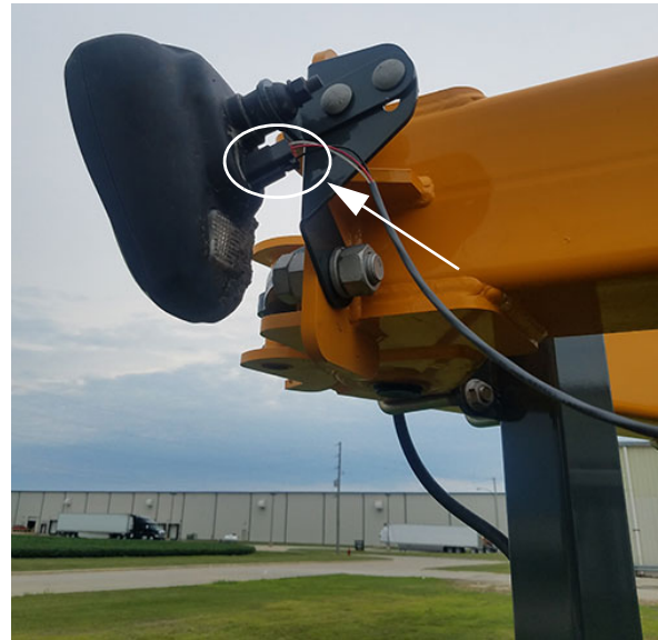
Headlight Wiring Harness Plug - Attachment View (Located on the back side of headlight assembly) -Typical View
