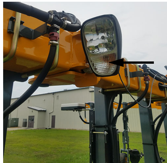
Hazard/Warning Light (2) (Mounted on each side of tool bar) -Typical View
