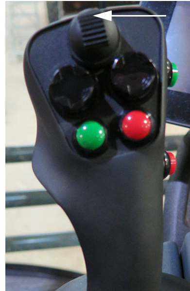
Transom Switch - UP (Located on the Hydrostatic Drive Control Handle) -Typical View
