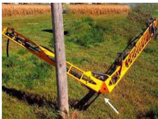
Outer Boom Breakaway -Typical View
