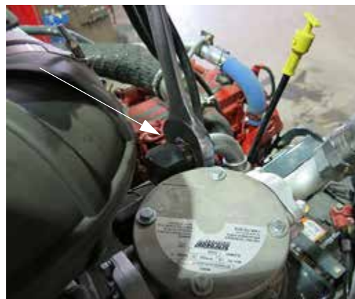
Case Drain Hose (Located near top of hydraulic reservoir) -Typical View
