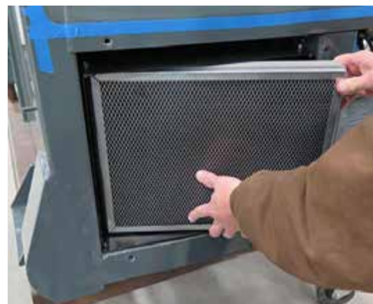
Charcoal Filter (Located behind the exterior service panel on the right-hand side of cab) -Typical View
