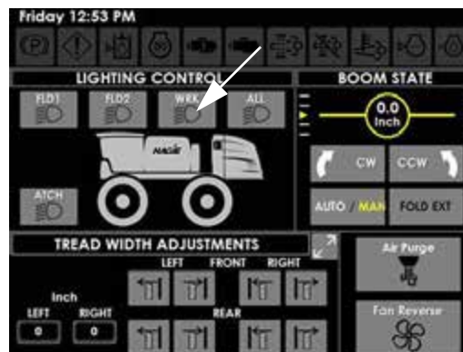
Work Lights Button (Located on the Auxiliary Controls Page)
