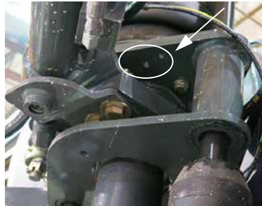
Collar Grease Zerk (Located beneath each air bag mounting plate) -Typical View
