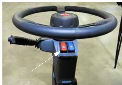
Hazard/Warning Lights Switch (Located on steering column)
