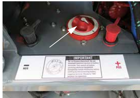
Battery Disconnect Switch (Located on the rear mainframe) -Typical View
