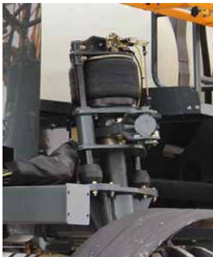
Air Bag (Located on each leg) -Typical View
