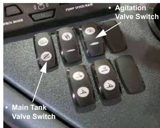
Main Tank and Agitation Valve Switches (Located on the side console) -Typical View
