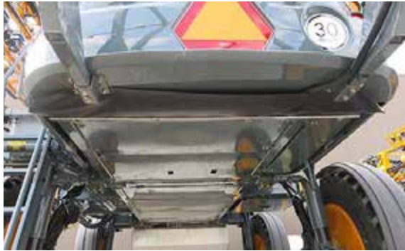
Belly Shield/Brush Curtain Installation -Typical View
