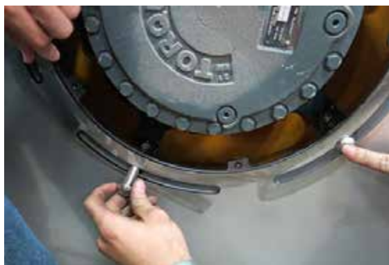
Wheel Cover Mounting Bolt Installation -Typical View
