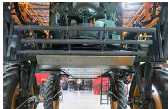
Brush Guard Installation -Typical View
