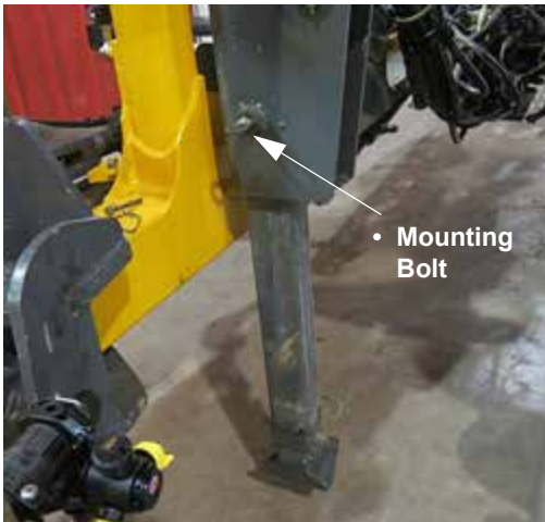
• Mounting Bolt Boom Stand (Extended position shown) -Typical View
