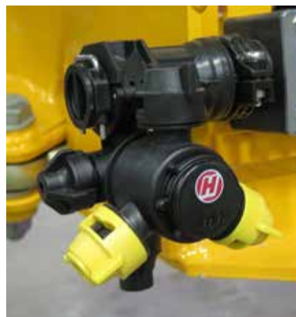
Nozzle Body (Located throughout boom) -Typical View
