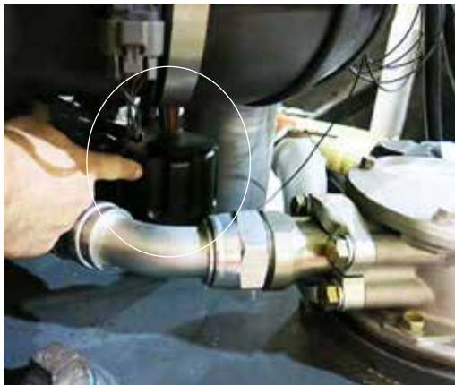
Breather Cap (Located on left-hand side of machine near return filter housing) -Typical View
