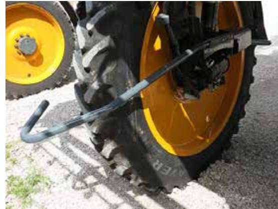
Installed Crop Divider -Typical View
