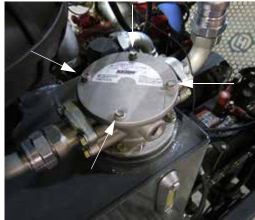
Return Filter Housing (Located on left-hand side of machine near hydraulic oil reservoir) -Typical View
