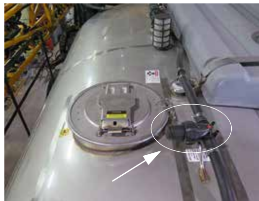
Tank Rinse Strainer (Located near top of main tank) -Typical View
