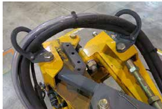
Boom Hose Clamp Installation -Typical View
