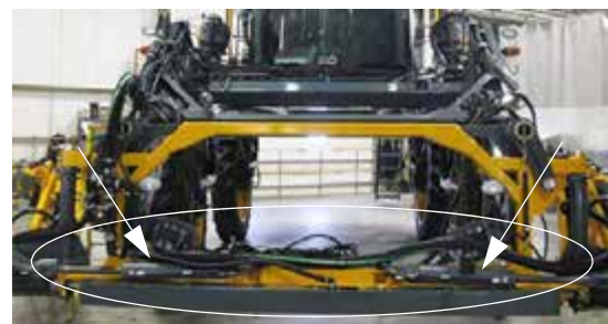
Main Pivot/Breakaway Cylinders -Typical View
