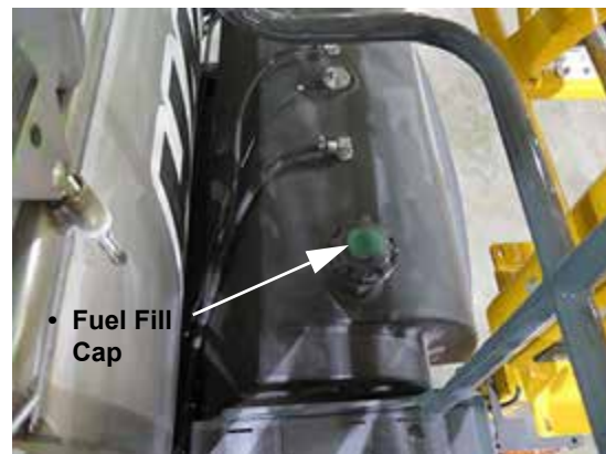
Engine Fuel Fill (Located behind the fuel tank on right-hand side of machine) -Typical View
