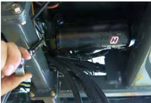
Charge Pump Filter (Located beneath drive pump) -Typical View
