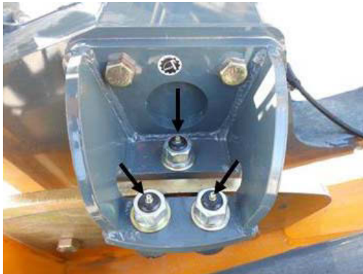
Roller Mount Assembly -Typical View
