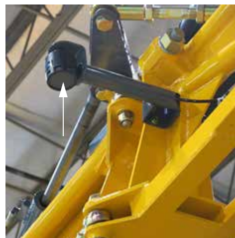
NORAC Sensor Foam Pad (Located on the bottom of each sensor) -Typical View
