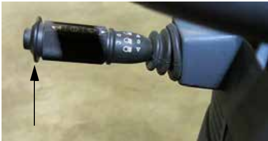
Windshield Washer Switch (Located on the end of the Turn Signal Lever) -Typical View
