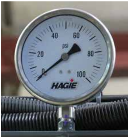
Pressure Gauge (Mounted on boom) -Typical View
