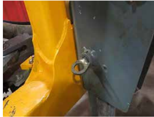
Lock Pin Removed -Typical View
