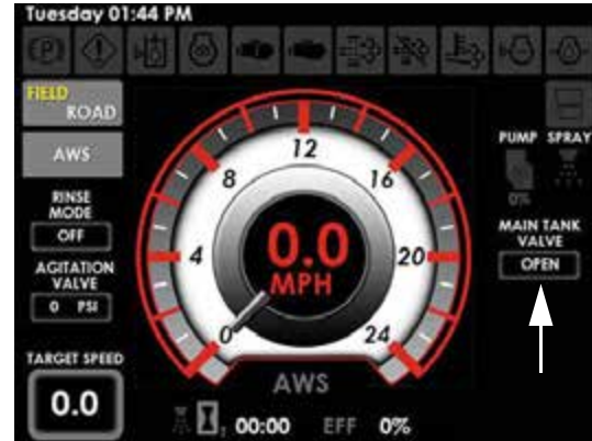
Main Tank Valve Status Indicator (Located on the Machine Home Page - Field Mode) -Typical View
