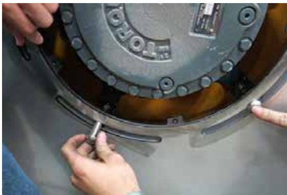
Wheel Cover Mounting Bolt Installation -Typical View
