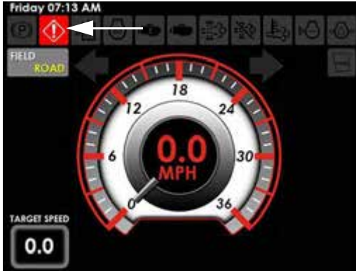
Warning Light Indicator (Located on the top left-hand side of each display page)
