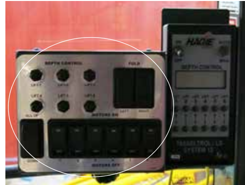
Detasseling Control Panel -Typical View
