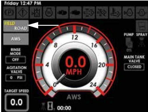
Field/Road Button (Located on the Machine Display Home Page - Road and Field Mode)
