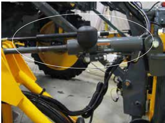
Level Cylinders -Typical View
