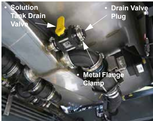
Solution Tank Drain Valve Assembly (Located beneath the solution tank on underside of machine) -Typical View
