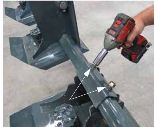
Cutter Head Bolts (Located on each Cutter Head Mounting Tube) -Typical View
