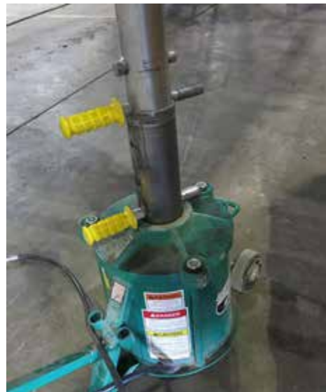
Lock Pin Installation -Typical View
