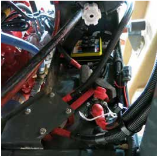
Tier 4 Final Engine Fuse/Relay Block (Located beneath batteries on the rear left-hand side of machine) -Typical View * View shown from beneath machine
