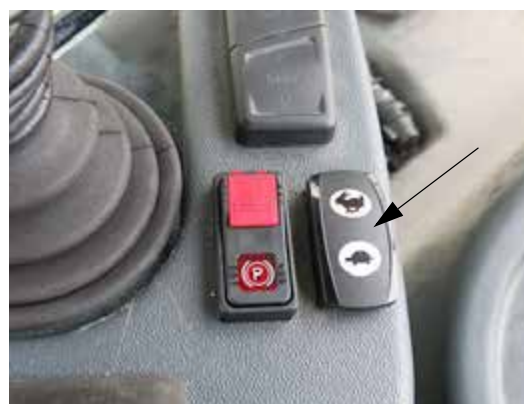
Throttle Switch (Located near the Hydrostatic Drive Control Handle) -Typical View
