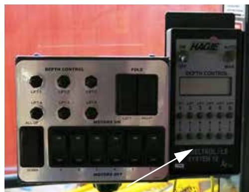
Tasselrol Control Panel -Typical View
