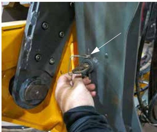
Lock Pin (Located on the outer side of transom frame) -Typical View
