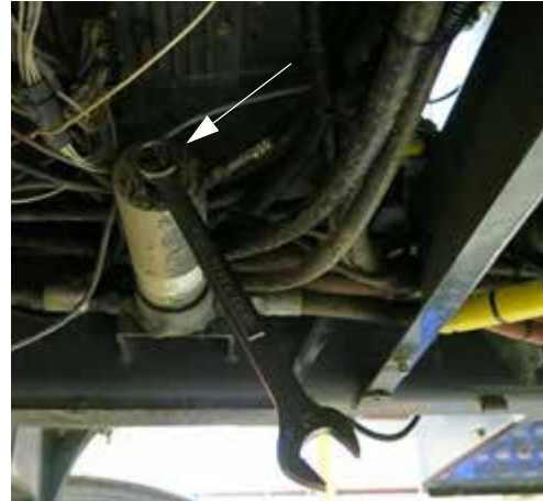
Pressure Filter Housing (Located beneath right-hand side of machine - lower metal shield to access) -Typical View
