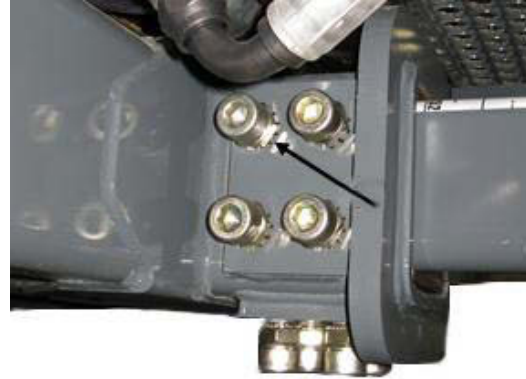
Jam Nut (Located on each tread adjust bearing bolt) -Typical View
