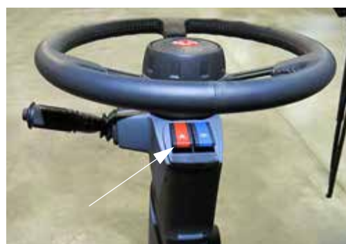
Hazard/Warning Lights Switch (Located on steering column)
