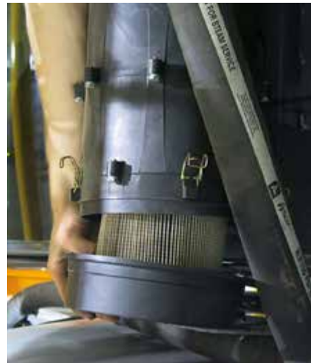
Filter Removal -Typical View
