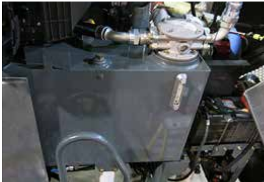
Hydraulic Oil Reservoir (Located on left-hand side of machine - open hood to access) -Typical View
