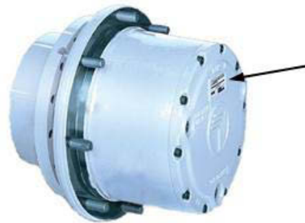
Wheel Hub Identification Plate -Typical View
