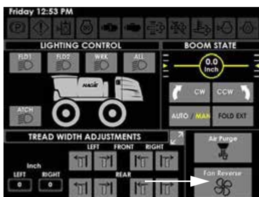
Reversible Fan Button (Located on the Auxiliary Controls Page)
