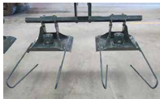
Stalk Guide Installation -Typical View
