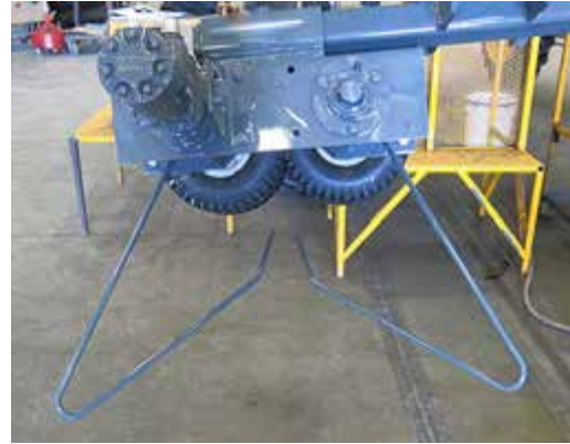
Stalk Guide Installation -Typical View
