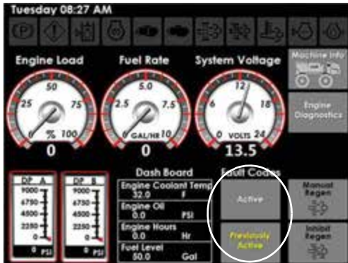
Fault Code Buttons (Located on the Machine Diagnostics Page)
