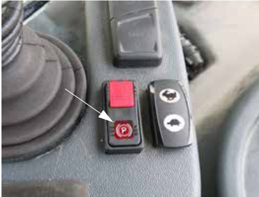
Parking Brake Switch (Located near the Hydrostatic Drive Control Handle) -Typical View
