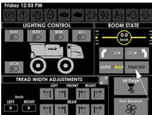
Fold Extension (Ext) Button (Located on the Machine Display Auxiliary Controls Page)
