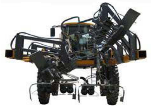
Staggered Detasseling Heads -Typical View
