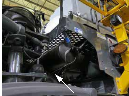
Tank Drain Valve (Air Purge) - if equipped (Located beneath platform near center right-hand side of machine)
