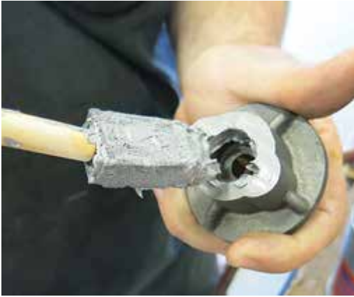
Anti-Seize Lubricant Application -Typical View
