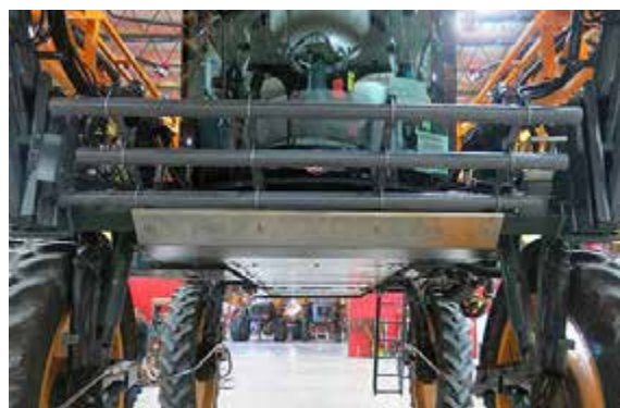
Brush Guard Installation -Typical View
