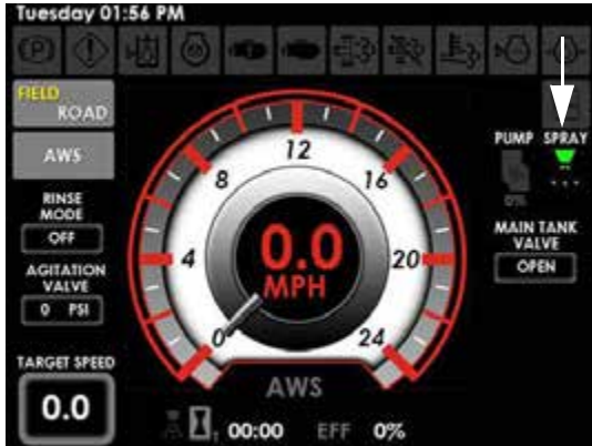
Master Spray Indicator (Located on the Machine Display Home Page - Field Mode) -Typical View
