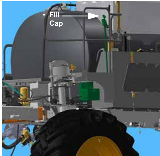
Foam Marker Reservoir Fill (Located on the rear right-hand handrail) -Typical View
