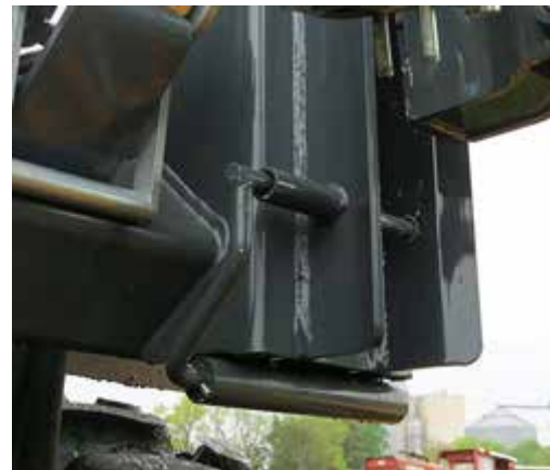
Lock Pin -Typical View * Engaged position shown
