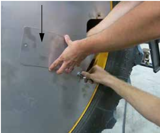
Valve Stem Access Panel -Typical View
