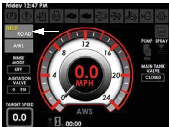
Field/Road Button (Located on the Machine Display Home Page) -Typical View
