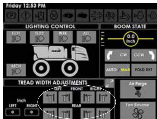
Tread Width Adjustment Buttons (Located on the Machine Display Auxiliary Controls Page)
