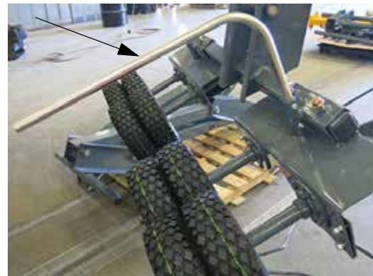
Deflector Shield Mounting Tube -Typical View
