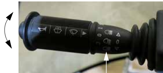
High Beams (Located on the Turn Signal Lever) -Typical View
