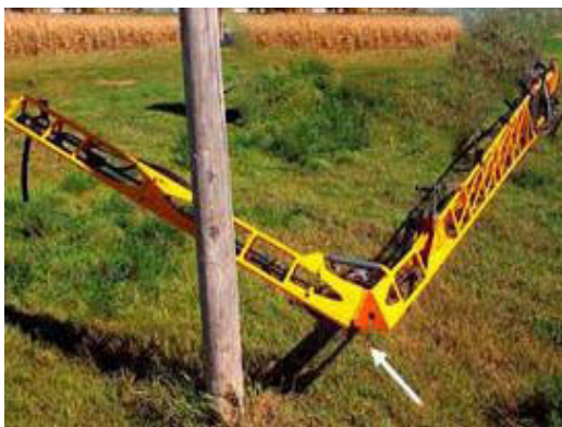
Outer Boom Breakaway -Typical View
