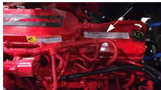
Engine Identification Plate -Typical View
