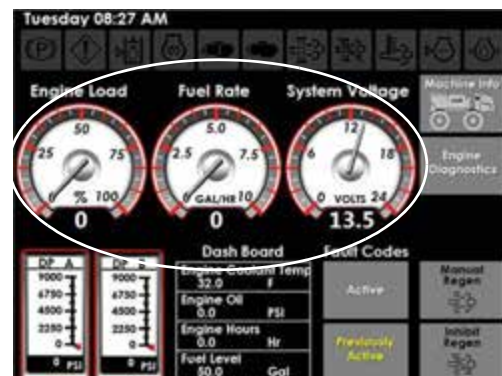
System Gauges (Located on the Machine Diagnostics Page)
