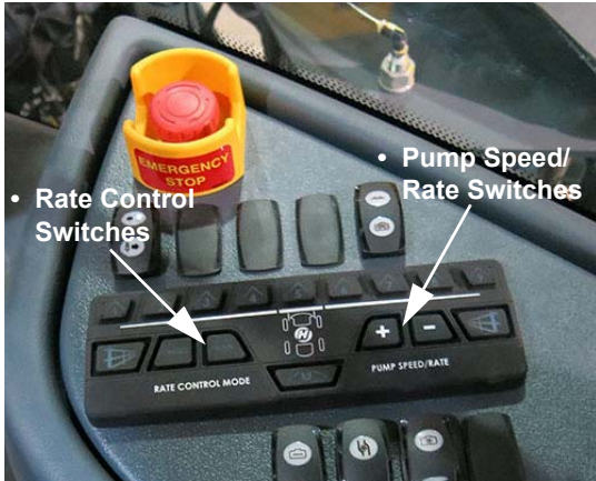
Rate Control and Pump Speed/Rate Switches (Located on the side console) -Typical View
