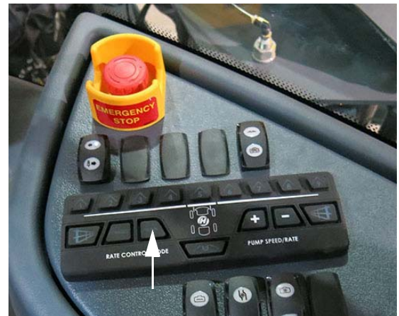
Manual "MAN" Rate Control Switch (Located on the side console) -Typical View
