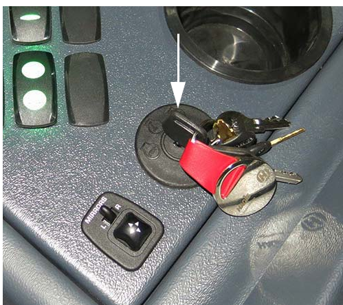
Ignition Switch (Located on the side console) -Typical View
