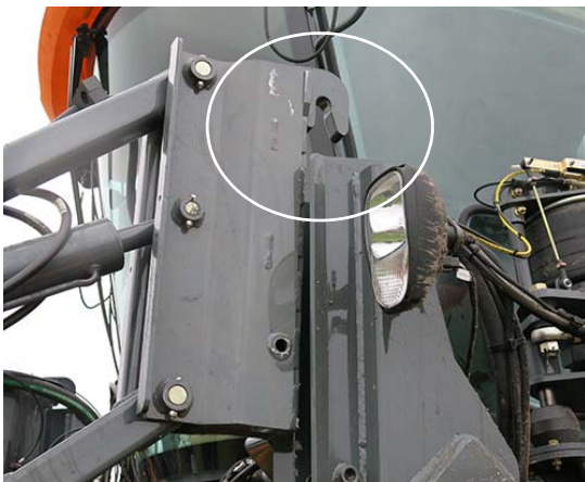
Attachment Clearing Mounting Pin -Typical View
