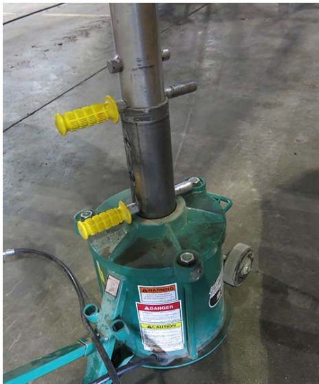
Lock Pin Installation -Typical View
