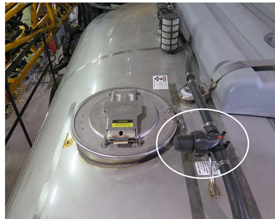
Tank Rinse Strainer (Located on top of solution tank) -Typical View
