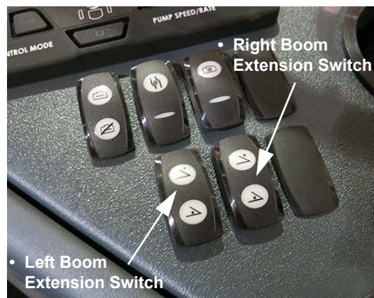
Left and Right Boom Extension Switches (Located on the side console) -Typical View
