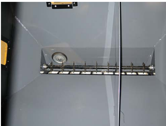
Clean-out Port Locations -Typical View
