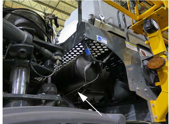
Tank Drain Valve (Air Purge) - if equipped (Located beneath platform near center right-hand side of machine) * Pull DOWN to open -Typical View
