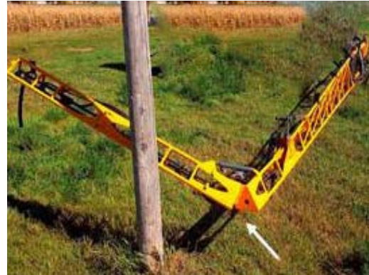
Outer Boom Breakaway -Typical View
