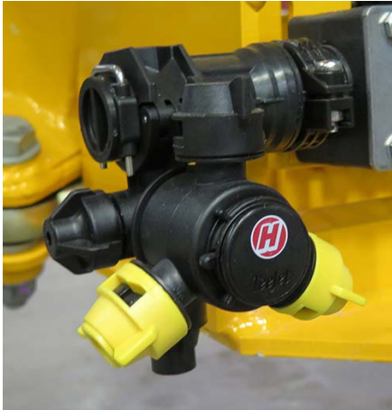
Nozzle Body (Located throughout boom) -Typical View
