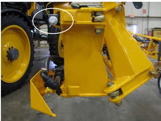
Proximity Sensors -Typical View
