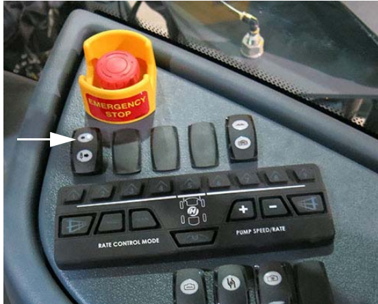
Foam Marker Switch (Located on the side console) -Typical View
