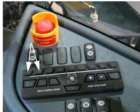
Boom Solution Valve Switches 1 and 2 (Located on the side console) -Typical View
