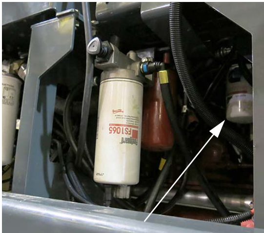
Engine Oil Filter (Located along left-hand side of machine - open hood to access) -Typical View
