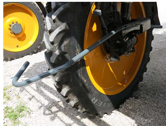
Installed Crop Divider -Typical View
