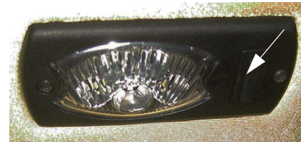
Interior Work Light Switch -Typical View
