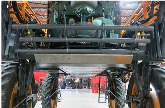
Brush Guard Installation -Typical View
