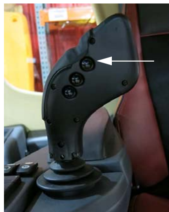
Master Spray Switch (Located on the back side of the Hydrostatic Drive Control Handle) -Typical View
