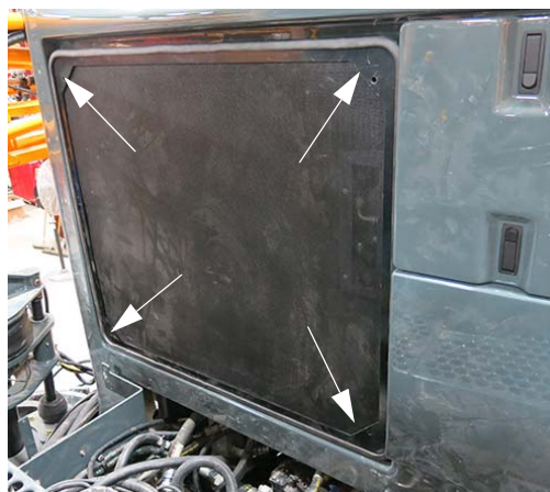
Radiator Screen Latches (Located on each corner of the screen) -Typical View
