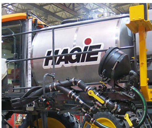
Solution Tank -Typical View
