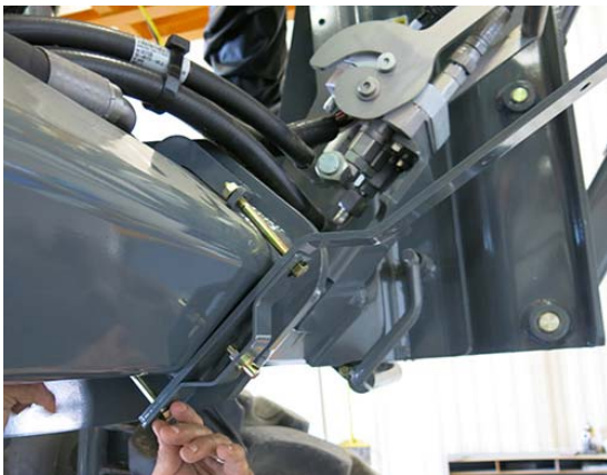
Anchor Bolt Assembly -Typical View
