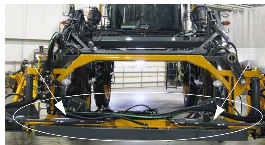
Main Pivot/Breakaway Cylinders -Typical View
