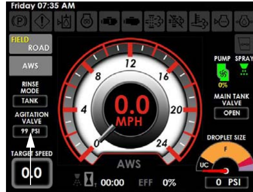
Agitation Valve Pressure Indicator (Located on the Machine Display Home Page - Road and Field Mode)
