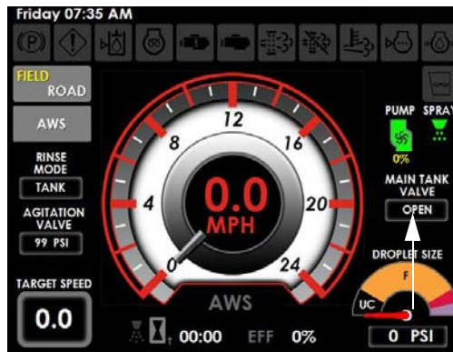
Main Tank Valve Status Indicator (Located on the Machine Display Home Page - Field Mode)
