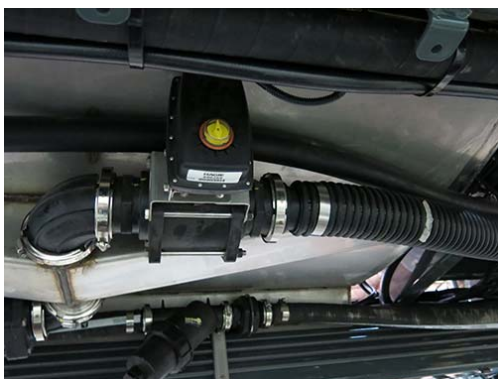
Solution Tank Valve -Typical View
