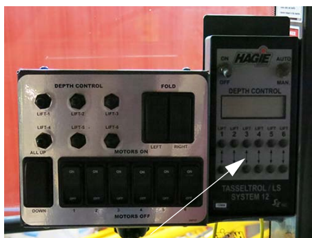
Tasselrol/LS System 12 Control Panel -Typical View
