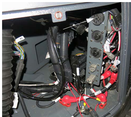
Engine Diagnostic Port (Located inside the side console - remove front panel to access) -Typical View
