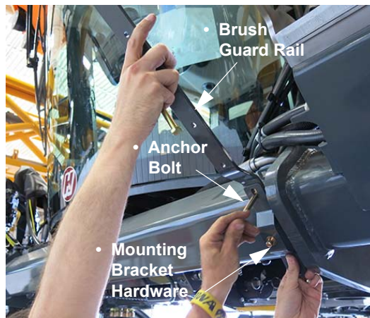
Brush Guard Rail Assembly -Typical View
