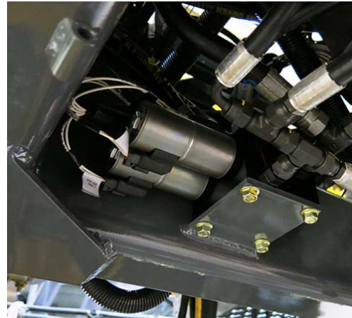
Valve Manifold (Located on the underside of machine) -Typical View
