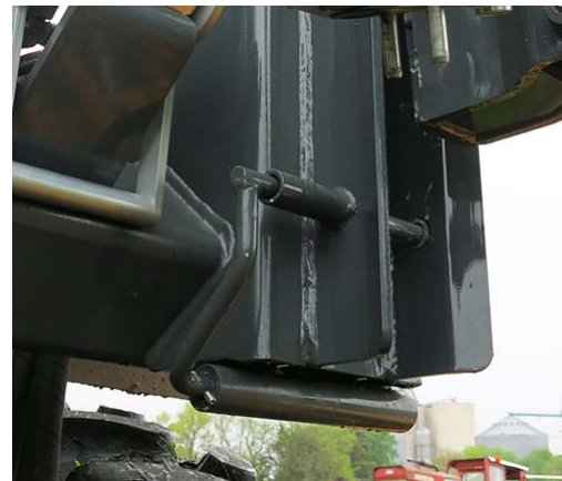
Lock Pin -Typical View * Engaged position shown
