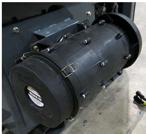
Cab Filtration System (Located on the right-hand side of the exterior cab) -Typical View
