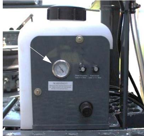
Foam Pressure Gauge (Located on the side of the Foam Marker Tank, mounted on the right-hand side of machine) -Typical View
