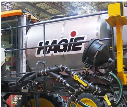
Solution Tank -Typical View
