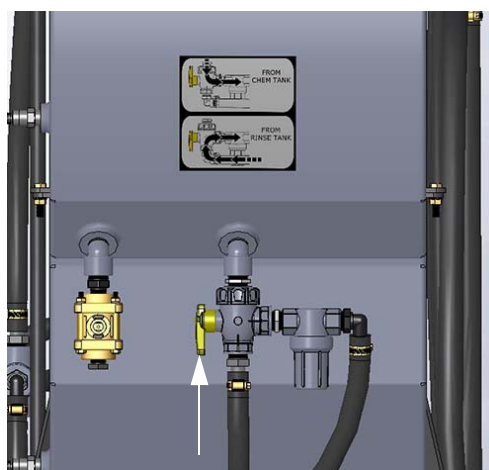
Inlet Selector Valve - 60 Gallon Tanks (Located on the outer side of Tanks 1 and 3) -Typical View
