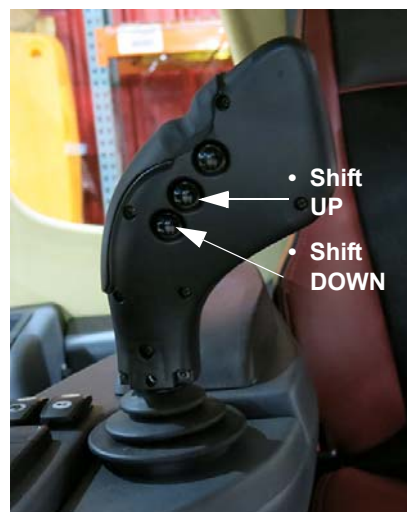
Shift Up/Down Switches (Located on the back side of the Hydrostatic Drive Control Handle) -Typical View
