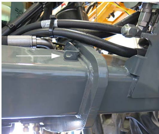
Brush Guard Mounting Bracket (Left-hand side of machine shown) -Typical View
