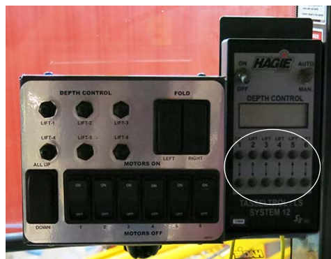
Lift Up/Down Switches (Located on the Tasseltrol Control Panel) -Typical View
