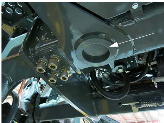
Lifting Point Containment Rings (Located on the frame near each leg) -Typical View
