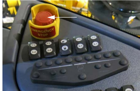
E-Stop Switch (Located on the side console) -Typical View
