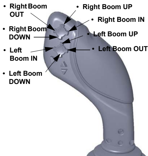
Left and Right Boom Switch Orientation -Typical View
