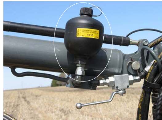
Accumulator -Typical View
