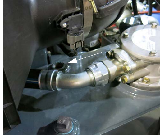
Breather Cap Removed -Typical View
