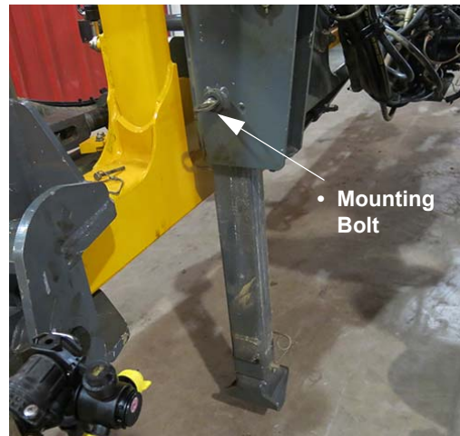
Boom Stand (Extended position shown) -Typical View
