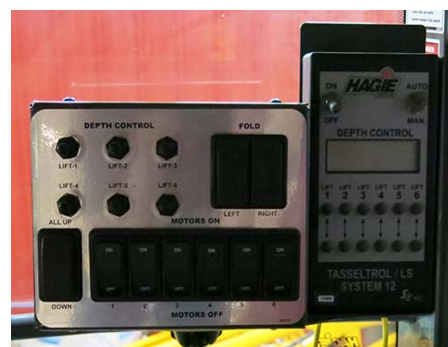
Detasseling and Tasselrol/ LS System 12 Control Panels -Typical View
