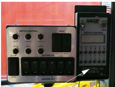
Tasselrol Control Panel -Typical View
