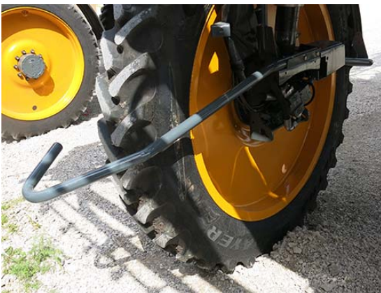
Installed Crop Divider -Typical View
