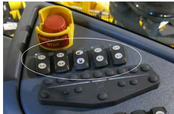
60' NTB Switches (Located on the side console) -Typical View
