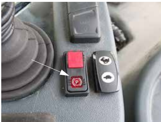
Parking Brake Switch (Located near the Hydrostatic Drive Control Handle) -Typical View
