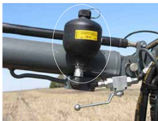
Accumulator -Typical View
