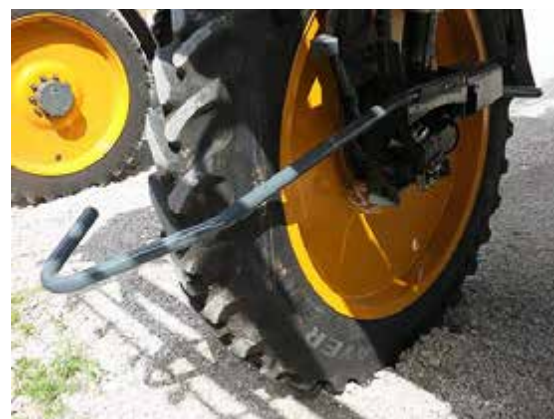
Installed Crop Divider -Typical View
