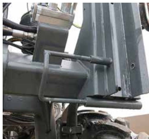
Lock Pin (Located on the front left and right-hand side of machine) -Typical View * Disengaged position shown
