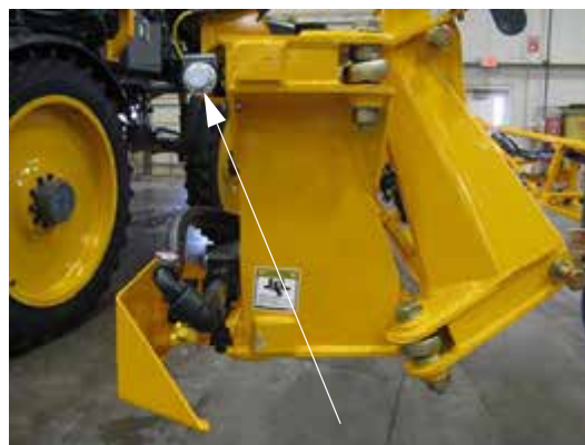
Proximity Sensors -Typical View
