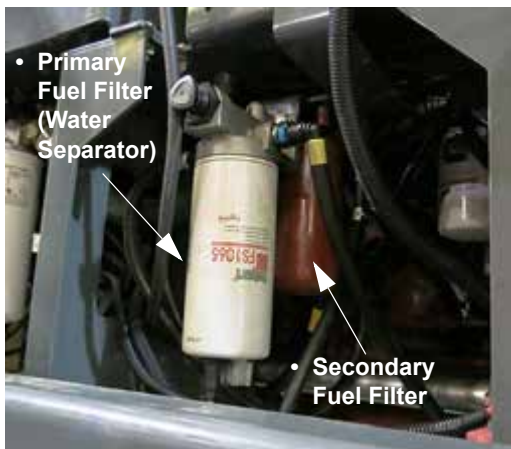
Primary and Secondary Fuel Filters (Located along left-hand side of machine - open hood to access) -Typical View
