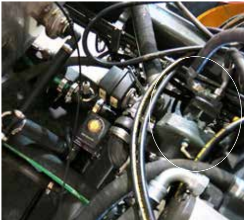
Solution Pump (Located near center of machine) -Typical View * View shown from top of machine
