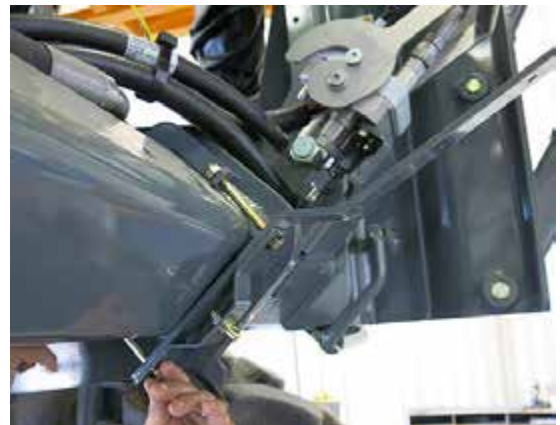
Anchor Bolt Assembly -Typical View
