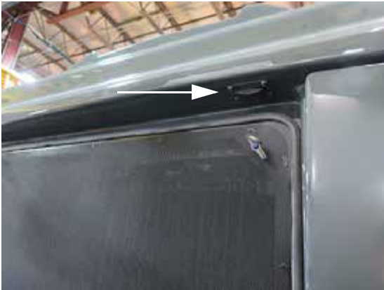
Hood Switch (Located ahead of rear hood above the radiator screen) -Typical View
