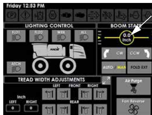
Boom Alignment Value (Located on the Auxiliary Controls Page)
