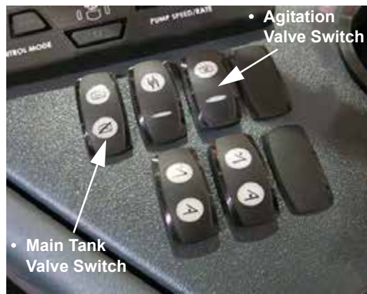
Main Tank and Agitation Valve Switches (Located on the side console) -Typical View
