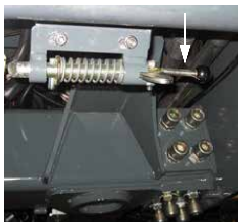
Front Fill Release Lever (Located beneath front end of machine) -Typical View
