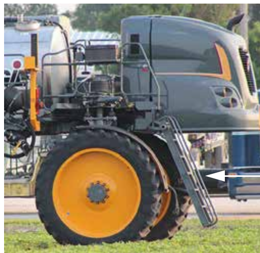
Ladder -Typical View * Lowered position shown
