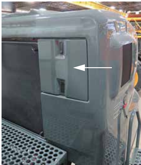
Engine Air Intake Filter Access Panel (Located on left-hand side of hood) -Typical View
