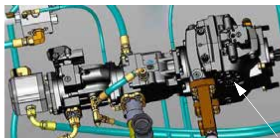
Hydrostatic Pump (Drive Pump) -Typical View (Viewed from top of machine)
