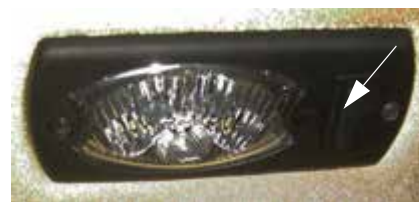
Interior Work Light Switch -Typical View
