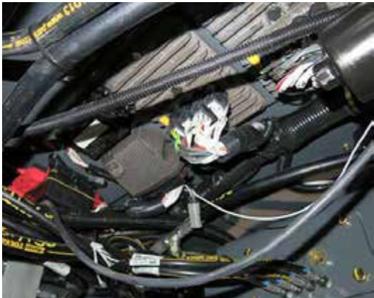
Circuit Breakers/Fuses (Exterior) (Located beneath cab - remove panel to access) -Typical View
