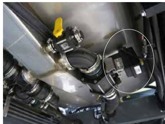
Solution Tank Valve (Located beneath the solution tank on underside of machine) -Typical View
