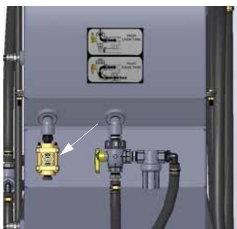
Tank Drain Valve -Typical View
