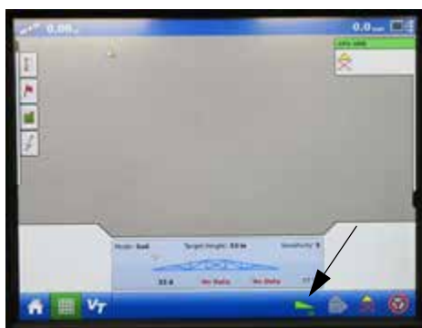
Auto/Manual Button - Ag Leader (Located on the main “Run Screen”) -Typical View * Your monitor may vary in appearance, depending on model
