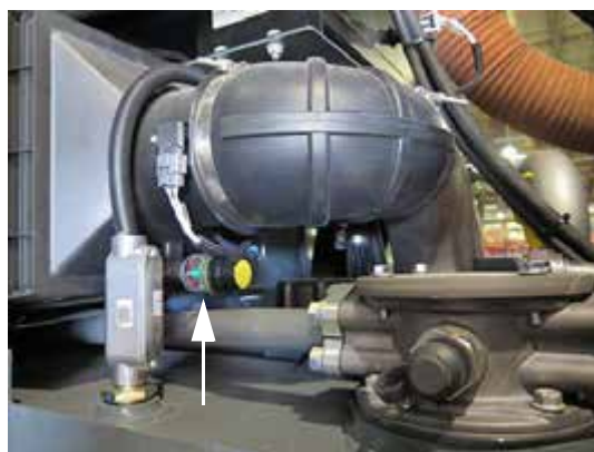
Filter Minder (Located near engine pre-filter - open hood to access) -Typical View
