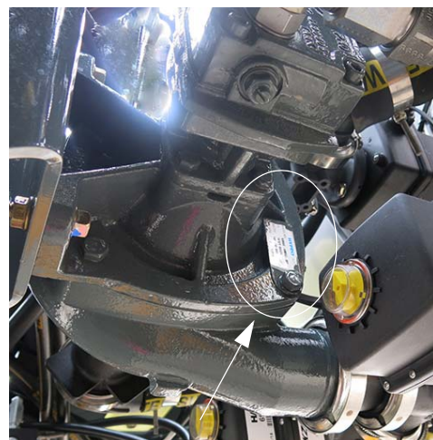
Solution Pump Identification Plate * View shown from beneath machine -Typical View
