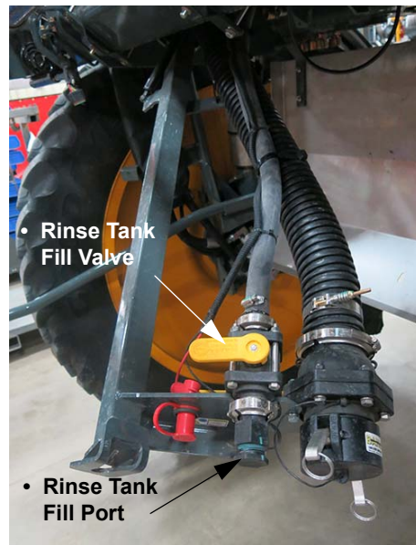
Front Fill Assembly (Lowered position shown) -Typical View
