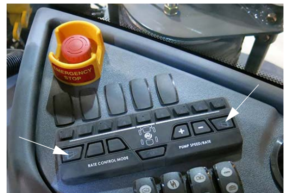
Fence Row Switches (Located on the side console) -Typical View
