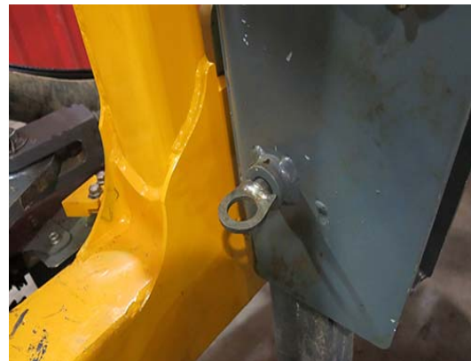
Lock Pin Removed -Typical View
