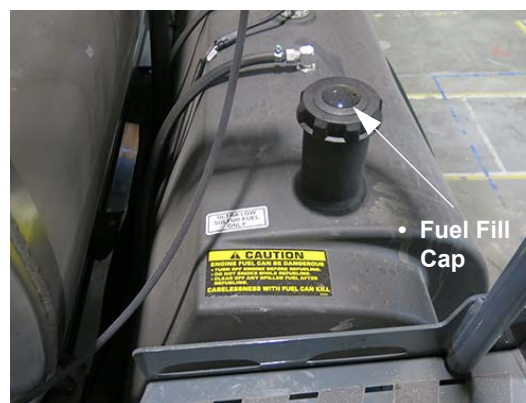
Engine Fuel Fill (Located behind the fuel tank on right-hand side of machine) -Typical View
