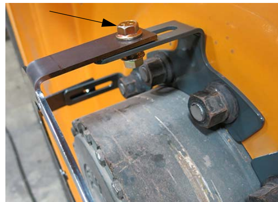
Hub Cap Adapter Bolt Installation -Typical View
