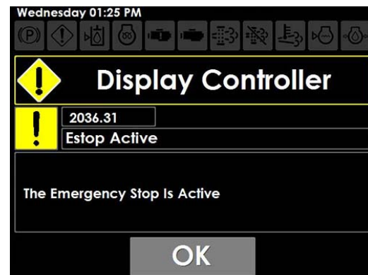
E-Stop Active Message (Located on the Machine Display)
