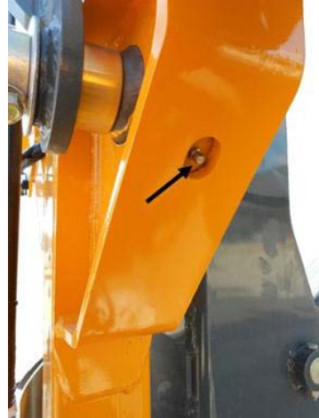
Pivot Transom Ball Joints -Typical View
