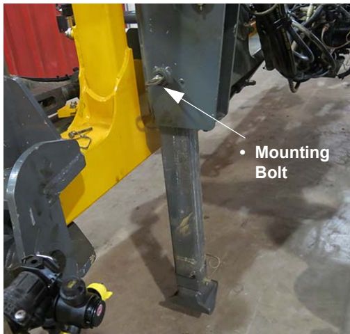
Boom Stand (Extended position shown) -Typical View
