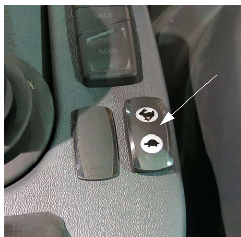
Throttle Switch (Located near the Hydrostatic Drive Control Handle) -Typical View
