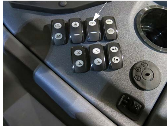
Agitation Valve Switch (Located on the side console) -Typical View
