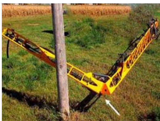
Outer Boom Breakaway -Typical View
