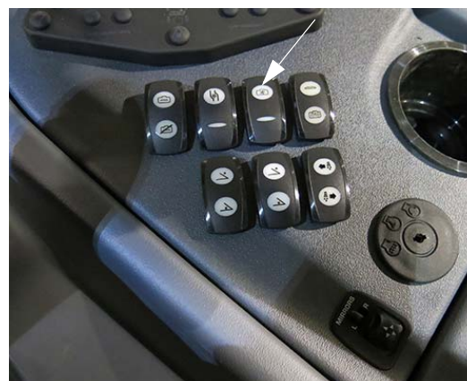
Agitation Valve Switch (Located on the side console) -Typical View
