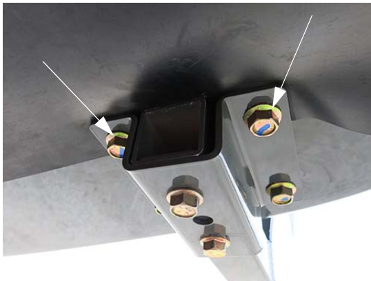
Mounting Bolts (Two located on each side of hood bracket) -Typical View * Your machine may vary in appearance, depending on available equipment.
