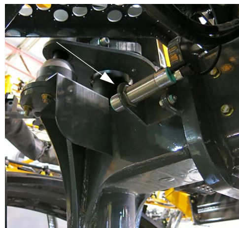
Tread Adjust Electronic Sensor (Rear Legs) -Typical View
