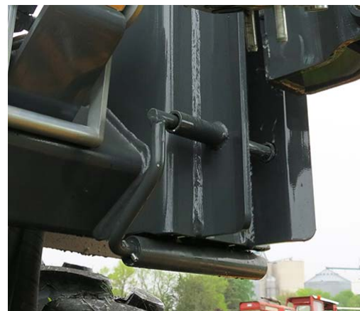
Lock Pin -Typical View * Engaged position shown
