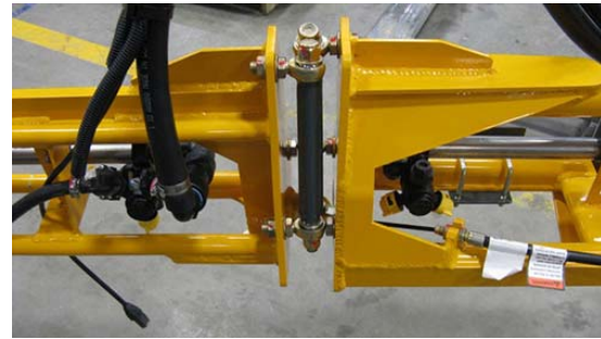
Outer Breakaway -Typical View
