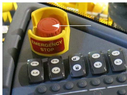
E-Stop Switch (Located on the side console) -Typical View
