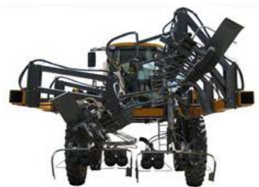
Staggered Detasseling Heads -Typical View
