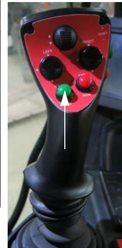
Main Control Switch (Located on the Hydrostatic Drive Control Handle) -Typical View
