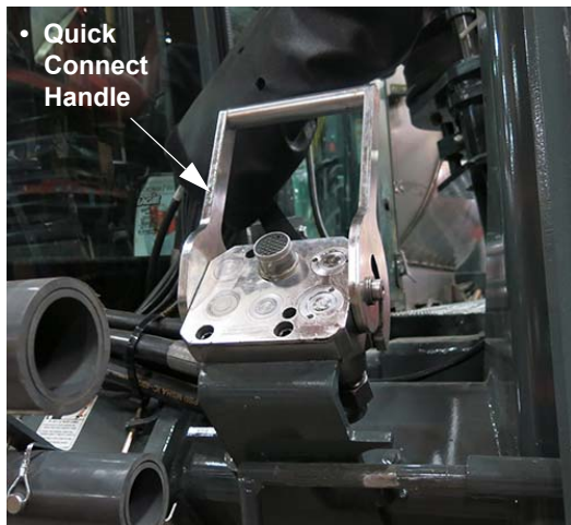
Hydraulic/Electric Multi-Coupler Assembly - If Equipped (Located on the front left-hand side of machine)
