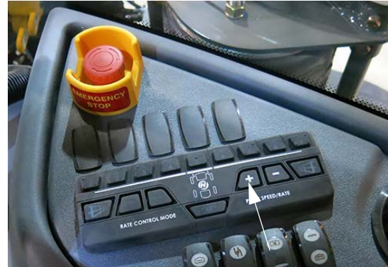
“+” Pump Speed/Rate Switch (Located on the side console) -Typical View
