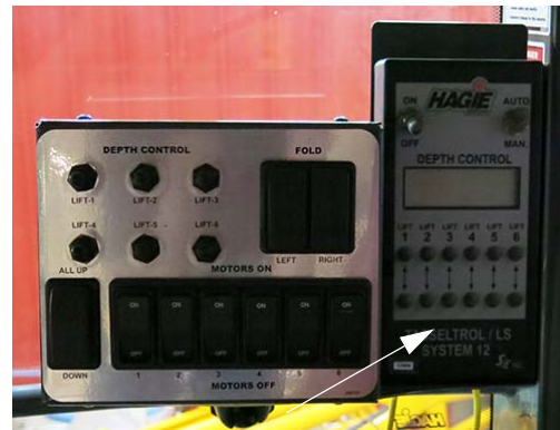
Tasselrol Control Panel -Typical View
