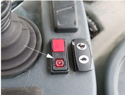
Parking Brake Switch - if equipped (Located near the Hydrostatic Drive Control Handle) -Typical View
