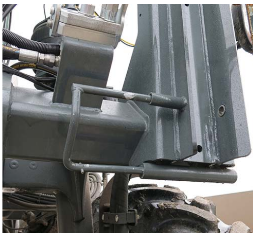
Lock Pin (Located on the front left and right-hand side of machine) -Typical View
