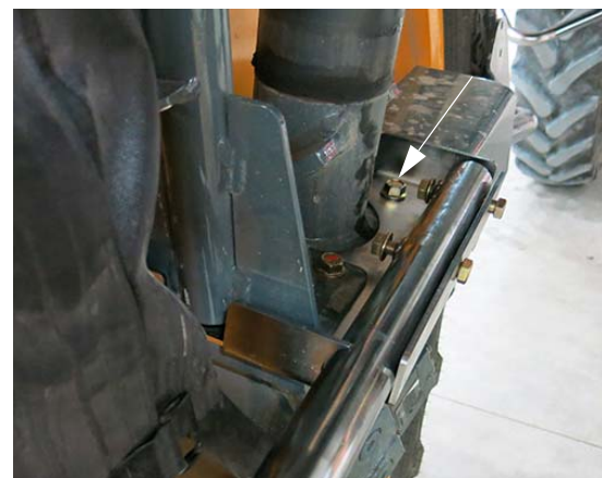
Mounting Plate Bolt -Typical View
