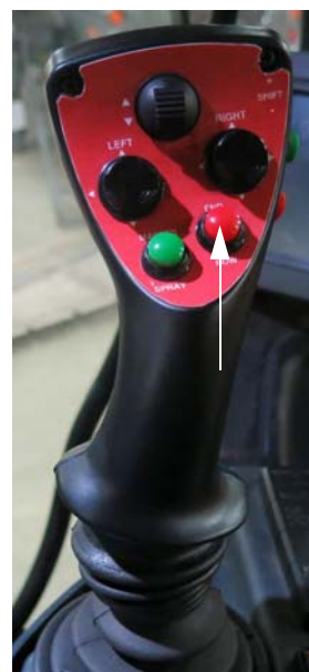
End Row Management Switch (Located on the Hydrostatic Drive Control Handle - Version 2) -Typical View
