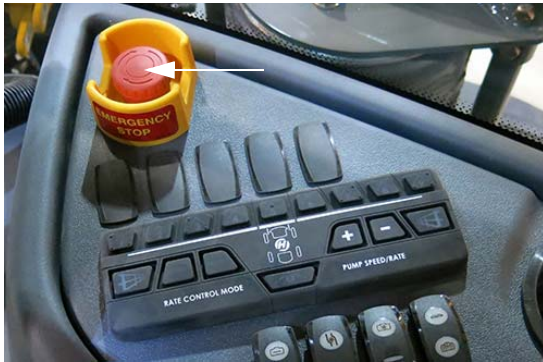
E-Stop Switch (Located on the side console) -Typical View
