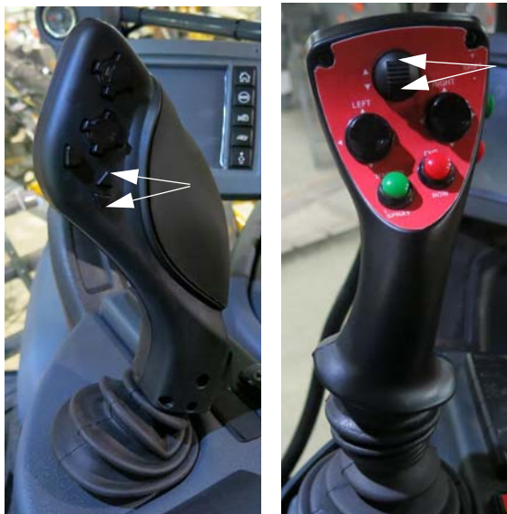
All-Up/Down Switches (Located on the Hydrostatic Drive Control Handle) -Typical View
