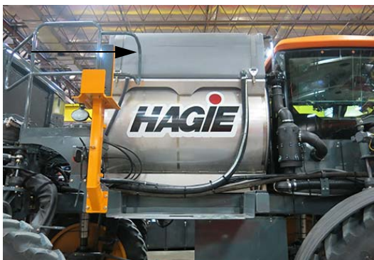
Rinse Tank -Typical View
