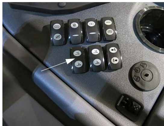
Boom Extension Switch * 90-ft. Spray Booms (Located on the side console) -Typical View
