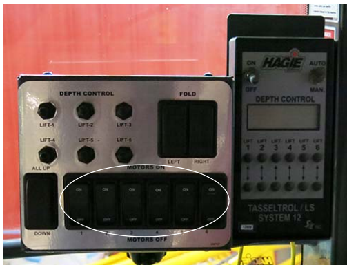
Motor Control Switches (Located on the Detasseling Control Panel) -Typical View
