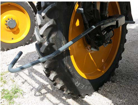
Installed Crop Divider -Typical View
