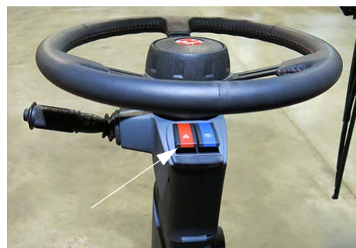
Hazard/Warning Lights Switch (Located on steering column)
