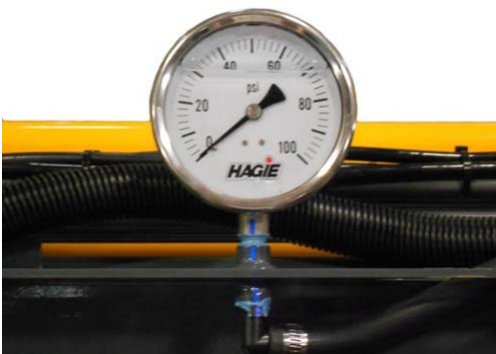
Pressure Gauge (Mounted on boom) -Typical View
