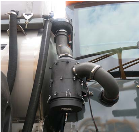
Cab Filtration System (Located on the right-hand side of the exterior cab) -Typical View
