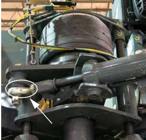
Tie Rod Ball Grease Zerk (Located on the front legs) -Typical View
