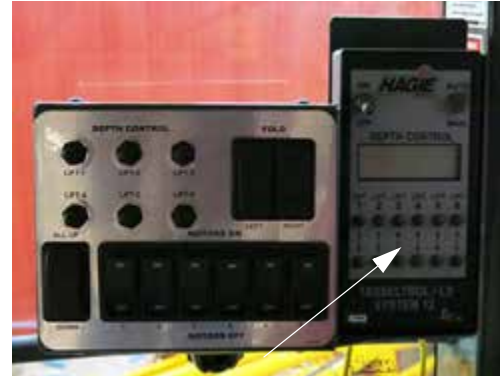
Tasselrol/LS System 12 Control Panel -Typical View
