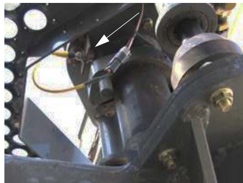
External Proximity Sensor -Typical View
