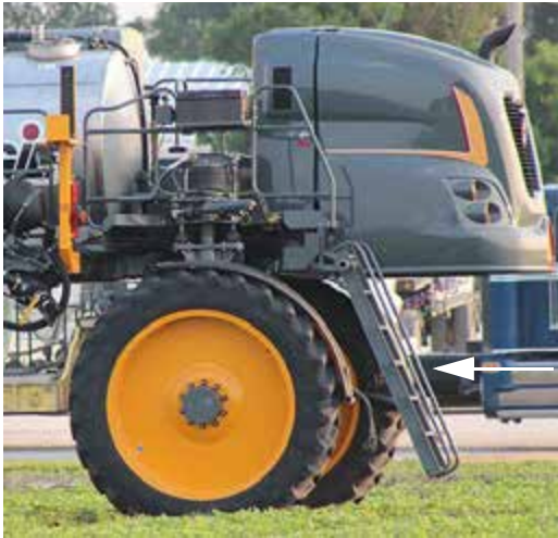
Ladder -Typical View * Lowered position shown
