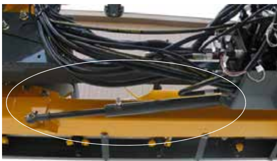
Roll Cylinder -Typical View
