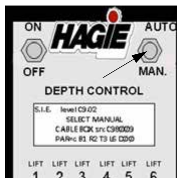
Auto/Manual Switch (Located on the Tasselrol Control Panel)
