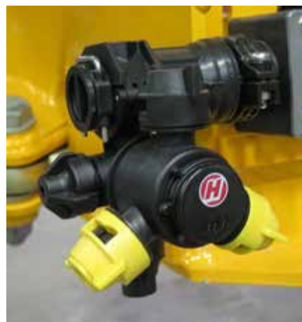
Nozzle Body (Located throughout boom) -Typical View
