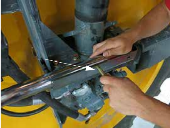
Crop Divider Mounting Bolt -Typical View
