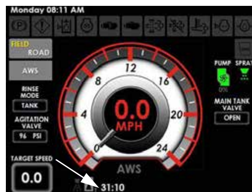
Spray Application Time Indicator (Located on the Home Page - Field Mode)
