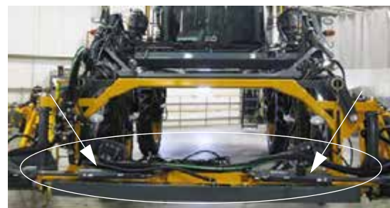
Main Pivot/Breakaway Cylinders -Typical View
