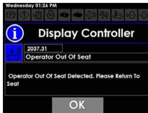
Operator Out Of Seat Message (Located on the Machine Display)
