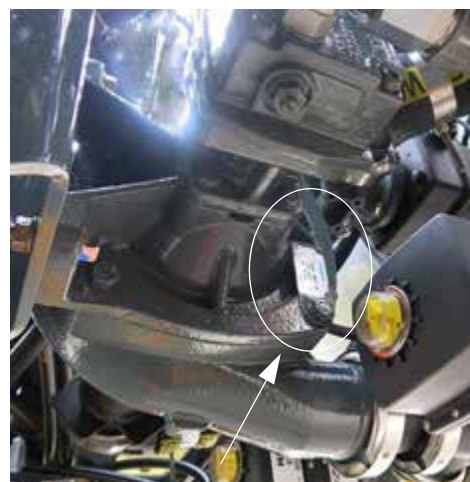
Solution Pump Identification Plate * View shown from beneath machine -Typical View
