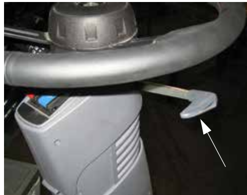
Steering Wheel Telescope Adjust Handle (Located to the right of the steering column) -Typical View
