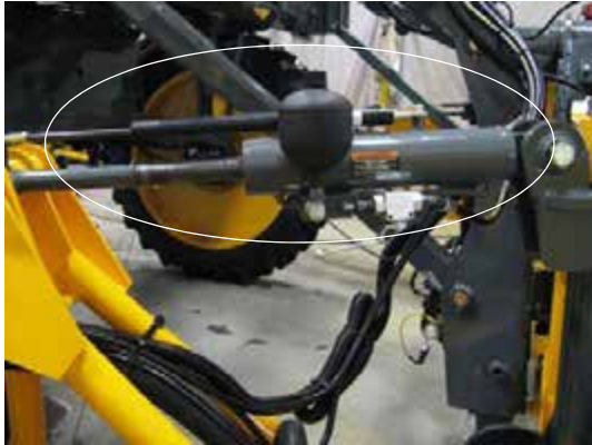
Level Cylinders -Typical View
