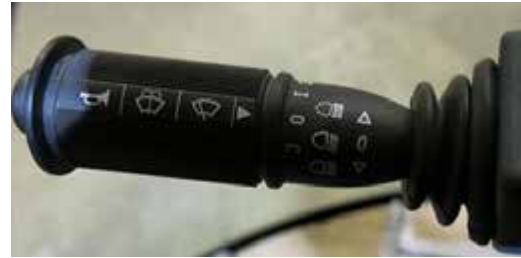
Turn Signal Lever -Typical View
