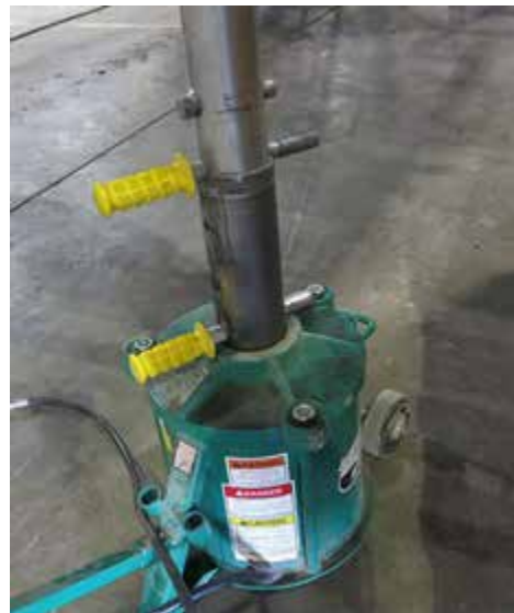
Lock Pin Installation -Typical View
