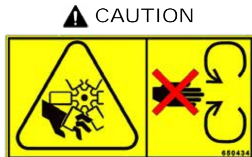
CUTTING/SEVERING OF FINGERS OR HAND. DO NOT PLACE FINGERS OR HAND NEAR MOVING FAN BLADES.
