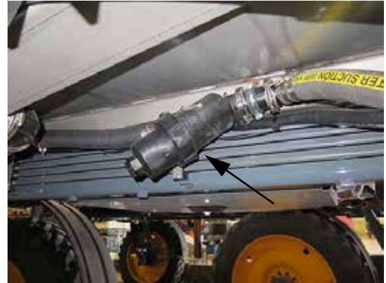
Solution Line Strainer (Located beneath the center right-hand side of machine) -Typical View
