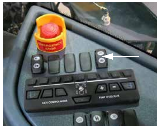
Rinse Switch (Located on the side console) -Typical View
