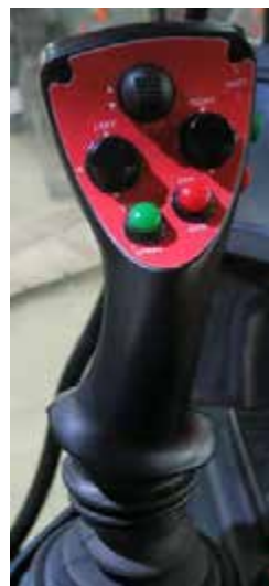
Hydrostatic Drive Control Handle -Typical View
