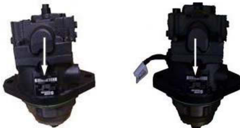
Front Rear Wheel Motor Identification Plates -Typical View
