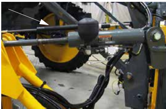
Position Sensor -Typical View
