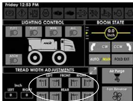
Tread Width Adjustment Buttons (Located on the Auxiliary Controls Page)
