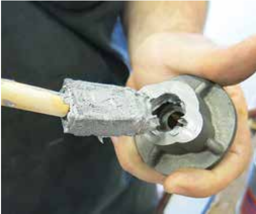
Anti-Seize Lubricant Application -Typical View
