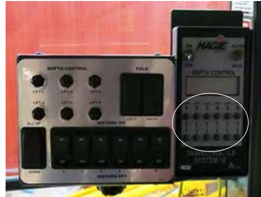
Lift Up/Down Switches (Located on the Tasselrol Control Panel) -Typical View
