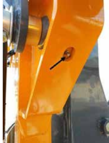
Pivot Transom Ball Joints -Typical View
