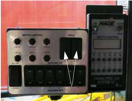
Left/Right Fold Switches (Located on the Detasseling Control Panel) -Typical View
