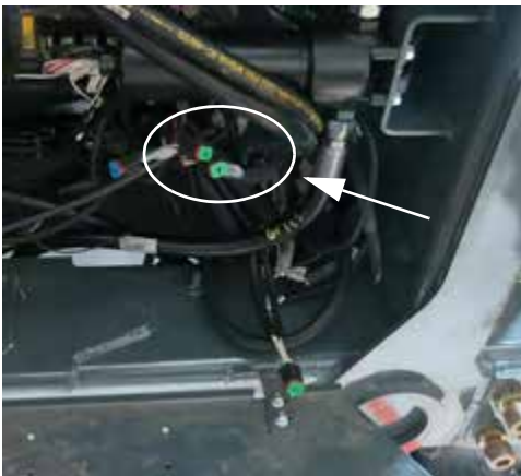
Video Camera Input Connections (Located beneath cab - remove front panel to access) -Typical View
