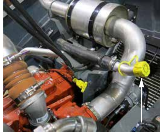
Engine Oil Fill (Located on rear left-hand side of machine - open hood to access) -Typical View
