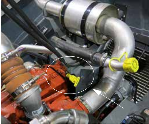
Engine Oil Dipstick (Located on rear left-hand side of machine - open hood to access) -Typical View
