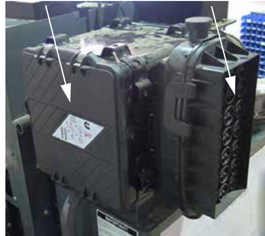
Engine Air Intake Filter and Pre-Cleaner (Located on rear left-hand side of machine) -Typical View
