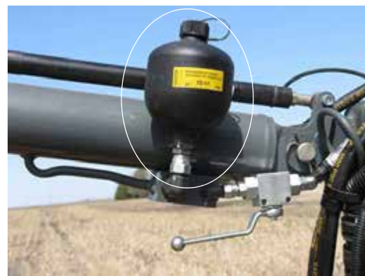
Accumulator -Typical View
