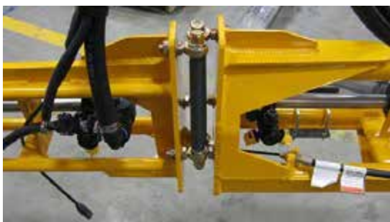
Outer Breakaway -Typical View
