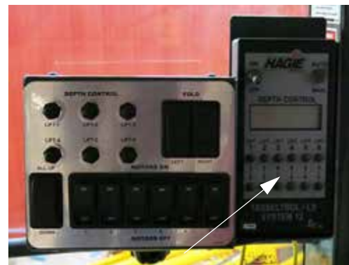
Tasselrol/LS System 12 Control Panel -Typical View
