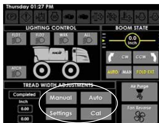
Tread Width Adjustment Buttons - Manual/Auto Tread (Located on the Auxiliary Controls Page)
