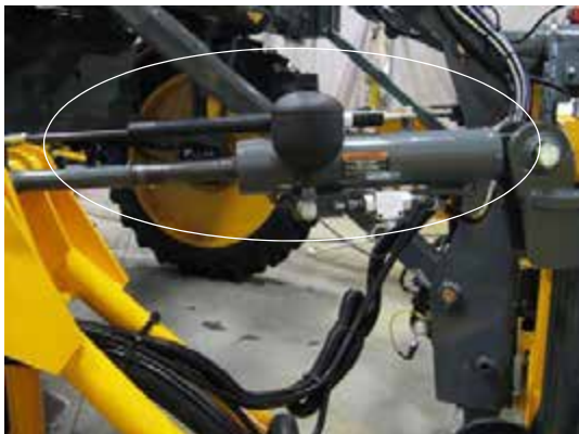
Level Cylinders -Typical View
