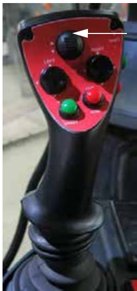
Transom Switch - UP (Located on the Hydrostatic Drive Control Handle) -Typical View
