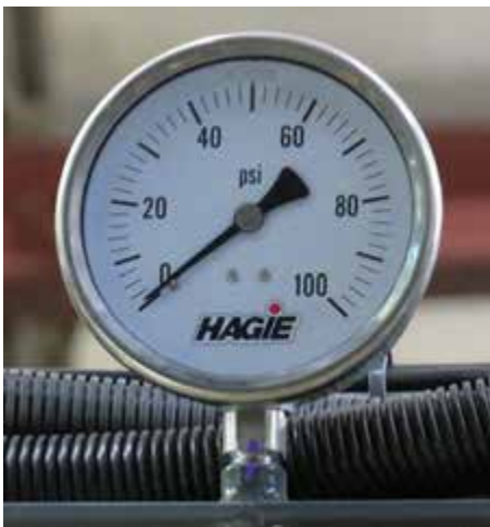
Pressure Gauge (Mounted on boom) -Typical View
