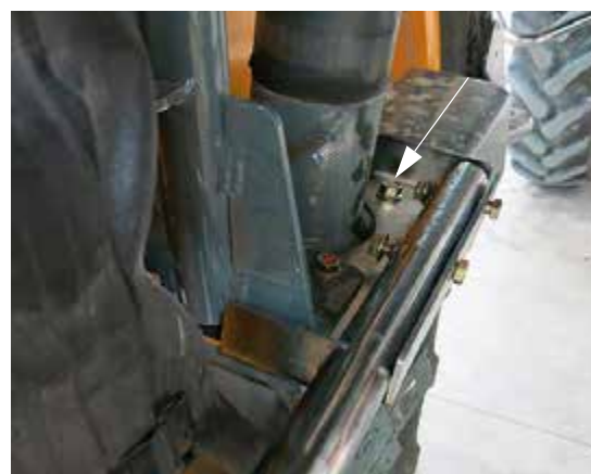
Mounting Plate Bolt -Typical View
