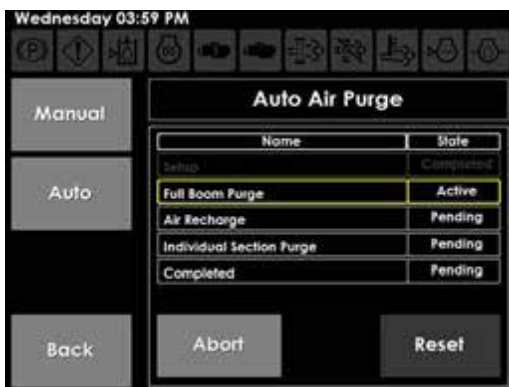
Air Purge Screen - Auto Cycle
