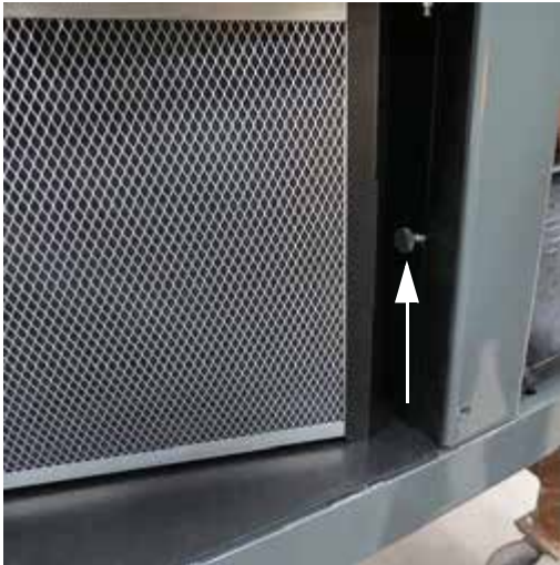
Security Screw (Located along the inside of filter compartment) -Typical View
