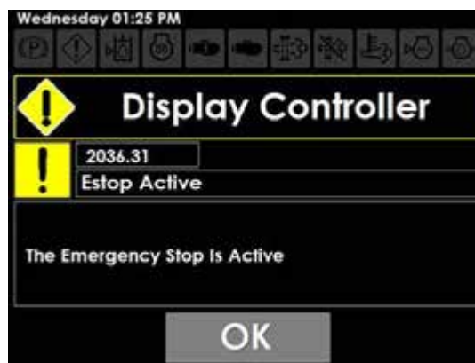
E-Stop Active Message (Located on the Machine Display)
