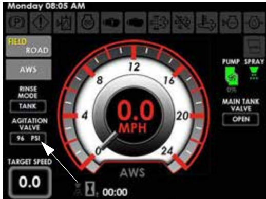
Agitation Valve Pressure Indicator (Located on the Machine Display Home Page - Road and Field Mode)
