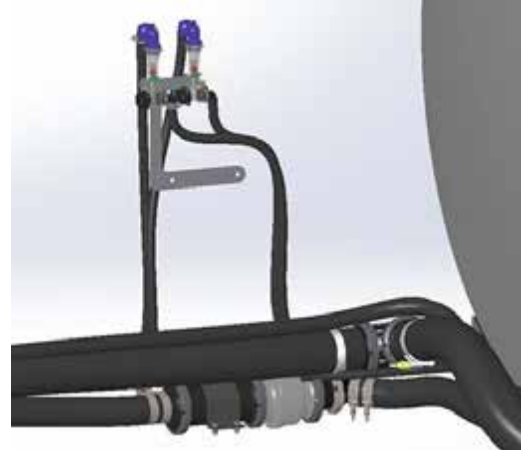
Flow Indicators (Located on the exterior right-hand side of cab) -Typical View
