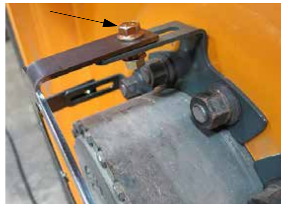
Hub Cap Adapter Bolt Installation -Typical View
