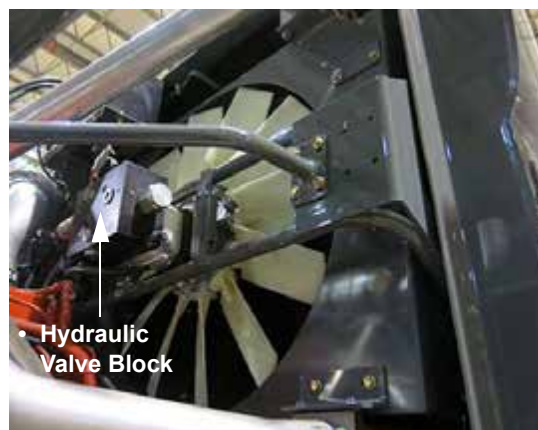
Reversible Fan (Located near the rear of machine - open hood to access) -Typical View
