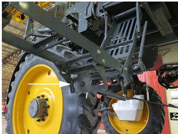
Ladder Platform -Typical View
