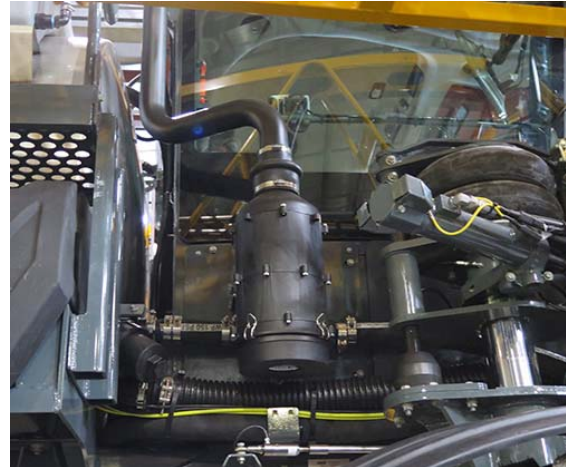
Cab Filtration System (Located on the right-hand side of the exterior cab) -Typical View
