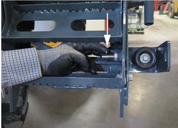
Security Pin (Located on lower right-hand side of folded ladder assembly) -Typical View
