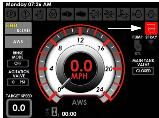
Insufficient Cab Air Pressure Indicator (Located on the Machine Display Home Page - Road or Field Mode)
