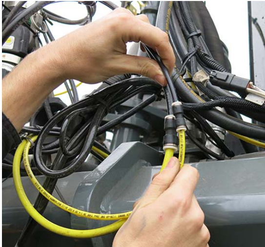
Foam Marker Connection (Located on the front right-hand side of machine) -Typical View
