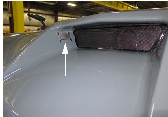
Hood Actuator Switch (Located near front top of hood) -Typical View
