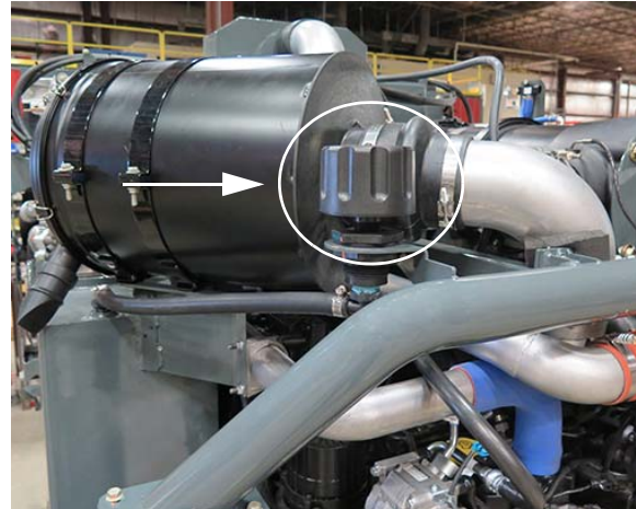
Breather Cap (Located on rear left-hand side of machine behind air intake filter) -Typical View
