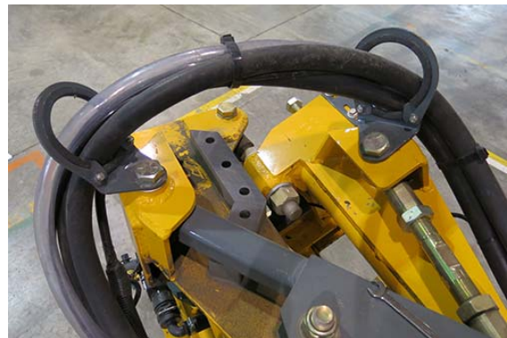
Boom Hose Clamp Installation -Typical View
