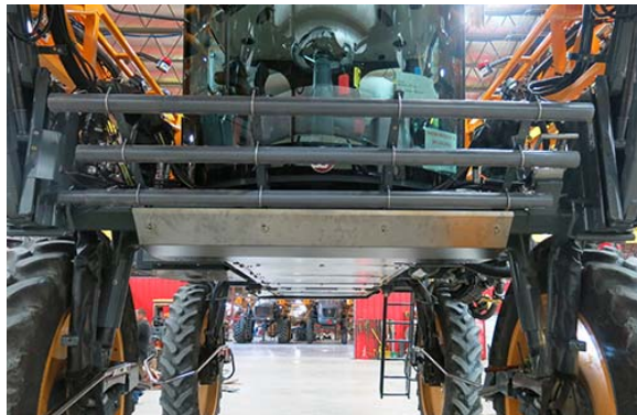
Brush Guard Installation -Typical View
