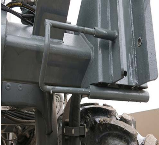
Lock Pin (Located on the front left and right-hand side of machine) -Typical View * Disengaged position shown
