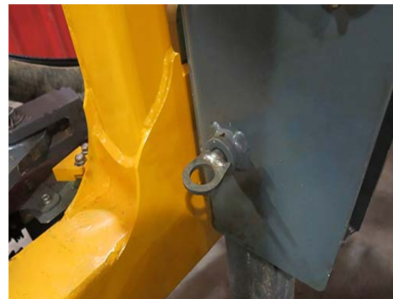
Lock Pin Removed -Typical View
