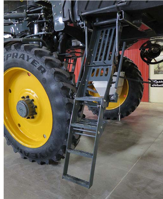
Fuel Fill Ladder (Lowered position shown) -Typical View
