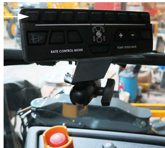
Boom Solution Valve Switches - Dual Product Section Keypad, Sections 10-14
