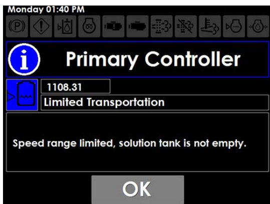
Limited Transportation Warning Message
