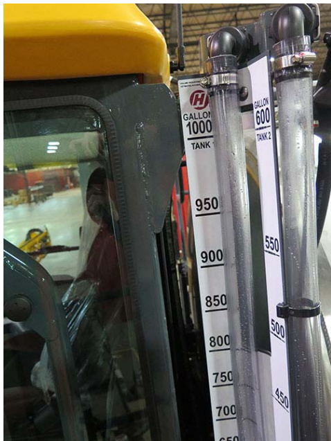
Dual Solution Tank Sight Gauge (Located behind the rear left-hand side of cab) -Typical View
