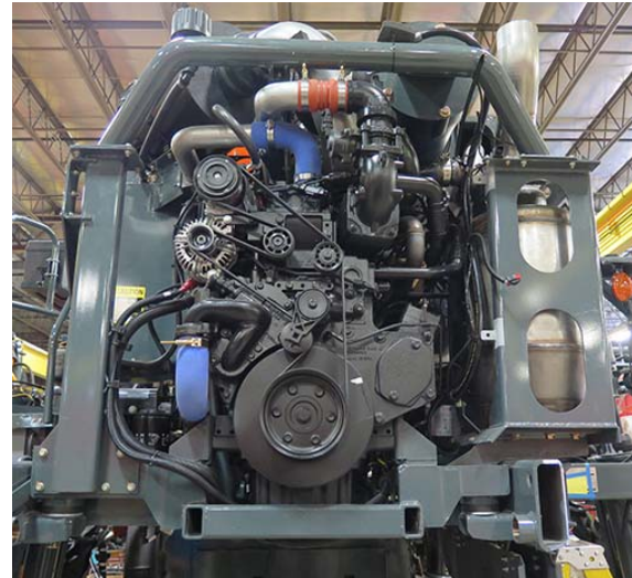
Final Tier 4 Diesel Engine (Located near rear of machine - open hood to access) -Typical View
