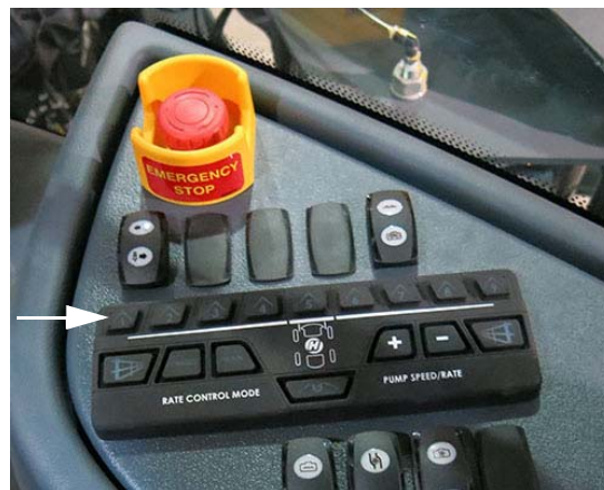
Boom Solution Valve Switches - Single Product Section Keypad, Sections 1-9
