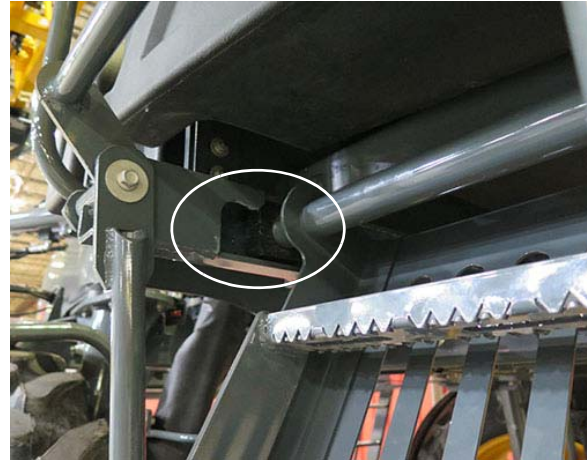
Ladder Disengaged from Track Detent (Left-hand side of ladder shown) -Typical View
