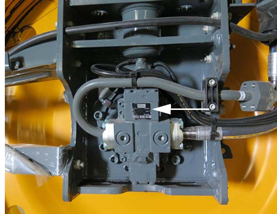
Wheel Motor Identification Plates -Typical View
