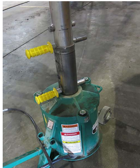
Lock Pin Installation -Typical View
