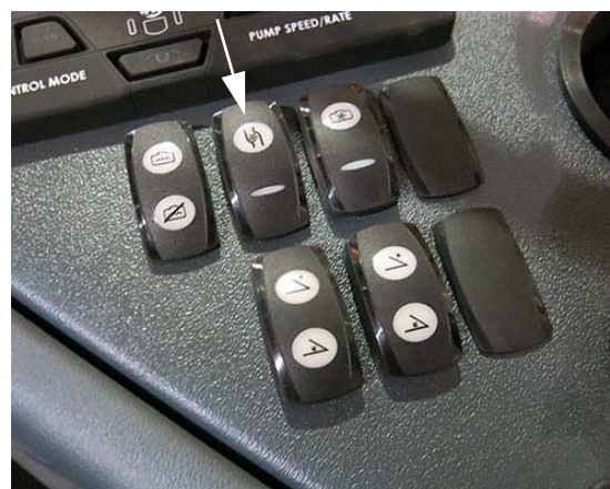
Solution Pump Switch - Primary (Located on the side console) -Typical View
