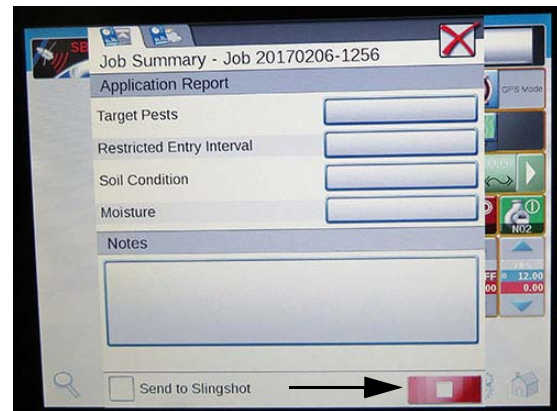
Stop Button (Located on the spray system console) -Typical View * Your machine may vary, depending on available equipment
