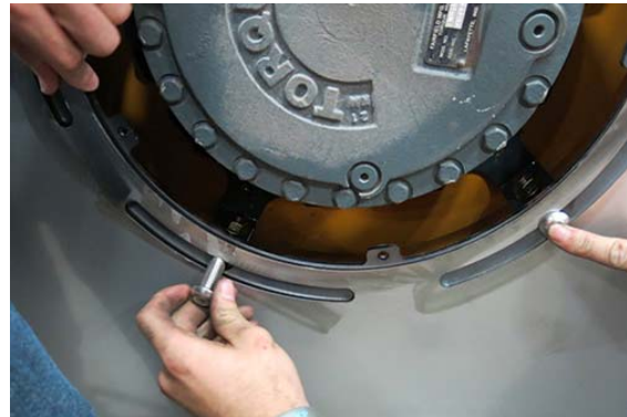
Wheel Cover Mounting Bolt Installation -Typical View
