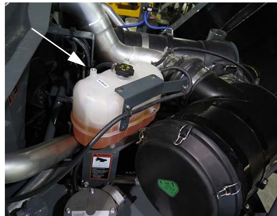
Surge Tank (Located near the rear of machine - open hood to access) -Typical View
