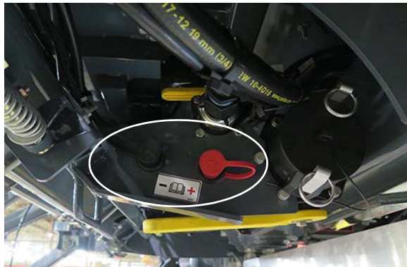
Power Ports (Located near front fill assembly) -Typical View
