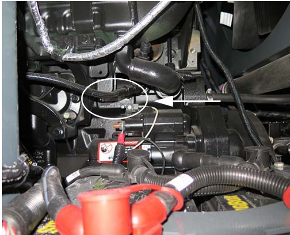
Engine Identification Plate -Typical View
