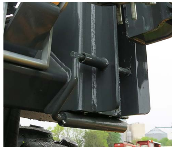
Lock Pin -Typical View * Engaged position shown
