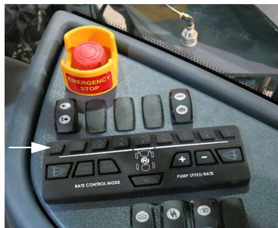
Boom Solution Valve Switches - Single Product Section Keypad (Located on the side console) -Typical View
