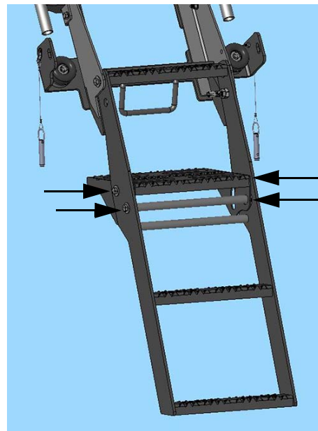
Lower Ladder Pivot Points - Platform (4) -Typical View
