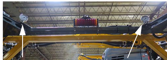
• Secondary Pressure Gauge • Primary Pressure Gauge
