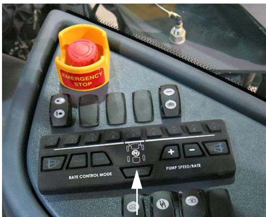
Rear Nozzle Switch (Located on the side console) -Typical View
