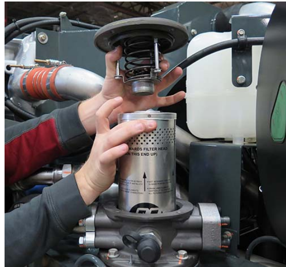
Return Filter (Located inside filter housing on top of hydraulic oil reservoir) -Typical View
