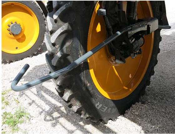
Installed Crop Divider -Typical View
