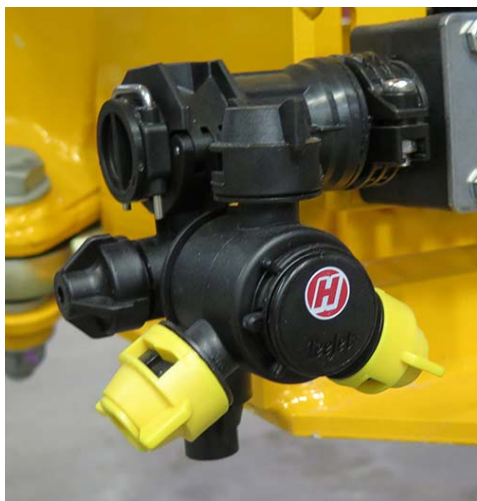
Nozzle Body (Located throughout boom) -Typical View
