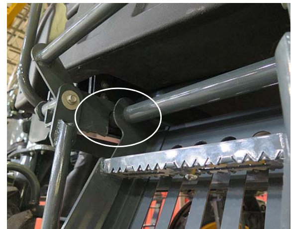
Ladder Engaged in Track Detent (Left-hand side of ladder shown) -Typical View
