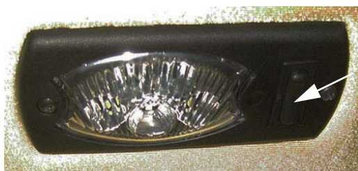
Interior Work Light Switch -Typical View
