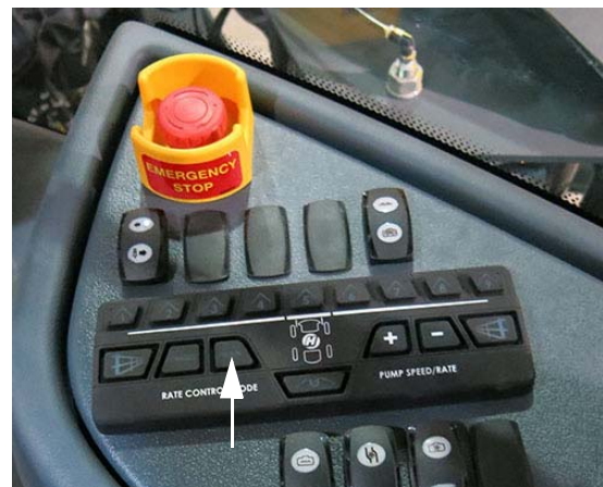
Manual "MAN" Rate Control Switch (Located on the side console) -Typical View
