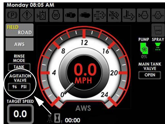
Agitation Valve Pressure Indicator (Located on the Machine Display Home Page - Field Mode)
