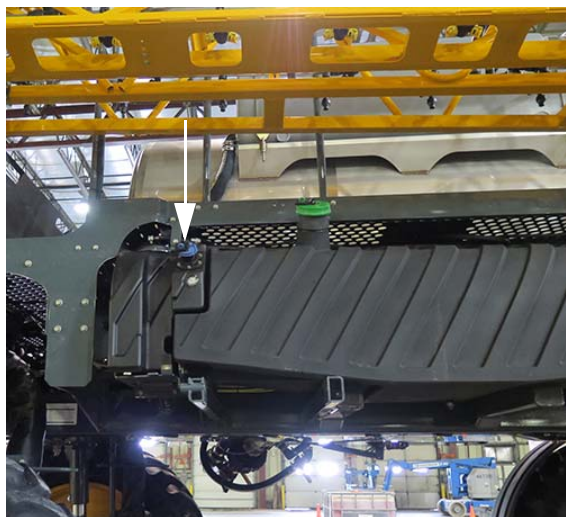
DEF Fill Cap (Located on front of DEF tank) -Typical View
