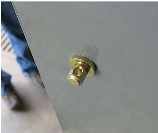
Hanger Pin Installation -Typical View
