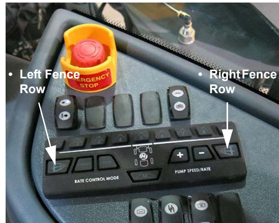
Fence Row Switches - Left/Right (Located on the side console) -Typical View
