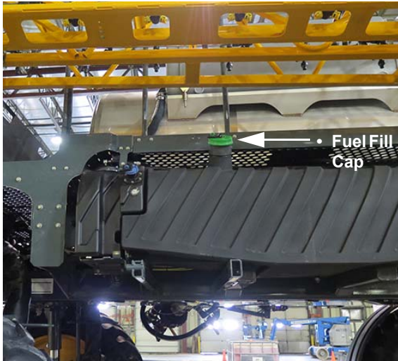
Engine Fuel Fill (Located on top of fuel tank on right-hand side of machine) -Typical View
