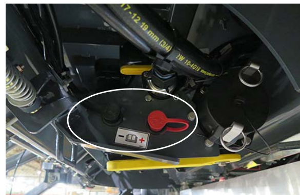
Power Ports (Located near front fill assembly) -Typical View
