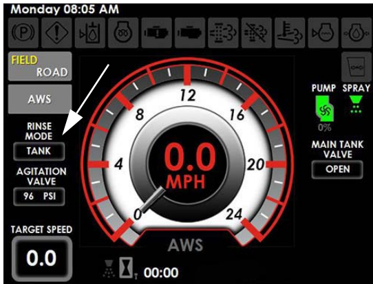
Rinse Mode Indicator (Located on the Machine Display Home Page - Field Mode)
