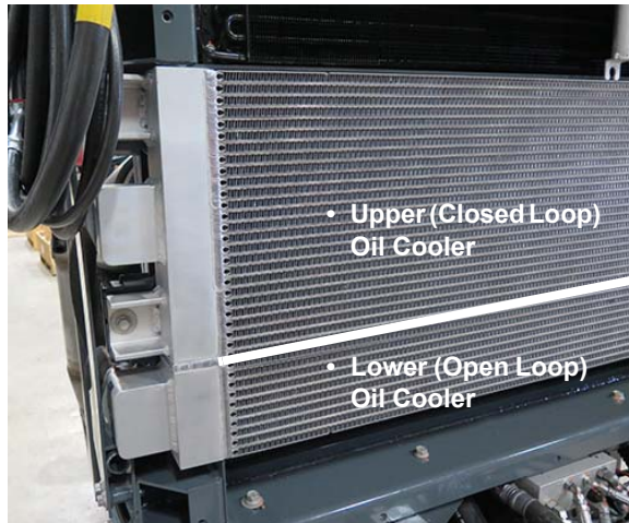
Oil Cooler (Located ahead of engine - remove radiator screen to access) -Typical View
