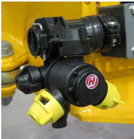
Nozzle Body (Located throughout boom) -Typical View
