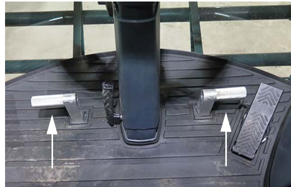
Operator Foot Pegs (Located on each side of the steering column) -Typical View
