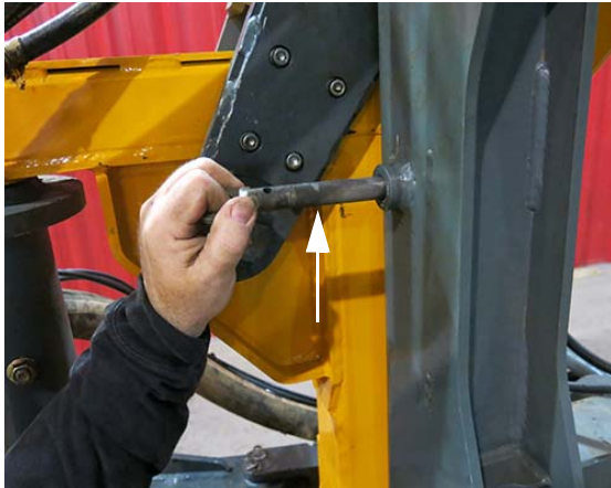
Mounting Bolt (Located on the outer side of transom frame) -Typical View
