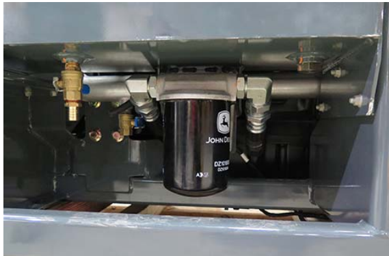
Engine Oil Filter (Located on rear left-hand side of machine below hydraulic oil reservoir) -Typical View
