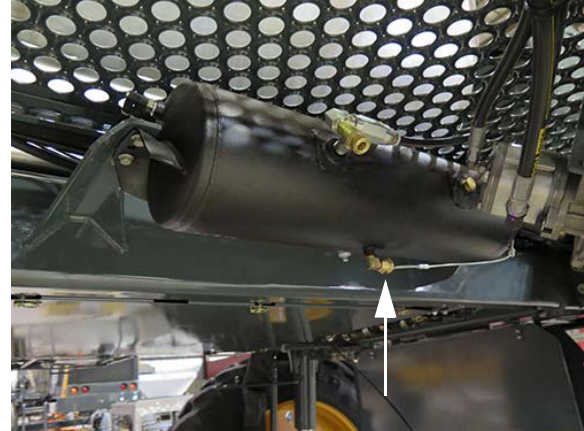
Tank Drain Valve (Main) (Located beneath platform on left-hand side of machine) * Pull DOWN to open -Typical View
