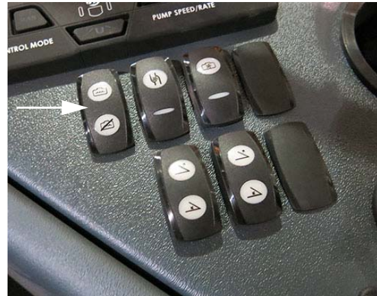
Main Tank Valve Switch (Located on the side console) -Typical View
