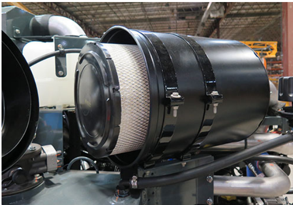
Engine Air Intake Filter (Shown with end cap removed) -Typical View
