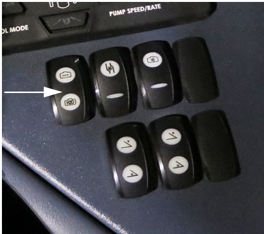
Tank Valve Selector Switch (Located on the side console) -Typical View
