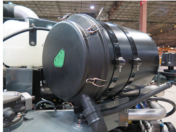
Engine Air Intake Filter (Located on rear left-hand side of machine - open hood to access) -Typical View
