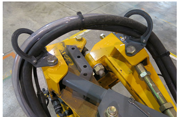
Boom Hose Clamp Installation -Typical View
