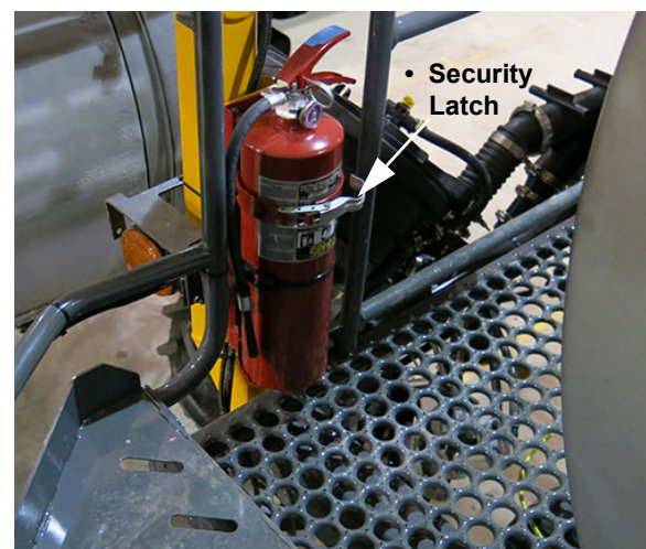
Fire Extinguisher (Located along platform on left-hand side of machine) -Typical View
