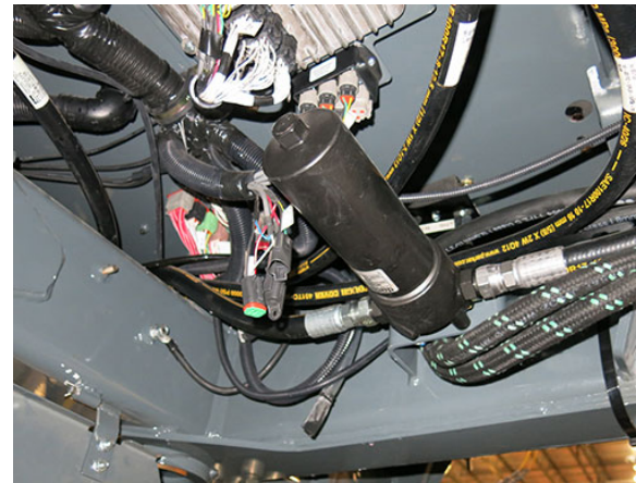
Pressure Filter (Located beneath right-hand side of machine - lower metal shield to access) -Typical View
