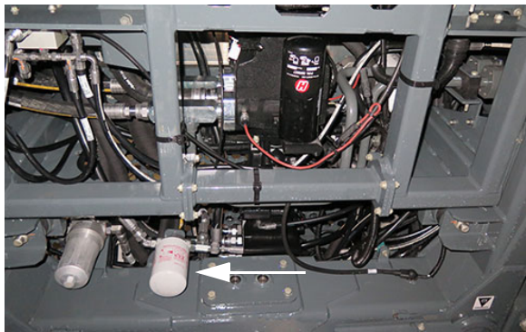
Case Drain Filter 2 (Located on left-hand side of machine ahead of engine frame) -Typical View
