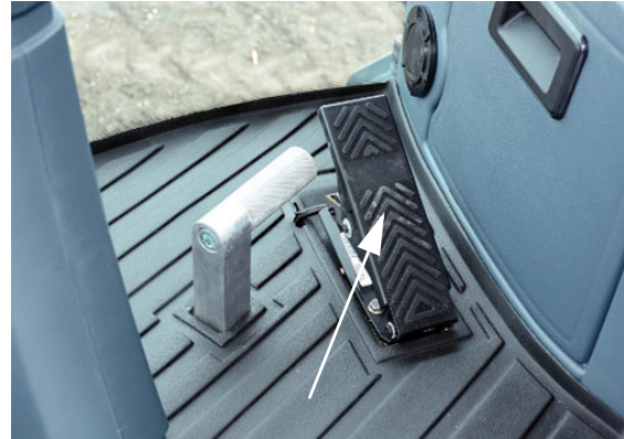
Decel Pedal (Located to the lower right-hand side of the steering column) -Typical View
