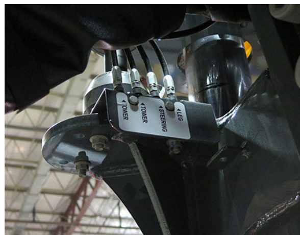
Grease Zerk Bank (4) (Located on the front side of each leg) -Typical View
