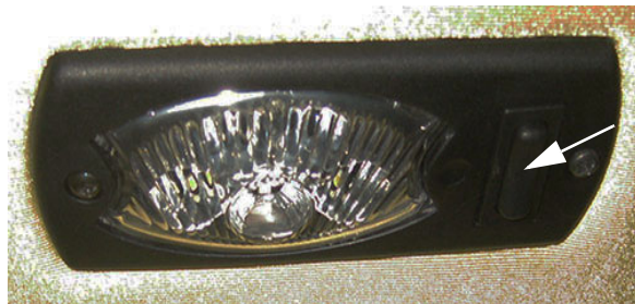
Interior Work Light Switch -Typical View
