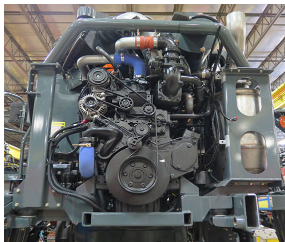
John Deere Final Tier 4 PSS 9.0L Diesel Engine -Typical View
