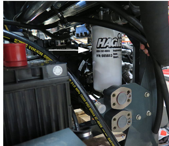
Case Drain Filter 1 (Located on right-hand side of machine near batteries) -Typical View
