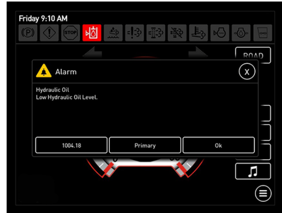
Low Hydraulic Oil Level Warning Message (Located on the Machine Display)
