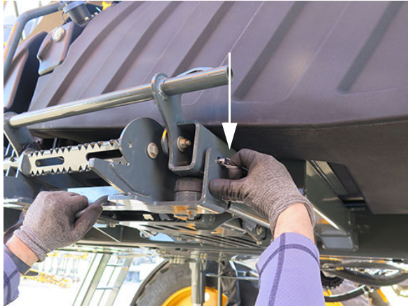
Lock Pins (2) (Located on each side of the ladder assembly) -Typical View
