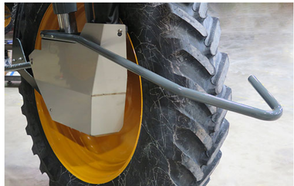
Installed Crop Divider -Typical View
