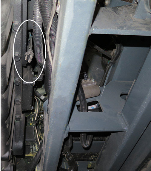
Engine Block Heater Power Cord (Located beneath machine along the right-hand side of engine) -Typical View
