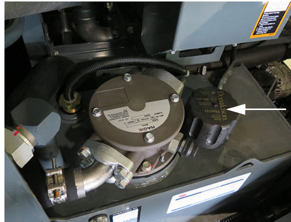
Breather Cap (Located on top of hydraulic oil reservoir) -Typical View
