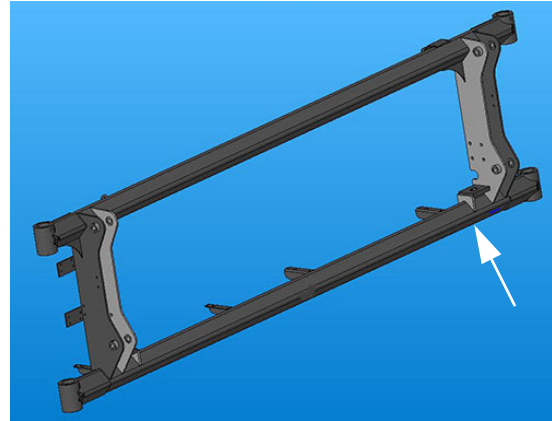
90/100' Steel Spray Boom Identification Plate -Typical View
