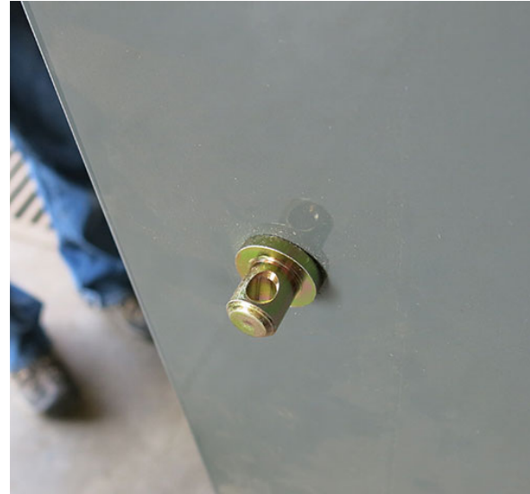
Hanger Pin Installation -Typical View
