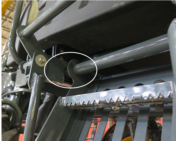
Ladder Engaged in Track Detent (Left-hand side of ladder shown) -Typical View
