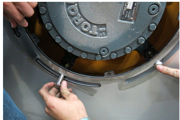
Wheel Cover Mounting Bolt Installation -Typical View
