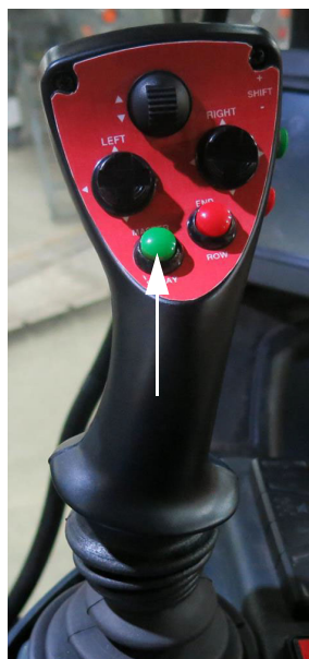
Master Spray Switch (Located on the Hydrostatic Drive Control Handle) -Typical View
