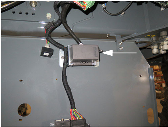
Solution Pump Relay Box (Located beneath front end of cab - lower panel to access) -Typical View
