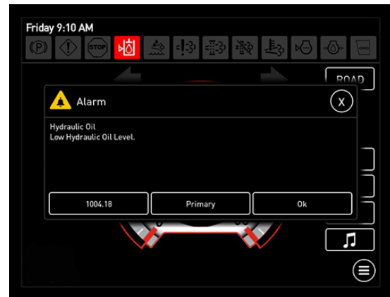
Low Hydraulic Oil Level Warning Message (Located on the Machine Display)
