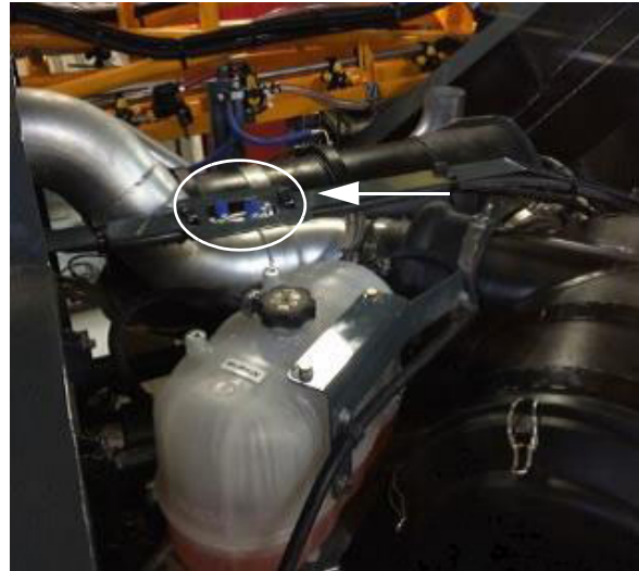
A/C Charge Ports (Located inside engine compartment - open hood to access) -Typical View
