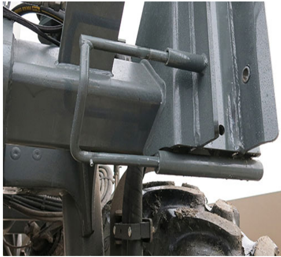
Lock Pin (2) (Located on the front left and right-hand side of machine) -Typical View * Disengaged position shown
