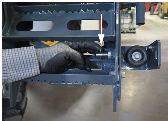
Security Pin (Located on lower right-hand side of folded ladder assembly) -Typical View
