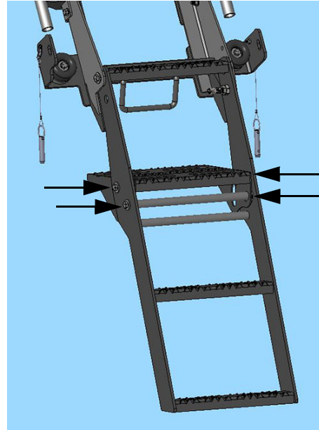
Lower Ladder Pivot Points - Platform (4) -Typical View
