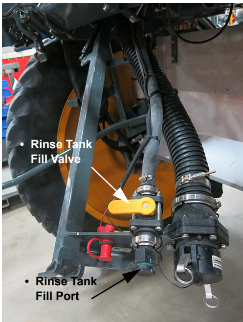
Front Fill Assembly (Lowered position shown) -Typical View
