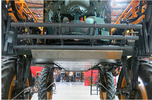
Brush Guard Installation -Typical View
