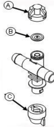
Nozzle Diaphragms and Spray Tips -Typical View
