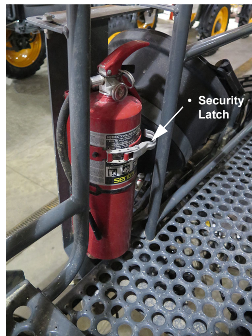
Fire Extinguisher (Located along platform on left-hand side of machine) -Typical View
