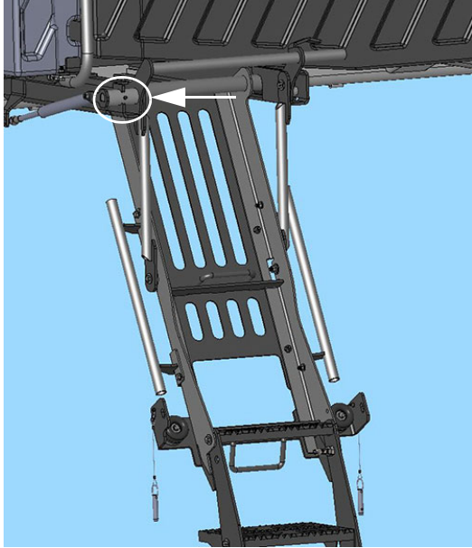
Gas Spring Axle Grease Zerk (Located near the top left-hand side of ladder) -Typical View
