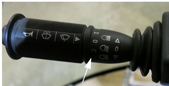
Windshield Wiper Speeds (Located on the turn signal lever) -Typical View
