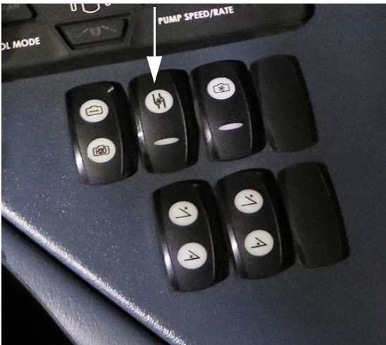
Solution Pump Switch - Primary (Located on the side console) -Typical View
