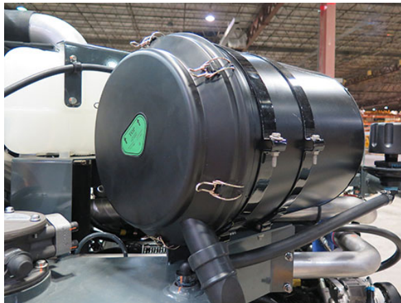
Engine Air Intake Filter - STS14/STS16 (Located on rear left-hand side of machine - open hood to access) -Typical View
