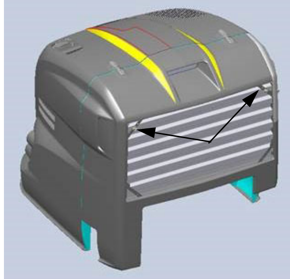
Radiator Screen Spring Clips (2) (Located on the top left and right-hand side of screen) -Typical View
