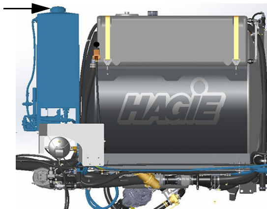
Fill Port Lid (Located on the top of chemical tank) -Typical View
