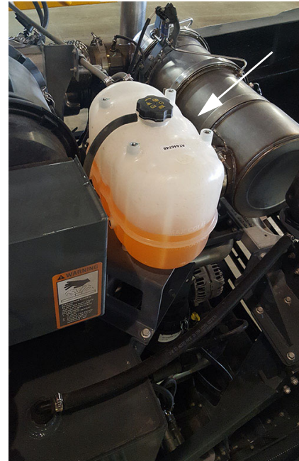
Surge Tank - STS10/STS12 (Located near the rear of machine - open hood to access) -Typical View
