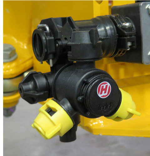
Nozzle Body (Located throughout boom) -Typical View
