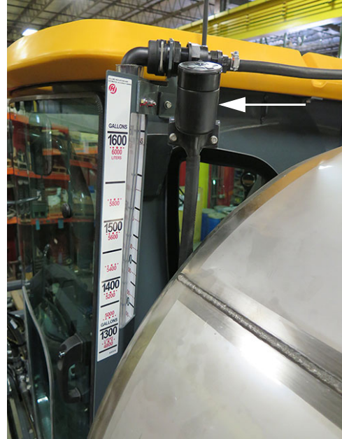
Windshield Washer Fluid Reservoir (Located behind the left-hand side of cab) -Typical View
