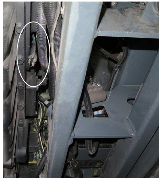
Engine Block Heater Power Cord - STS14/STS16 (Located beneath machine along the right-hand side of engine) -Typical View
