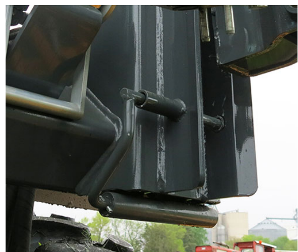
Lock Pin (2) -Typical View * Engaged position shown
