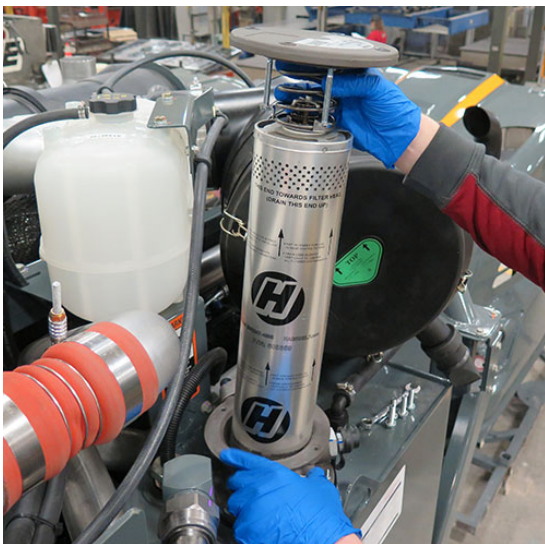
Return Filter (Located inside filter housing on top of hydraulic oil reservoir) -Typical View
