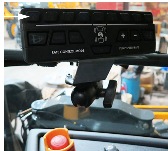
Boom Solution Valve Switches - Dual Product Section Keypad, Sections 10-14 (Mounted near the side console) -Typical View
