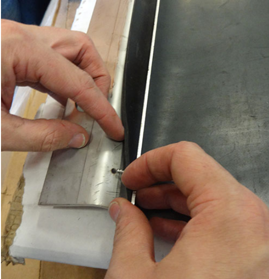
Brush Curtain Assembly -Typical View
