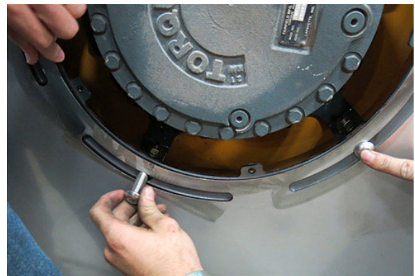
Wheel Cover Mounting Bolt Installation -Typical View
