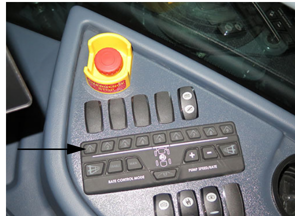
Boom Solution Valve Switches - Single Product Section Keypad, Sections 1-9 (Located on the side console) -Typical View
