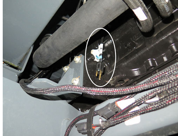
Engine Block Heater Power Cord - STS10/STS12 (Located beneath engine on left-hand of machine) -Typical View
