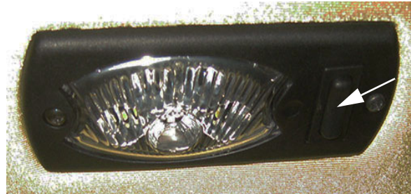
Interior Work Light Switch -Typical View
