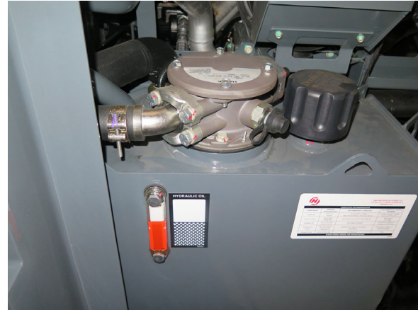
Hydraulic Oil Reservoir (Located on rear left-hand side of machine - open hood to access) -Typical View
