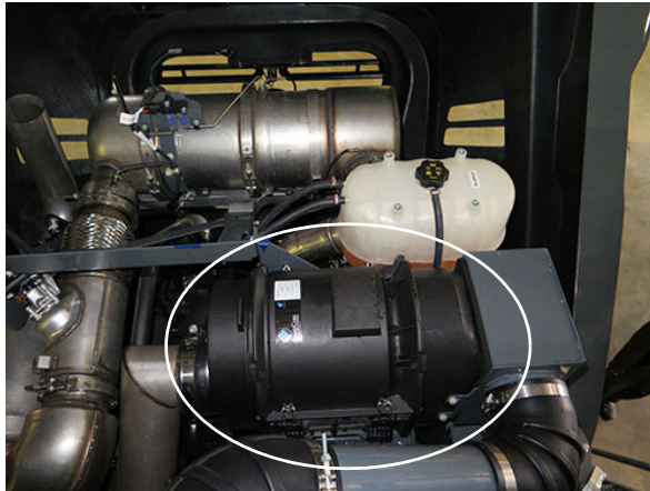
Engine Air Intake Filter - STS10/STS12 (Located on rear left-hand side of machine - open hood to access) -Typical View
