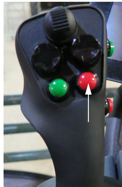
End Row Management Switch (Located on the Hydrostatic Drive Control Handle) -Typical View
