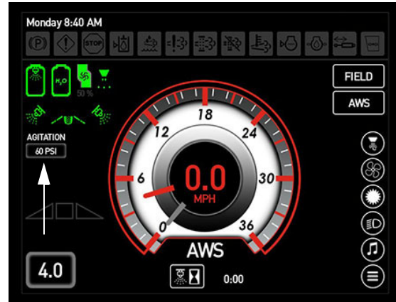
Agitation Valve Pressure Indicator (Located on the Machine Display Home Page - Field Mode)
