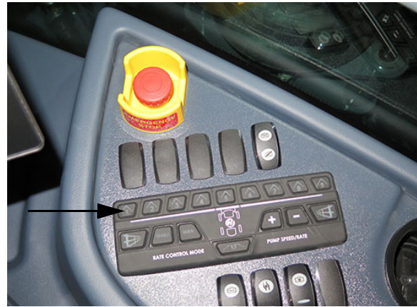
Boom Solution Valve Switches - Single Product Section Keypad (Located on the side console) -Typical View * Used with 9-section wet boom
