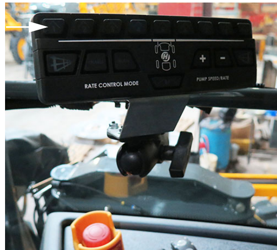
Boom Solution Valve Switches - Dual Product Section Keypad (Mounted near the side console) -Typical View * Used with 5-section wet boom
