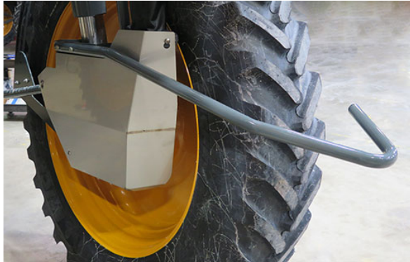
Installed Crop Divider -Typical View
