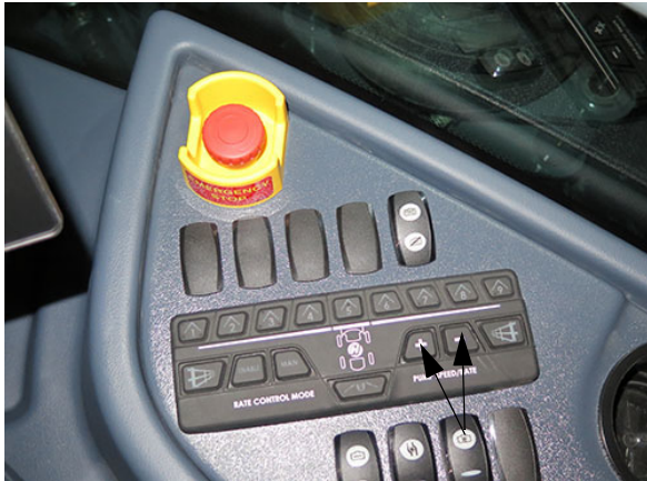
Pump Speed/Rate Switches (Located on the side console) -Typical View * Used for primary system only
