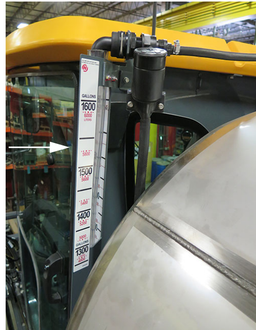
Solution Tank Sight Gauge (Located behind the rear left-hand side of cab) -Typical View
