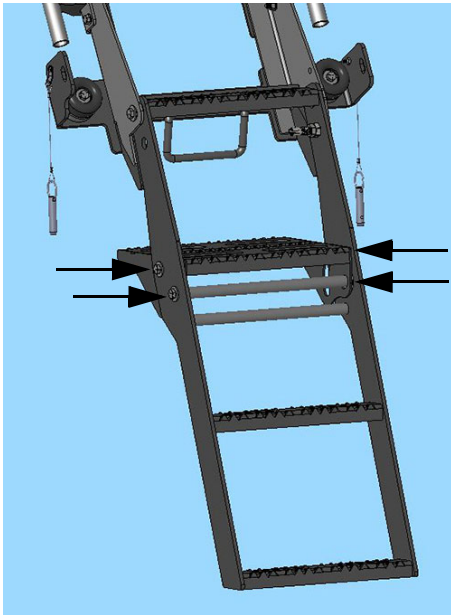
Lower Ladder Pivot Points - Platform (4) -Typical View
