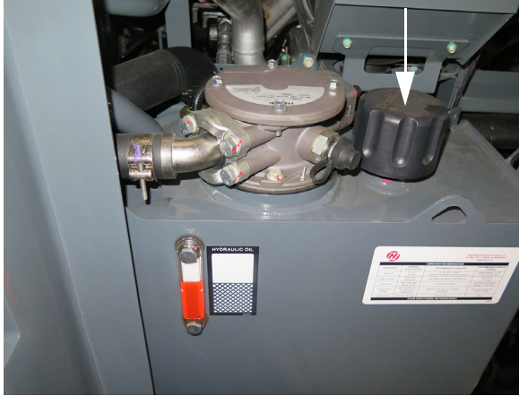
Breather Cap - STS10/STS12 (Located on top of hydraulic oil reservoir) -Typical View
