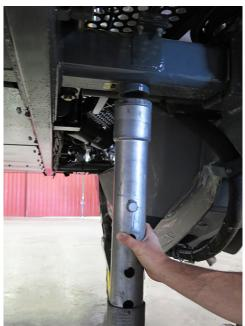
Insert Jack Around Lifting Point Containment Ring -Typical View
