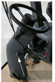
Steering Column Tilt Adjust Button (Located on the left-hand side of the steering column) -Typical View
