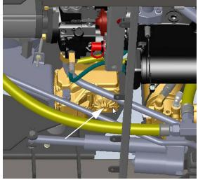
DEF Supply Module Filter (Closeup View)
