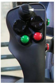
All Up/Down Switch (Located on the Hydrostatic Drive Control Handle) -Typical View
