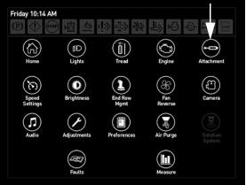
Attachment Button (Located on the Machine Display Main Menu)
