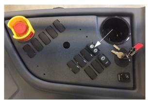
4-2 Slide Extension Switch (Located on the side console) -Typical View
