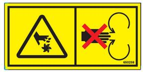
CAUTION SEVERING OF FINGERS OR HAND. DO NOT PLACE FINGERS OR HAND NEAR A MOVING CUTTER BLADE, ATTEMPT TO STOP A MOVING CUTTER BLADE, OR PERFORM MAINTENANCE NEAR A MOVING CUTTER BLADE.
