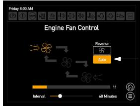
Auto Button (Located on the Engine Fan Control Screen)
