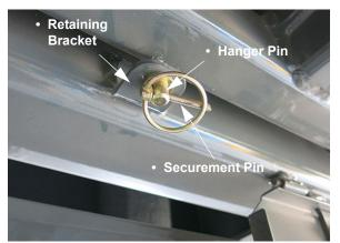
Retaining Bracket/ Securement Pin Assembly -Typical View
