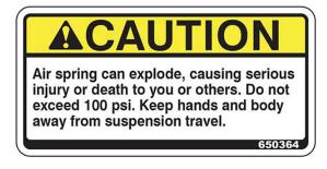
NOTE: Inspect air bags daily for leaks and/ or cracking.
