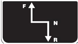
Hydrostatic Drive Control Handle -Typical View
