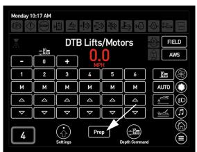
Prep Button (Located on the Machine Display DTB Lifts/Motors Screen <u>or</u> DTB Depth Command Screen)
