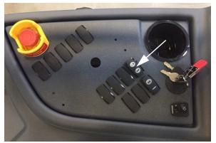
4-2 Detasseler Switch (Located on the side console) -Typical View
