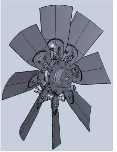
Variable Pitch Fan (Located near the rear of machine - open hood to access) -Typical View
