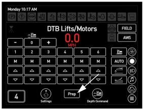
Prep Button (Located on the Machine Display DTB Lifts/Motors Screen <u>or</u> DTB Depth Command Screen)
