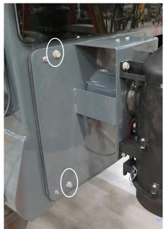
Mounting Bolts (4) (Two located on each side of access panel on the right-hand side of cab) -Typical View
