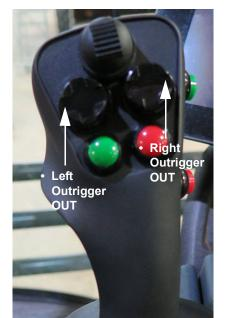
Outrigger Fold Switches - Left/Right (Located on the Hydrostatic Drive Control Handle) -Typical View
