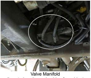
(Located on the underside of machine) -Typical View
