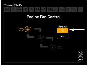
Reverse Button (Located on the Engine Fan Control Screen)
