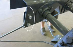
Install four (4) Stalk Guide Nuts onto the bolts and tighten with a 9/16" wrench
