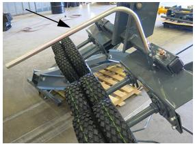
Deflector Shield Mounting Tube -Typical View
