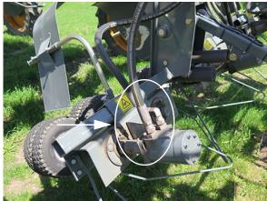
Quad Puller Hydraulic Connections -Typical View
