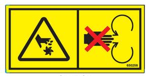
**CAUTION** SEVERING OF FINGERS OR HAND. DO NOT PLACE FINGERS OR HAND NEAR A MOVING CUTTER BLADE, ATTEMPT TO STOP A MOVING CUTTER BLADE, OR PERFORM MAINTENANCE NEAR A MOVING CUTTER BLADE.
