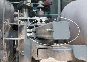
Tread Adjust Bearing Slide Path (4) (Located on each leg) -Typical View
