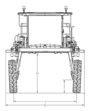
\* Tread width is measured from center of tire at ground.
