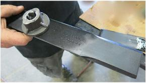
Install Cutter Blade Adapter Plug onto center of blade
