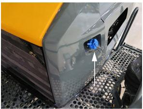
DEF Fill Cap (Located on left-hand side of hood) -Typical View
