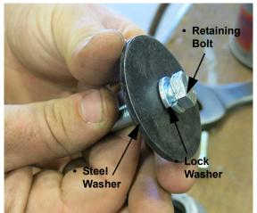
Cutter Blade Bolt/Washer Assembly -Typical View
