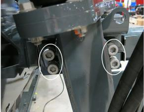
Tread Adjust Bearing Bolts - Top/Side (Located on each leg) -Typical View
