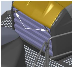
Radiator Screen Spring Clips (2) (Located on the top left and right-hand side of screen) -Typical View
