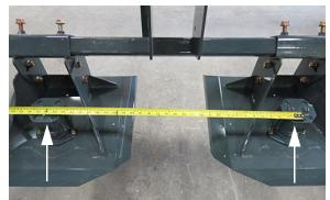
Measure 30" (76.2 cm) from center of each cutter head motor
