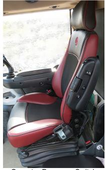
Operator Presence Switch (Located inside the operator's seat) -Typical View
