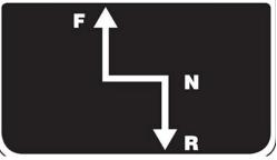
Hydrostatic Drive Control Handle -Typical View
