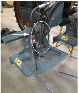
Cutter Head Hydraulic Connections -Typical View
