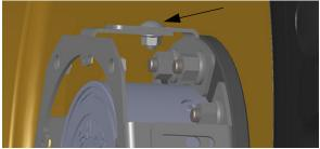
Hub Cap Adapter Bolt Installation -Typical View
