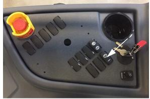
Traction Valve Switch (Located on the side console) -Typical View
