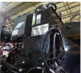
Hydraulic Oil Reservoir (Located near rear left-hand side of machine - open hood to access) -Typical View
