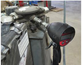
Filling Tank Through Hydraulic Oil Fill Port -Typical View
