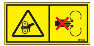
**CAUTION** RISK OF INJURY FROM ROTATING TIRES. DO NOT PLACE FINGERS OR HAND NEAR MOVING QUAD PULLER TIRES, DISLODGE A WEDGED OBJECT FROM MOVING TIRES, OR PERFORM MAINTENANCE NEAR MOVING TIRES.
