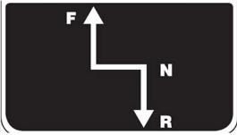
Hydrostatic Drive Control Handle -Typical View
