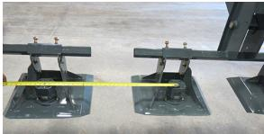
Measure 30" (76.2 cm) from center of each cutter head motor, across each lift mount
