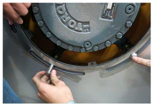
Wheel Cover Mounting Bolt Installation -Typical View
