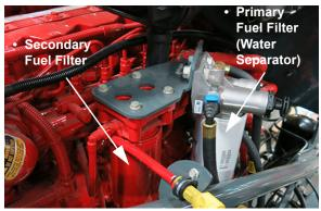
Primary and Secondary Fuel Filters (Located on left-hand side of engine through access opening) -Typical View
