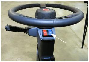
Highway Running Lights Switch (Located on steering column) -Typical View
