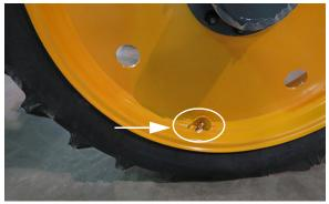
Valve Stem (4) (Located on the inside of each wheel) -Typical View
