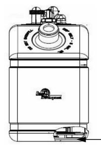
DEF Suction Strainer (Located near bottom of the DEF Tank) -Typical View
