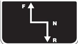
Hydrostatic Drive Control Handle -Typical View
