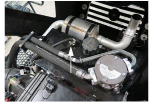
Level/Temp Sensor (Located on top of hydraulic oil reservoir - open hood to access) -Typical View
