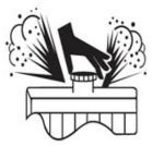
• Disconnect battery ground cable and turn the Battery Disconnect Switch OFF before servicing the electrical system or welding on the machine.
