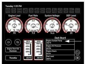
Engine Coolant Temperature (Located on the Engine Diagnostics Screen)
