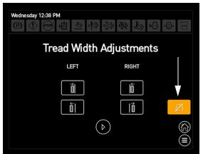
Rear-view Camera Activation Button (Located on the Tread Width Adjustments Screen and Individual Tread Screen) - Deactivated (illuminated) position shown
