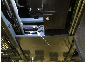
Pressure Filter (Located beneath center of machine) -Typical View \* Lower Tall Crop Package Belly Shield to access - if equipped
