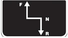
Hydrostatic Drive Control Handle -Typical View
