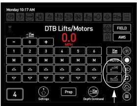
Lift Icon Buttons (All Up/Down) (Located on the Machine Display DTB Lifts/Motors Screen) -Typical View
