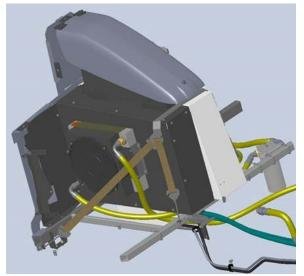
Auxiliary Hydraulic Oil Cooler (Located inside the FRM behind left-hand side of cab) -Typical View
