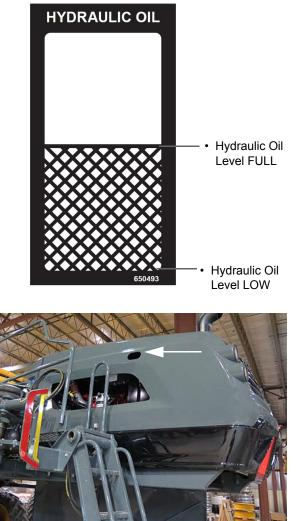
Hydraulic Oil Reservoir Sight Gauge (Located near the rear left-hand side of machine) -Typical View
