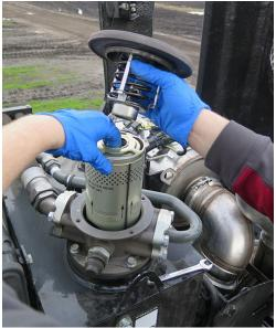
Return Filter 1 (Located inside filter housing) -Typical View
