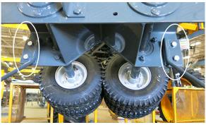
• Install four (4) Stalk Guide Bolts through the front side of each Stalk Guide/Quad Puller
