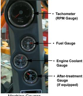
Machine Gauges (Located on cab A-post) -Typical View
