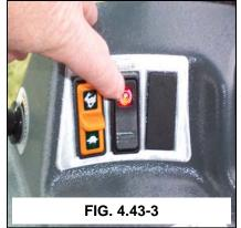
**LADDER-** To raise or lower the ladder you will need to locate the BRAKE/LADDER switch at the front of the right hand console (fig. 4.43-3). When the brake is applied the ladder will lower automatically (fig. 4.43-1). The ladder will not raise (fig. 4.43-2) until the machine is running and the switch has been returned to the OFF position.
