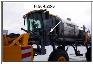
TURN SIGNALS— To activate the front turn signals (fig. 4.22-3) and the rear turn signals (fig. 4.22-4 and 5), move the turn signal lever (fig. 4.21-2, item E) forward, away from the operator, to signal a right turn and back, toward the operator, to signal a left turn. Steering column— mounted turn signal indicators will correspondingly flash when either turn signal is activated. The turn signal switch is not a self— centering switch; you must return it to the "OFF" position by
