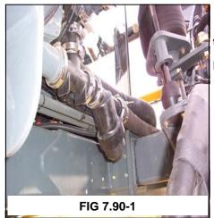
Check all strainers occasionally for blockage and replace them if they show signs of deterioration. Refer to the Hagie Parts Manual for replacement part numbers and specific locations.
