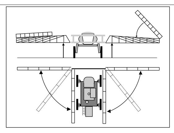
The booms should always be cradled before traveling, transporting, or parking for an extended period of time. The booms must be folded when cradled.
