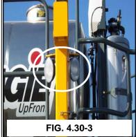
The work lights (fig. 4.30-3), located on each boom cradle, one facing forward and one facing backward, are activated by pressing the other switch located on the right upper cab headliner. These lights can also be used when operating in the field after dark. Turn them off before entering a public roadway.
