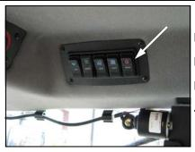
HEATED MIRRORS— The mirrors are heated for easy de-icing. To activate the mirror heat, depress the top of the switch. To turn the heat off, depress the bottom of the switch (fig. 4.31-1).
