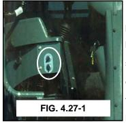
**POWER PORTS-** On the front of the side console there are two power ports (fig. 4.27-1) for extra equipment to be plugged in. They are each protected by a 15 amp fuse. They are not intended for the permanent connection of extra systems to the sprayer. There is a terminal strip intended for the installation of extra radios and computer equipment. See the SERVICE section E on the electrical components. Top port is 12V all the time and bottom port is powered by key.
