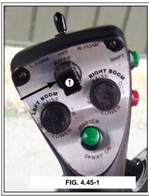
To raise and lower the transom/boom assembly, depress the "square rocker" on the hydrostatic lever (fig. 4.45-1) and move it either UP or DOWN. While pressed, it will activate the transom lift cylinders (fig. 4.45-2).
