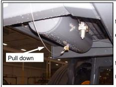
**WET TANK**Drain the wet tank (fig. 7.99-3) daily to prevent system condensation from contaminating the engine air compressor or dryer.
