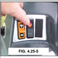
**PARKING BRAKE-** The parking brake switch is located next to the throttle switch on the side console. The switch also controls the ladder. The brake switch must be on to lower the ladder and to run the side fill or pressure washer (if equipped).
