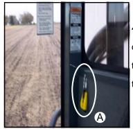
**RES-Q-ME TOOL/ EMERGENCY EXIT**— The RES-Q-ME tool (fig. 4.33-1) located on the right rear cab frame, is used for an emergency exit. The device, when firmly pressed against any glass in the cab, will automatically trigger shattering the glass. Do not look directly at the glass as you use the tool.
