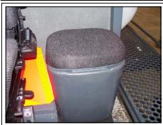
BUDDY SEAT- The buddy seat (fig. 4.34-1) was designed as an instructional tool. It is specifically designed for a "co-pilot" to be seated in a good position to be taught how to use the sprayer.
