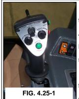
HYDROSTATIC LEVER— The hydrostatic lever is used to control the direction of motion of the machine and the speed at which it travels. It is a part of the ACE hydrostatic drive system or the Automatically Controlled Engine Hydrostatic Drive. To learn more about the ACE system, refer to the OPERATING SYSTEMS section B on the hydrostatic drive system.
