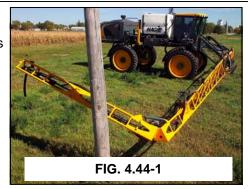
All GST spray booms are equipped with a hydraulic breakaway circuit. When folded out as a 100 foot spray boom, a one-way hydraulic circuit on the outer boom section provides outer boom breakaway functions. The outer breakaway is self-resetting and will return to normal operating position after it has cleared the hazard (fig. 4.44-1).
