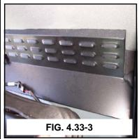
**CAB FILTERS**— Inside the cab are two filters (fig. 4.33-3), a charcoal filter and a paper filter. Refer to the SERVICE section B on filters for maintenance information. Refer to the Hagie GST20 Part Manual for replacement part information.
