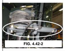
**SOLUTION PUMP**– The solution pump is a centrifugal pump controlled hydraulically with the pulse width modulated control valve. The valve is controlled by the Raven console per the calibration settings entered by the operator.
