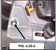
BRUSH CONTROL- The brush control dial is used to control the speed that the brushes are turning. The dial is only functional when the FLOAT and WORK MODE switches on the side console are on and the MAIN SPRAY CONTROL/ BRUSH CONTROL switch on the hydrostatic lever is activated.
