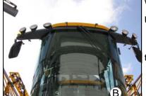
with a green UV reflective tint and the side and back panels are flat with a UV reflective gray tint.
