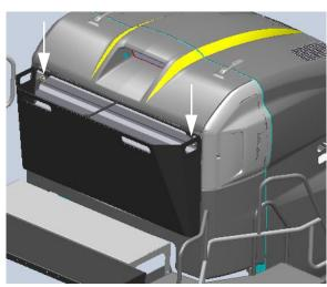
Engine Scoop Spring Clips - *if equipped*(Located on the top left and right-hand side of inside scoop)
