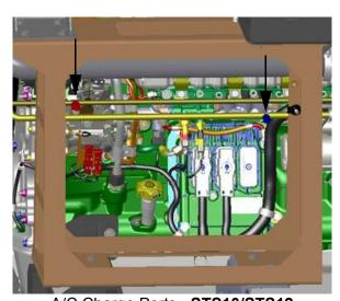
A/C Charge Ports - STS10/STS12 (Located on the right-hand side of machine - open hood to access) -Typical View
