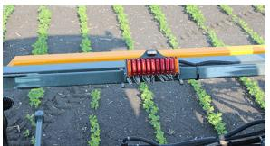
Boom Solution Valve Indicators (Located on transom) -Typical View \* Used for primary system only
