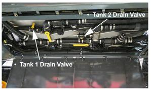
Solution Tank Drain Valves - Tanks 1 and 2 (Located beneath the solution tank on underside of machine)
