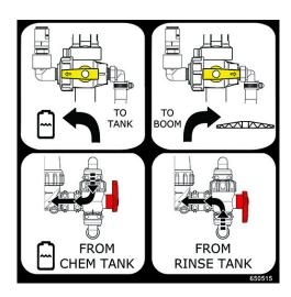
Run the Injection Pump(s) with the Outlet Selector Valve(s) (located on the front of injection pump(s)) in the "TO BOOM" position.
