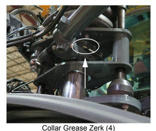
(Located beneath each air bag mounting plate)
