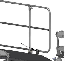
Hand Wash Foot Pedal (Located along the left-hand lower handrail)
