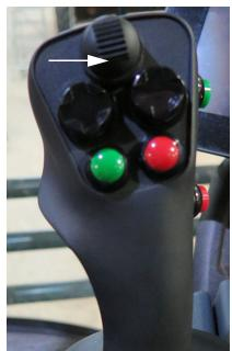
Transom Switch - DOWN (Located on the Hydrostatic Drive Control Handle)
