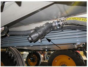
Solution Line Strainer (Located beneath the center right-hand side of machine) -Typical View
