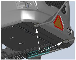
Brush Curtain Attached to Hood (Equipped with Rear Boom)
