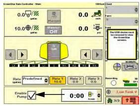
"Enable Pump" Check Box - **Secondary**(Located on the Precision Display
