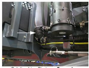
Solution Line Strainer - **Secondary**(Located near the front right-hand side of machine)
