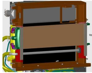
Oil Cooler - **Single Core**(Located ahead of engine remove radiator screen to access)
