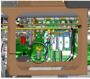
Engine Oil Fill - **STS10/STS12** (Located on the right-hand side of machine - open hood to access)
