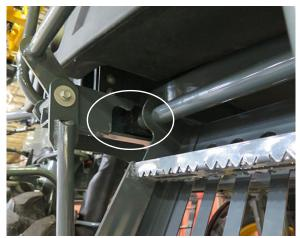
Ladder **Disengaged** from Track Detent (Left-hand side of ladder shown)
