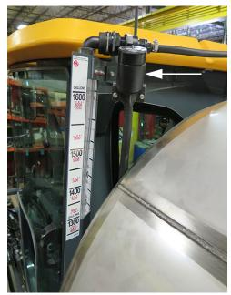
Windshield Washer Fluid Reservoir (Located behind the left-hand side of cab)
