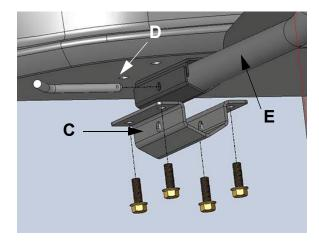
5. While maintaining position, install the Bent Pull Hitch Pin (F) through the aligned holes of the boom mounting assembly on each side.
