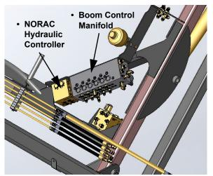
Boom Control Manifold and NORAC Hydraulic Controller (Located on the boom lift arm assembly)
