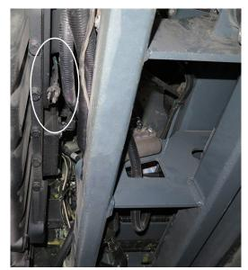
Engine Block Heater Power Cord
