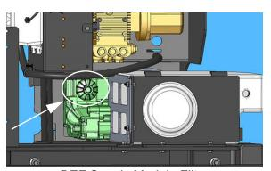
DEF Supply Module Filter (Located beneath DEF Supply Module access from underside of machine) -Typical View
