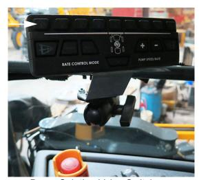
Boom Solution Valve Switches -**Dual Product Section Keypad**(Mounted near the side console)
