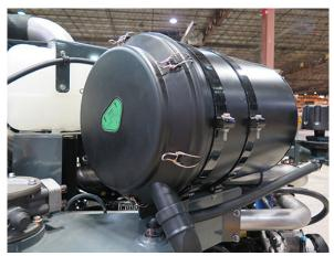
Engine Air Intake Filter - **STS14/STS16**(Located on rear left-hand side of machine - open hood to access)
