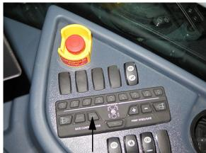
Manual "MAN" Rate Control Switch (Located on the side console)
