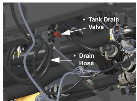
Tank Drain Valve (Lower)/Drain Hose (Located beneath platform behind solution tank)
