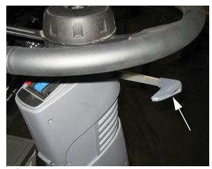
Steering Wheel Telescope Adjust Handle (Located on the right-hand side of steering column)
