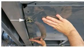
Securement Pin (Installed into Hanger Pin) -Typical View
