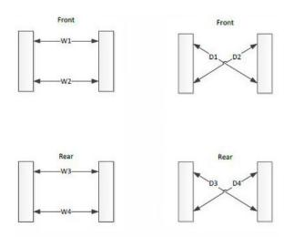
Continue to cycle between Steps 5-6 and 7-8 until the width measurements match and the diagonal measurements match. Then and only then are the wheels parallel to each other and the frame.
