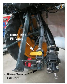
Front Fill Assembly (Lowered position shown)
