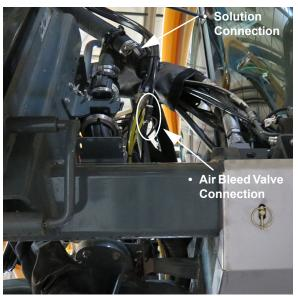
Solution and Air Bleed Valve Connections - **Standard**
