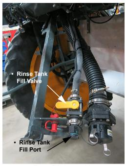
Front Fill Assembly (Lowered position shown)
