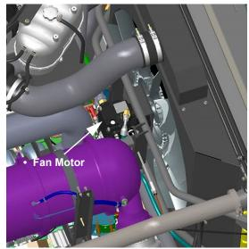
Reversible Fan - **STS14/STS16** (Located near the rear of machine - open hood to access)
