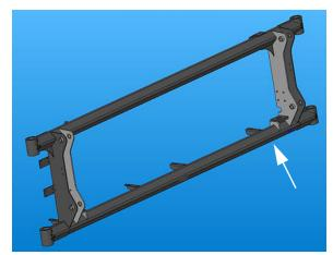
90/100' Steel Spray Boom Identification Plate -Typical View
