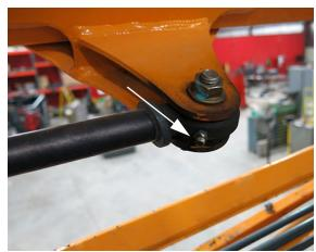
Boom Breakaway Cylinder Rod End -Typical View
