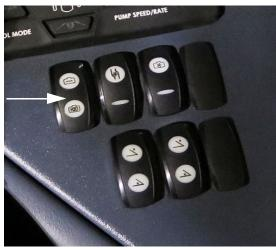
Tank Valve Selector Switch (Located on the side console)
