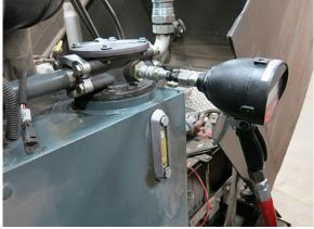
Filling Tank Through Hydraulic Oil Fill Port
