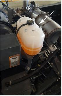
Surge Tank - **STS10/STS12**(Located near the rear of machine - open hood to access)
