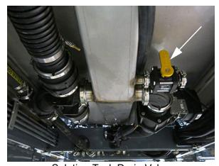
Solution Tank Drain Valve (Located beneath the solution tank on underside of machine)
