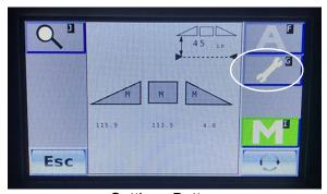
Settings Button (Located on the Main Run Screen) -Typical View
