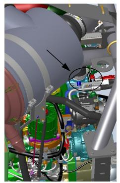
A/C Charge Ports - **STS14/STS16** (Located in the rear left-hand engine compartment - open hood to access)
