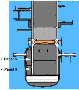
Rear Belly Shield Installation
