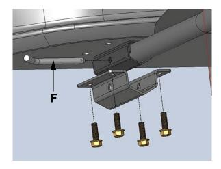
6. Ensuring the boom mounting hardware is aligned, hand-tighten the four (4) Boom Mounting Bolts (G) until snug on each side.
