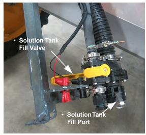
Front Fill Assembly (Lowered position shown)
