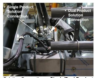
Solution Connections - **Single/Dual Product**(Located on the front right-hand side of machine)
