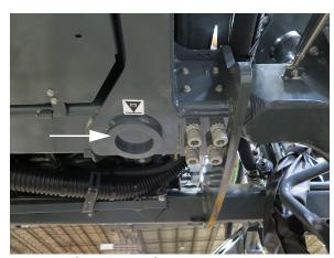
Lifting Point Containment Ring (Located on the frame near each leg)
