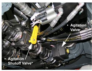
Agitation Valve and Agitation Shutoff Valve (Located beneath rear of machine)
