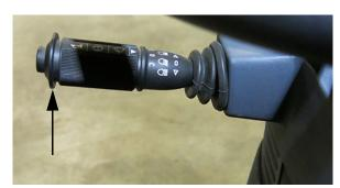
Windshield Washer Button (Located on the end of the turn signal lever) -Typical View
