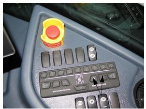
Pump Speed/Rate Switches (Located on the side console)
