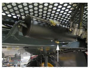
Tank Drain Valve (Main)
