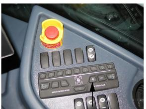
"+" Pump Speed/Rate Switch (Located on the side console)
