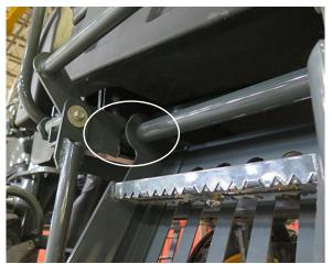
Ladder **Engaged** in Track Detent (Left-hand side of ladder shown)
