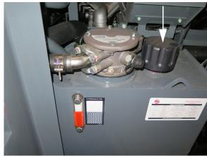
Breather Cap - STS10/STS12 (Located on top of hydraulic oil reservoir) -Typical View
