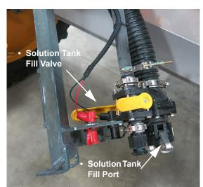
Front Fill Assembly (Lowered position shown)
