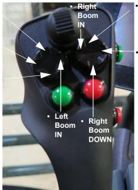
(Located on the Hydrostatic Drive Control Handle) -Typical View
