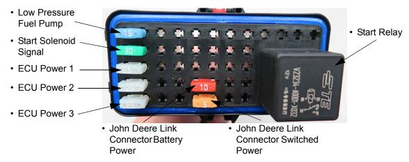
**Fuses (Mini ATM LED):** 5, 10, 15, 25, 30 respective amperage rating. **Start Relay:** 12V/50A SPST mini relay.
