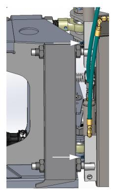
Outer Fold Latch Grease Zerks (4) (Top/Bottom) -Typical View
