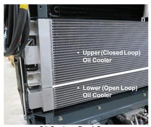
Oil Cooler - **Dual Core**(Located ahead of engine remove radiator screen to access)
