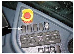
Foam Marker Switch (Located on the side console)
