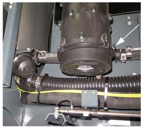
Flow Meter - **Secondary**(Located near the front right-hand side of machine)
