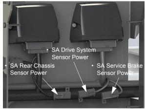
Rear Sensor Power Fuses (Located beneath machine near the rear right-hand tire) -Typical View
