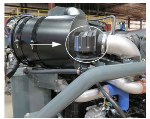
Breather Cap - **STS14/STS16** (Located on rear left-hand side of machine behind air intake filter)
