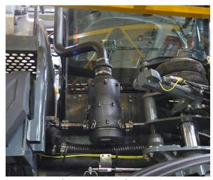
Cab Filtration System (Located on the right-hand side of the exterior cab)
