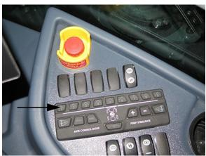
Boom Solution Valve Switches (Located on the side console)
