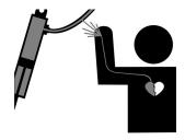
Always lower the load or relieve the pressure before repairing a hydraulic oil leak.
