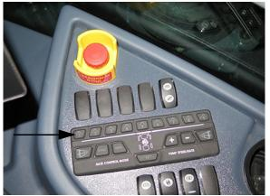
Boom Solution Valve Switches -Single Product Section Keypad, Sections 1-9
