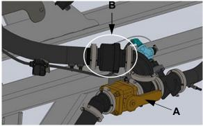
Air Bleed and Check Valves (Located on the center transom frame) -Typical View
