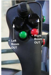
Left and Right-Hand Boom Switches (Located on the Hydrostatic Drive Control Handle) -Typical View
