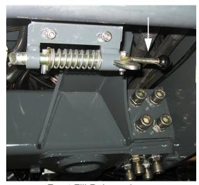
Front Fill Release Lever (Located beneath front end of machine)
