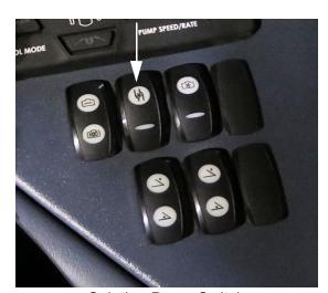
Solution Pump Switch (Located on the side console)
