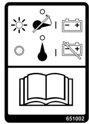
DO NOT TURN BATTERY DISCONNECT SWITCH OFF WHEN FINAL TIER 4 INDICATOR LIGHT IS ILLUMINATED
