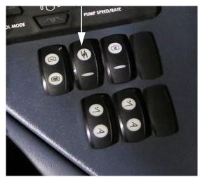
Solution Pump Switch - **Primary** (Located on the side console)
