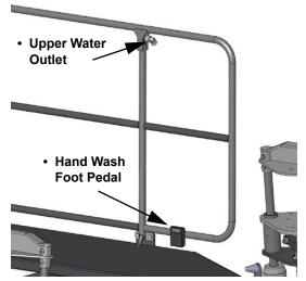
Upper Water Outlet/Hand Wash Foot Pedal (Mounted on left-hand handrail near cab door) -Typical View
