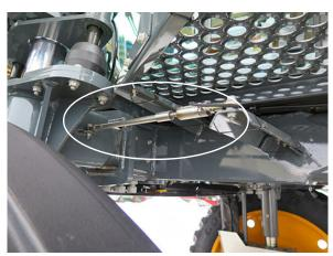
Tread Adjust Sensor (4) (Located on each leg) -Typical View
