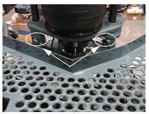
Tower Bearing Grease Zerks (8) (Located on the front and rear legs)
