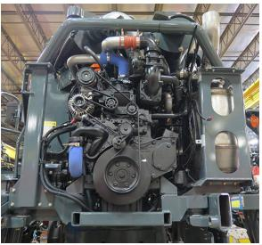
John Deere Final Tier 4 PSS 9.0L Diesel Engine - **STS14/STS16** -Typical View
