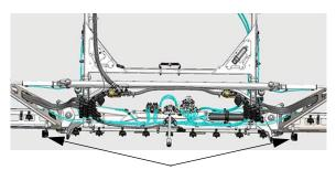
Night Spray Lights (2) - 120' Hybrid Boom (Located on each side of the main boom fold section) -Typical View
