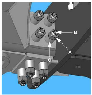
Tread Adjust Plates - Bottom/Side (Located on each leg) -Typical View
