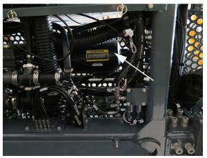
Tank Drain Valve (Air Purge) - if equipped (Located beneath platform near center of machine)
