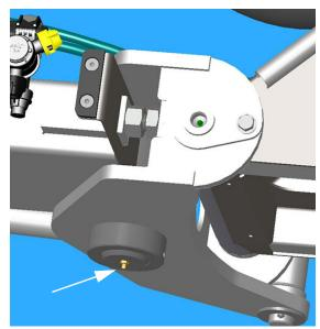
Main Fold Pivot Grease Zerk - Lower (2)
