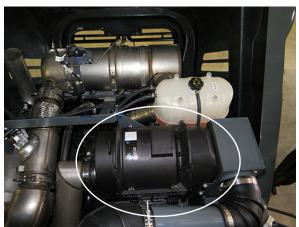
Engine Air Intake Filter - STS10/STS12
