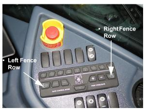
Fence Row Switches - Left/Right (Located on the side console)
