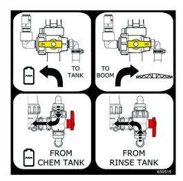
Rotate the Inlet Selector Valve(s)
