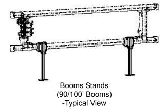
Each boom stand has a leg with a "foot" on the bottom and a hex bolt in the top hole of the leg to secure it from sliding off, as well as a "snap" lock pin in the hole (located directly below the bracket) to maintain it's position.
