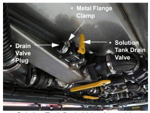
Solution Tank Drain Valve Assembly (Located beneath the solution tank on underside of machine)
