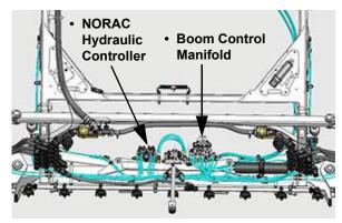
Boom Control Manifold and NORAC Hydraulic Controller (Located near center of inner transom) -Typical View \* 120' Hybrid Spray Booms
