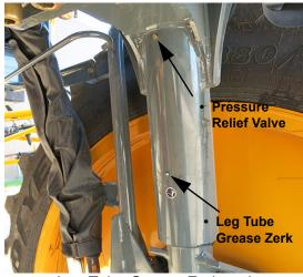
Leg Tube Grease Zerk and
