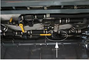
Solution Line Strainer - **Primary**(Located beneath the center right-hand side of machine)
