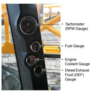
Machine Gauges (Located on cab A-post) -Typical View
