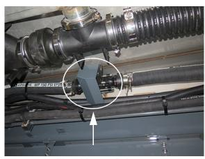
Flow Meter - **Primary**(Located beneath the center right-hand side of machine)
