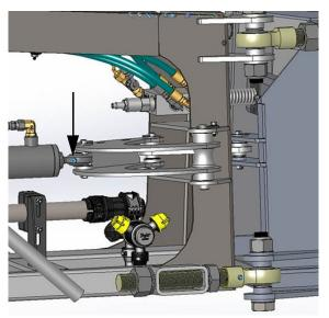
Outer Fold Cylinder Grease Zerk (2)
