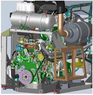
Final Tier 4 Diesel Engine (PSS 6.8L) - STS10/STS12 (Located near rear of machine
