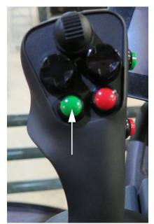
Master Spray Switch (Located on the Hydrostatic Drive Control Handle) -Typical View
