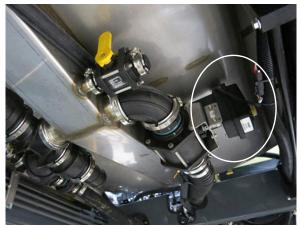
Solution Tank Valve (Located beneath the solution tank on underside of machine)
