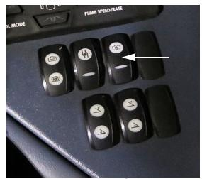
Agitation Valve Switch (Located on the side console)
