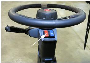
Hazard/Warning Lights Switch (Located on steering column)
