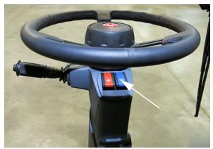
Highway Running Lights Switch (Located on steering column)
