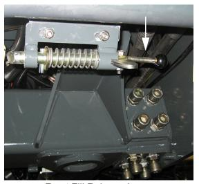
Front Fill Release Lever (Located beneath front end of machine)
