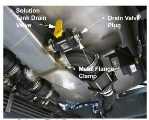
Solution Tank Drain Valve Assembly (Located beneath the solution tank on underside of machine)
