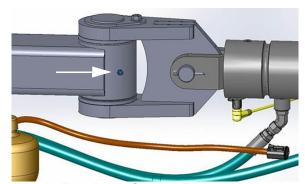
Main Fold Pivot Grease Zerk - Upper (2)
