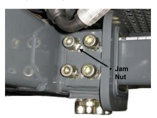
Tread Adjust Bearing Bolts - Bottom/Side (Located on each leg)
