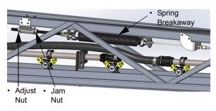
Spring Breakaway Adjust/Jam Nuts (Located near the outer end of the spring breakaway) -Typical View
