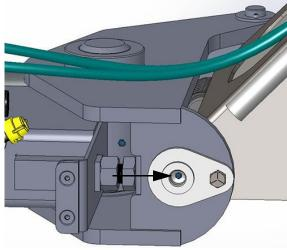
Level Pin Grease Zerk (4)
