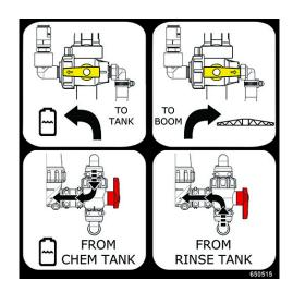
When pump calibration is complete, rotate the Outlet Selector Valve(s) to the "TO BOOM" position to send chemical to the Mixer Assembly.
