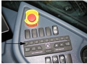
Boom Solution Valve Switches Single Product Section Keypad
