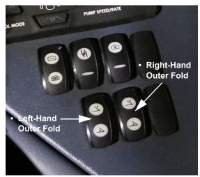
Boom Extension Switches - Left/Right (Located on the side console)
