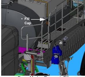
Foam Marker Reservoir Fill (Located on the rear right-hand handrail)
