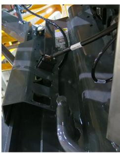
NORAC Connection (Located on the front right-hand side of machine) -Typical View
