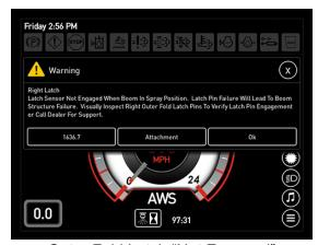
Outer Fold Latch "Not Engaged" Malfunction Warning
