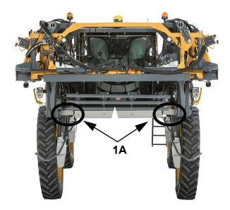
Attach two (2) suitable chains or straps to the rear axle tubes (as close to the mainframe as possible). These chains/ straps will be used to brake the machine once it is moving, as the machine will not be capable of stopping itself.
