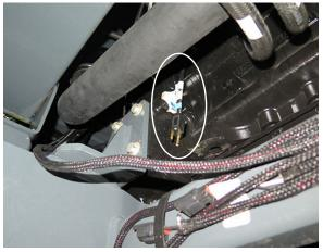
Engine Block Heater Power Cord
