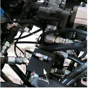
Solution Pump Control Manifold (Located near center of machine)
