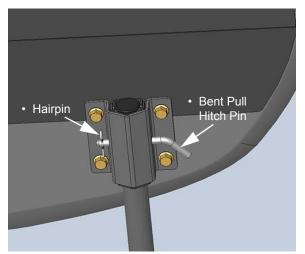
Hairpin/Bent Pull Hitch Pin Assembly (Located on each left and right-hand hood bracket)
