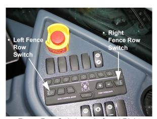
Fence Row Switches - Left and Right (Located on the side console)
