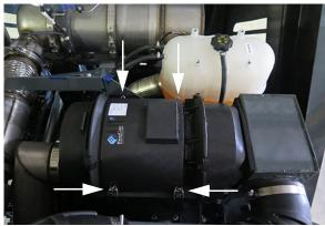
Security Latches (4) - **STS10/STS12** (Located on each side of filter housing) -Typical View
