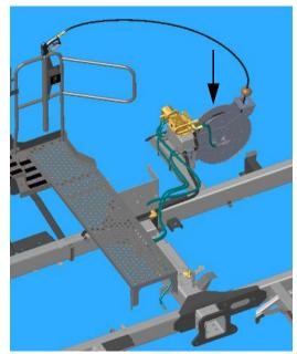
Pressure Washer Hose Reel (Located near the rear right-hand side of machine) -Typical View
