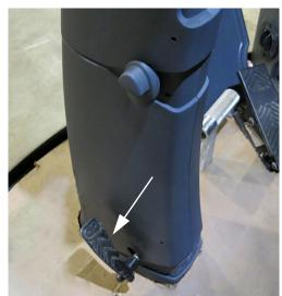
Steering Column Release Pedal (Located on the lower left-hand side of the steering column)
