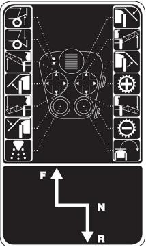
Hydrostatic Drive Control Handle
