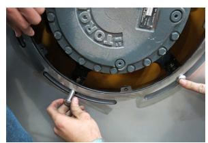
Wheel Cover Mounting Bolt Installation
