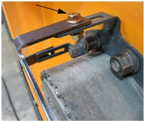
Hub Cap Adapter Bolt Installation
