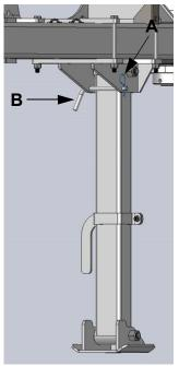
Lock Pin Reinstalled -Typical View
