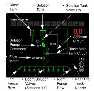
Solution System Schematic Screen
