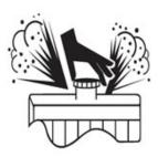
Disconnect battery ground cable and turn the Battery Disconnect Switch OFF before servicing the electrical system or welding on the machine.
