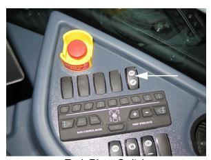
Tank Rinse Switch (Located on the side console)
