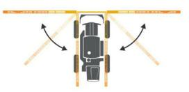
NOTE: When boom reaches the last 8-10 degrees of travel, it will automatically slow down to avoid impact with the cradle.
