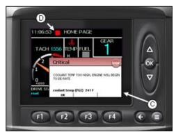
When this warning appears, the machine may be severely limited in engine and hydraulic functions to prevent damage to those systems. The warning will disappear and the buzzer will go off by pressing F2 to clear, but it does not correct the problem. The red warning light at the top (D) will continue to flash until the fault is resolved.
