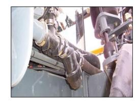
Solution Line "Y" Strainer-To help maintain consistent application rates, check the solution line strainer daily for blockage. Clean the strainer screen as required. Be sure to wear appropriate clothing while removing and cleaning the line strainer screen. Confirm the gasket is in place before re-installing the screen.
