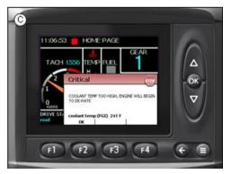
To toggle between the two drive states, make sure there are no drive faults present and that the machine is in neutral. Press the F1 button until the desired drive state appears below "Drive State" on the display screen.
