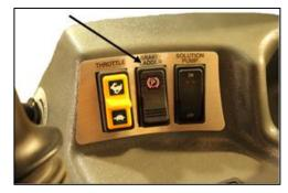
complete stop with the hydrostatic lever in the neutral position before applying the parking brake.
