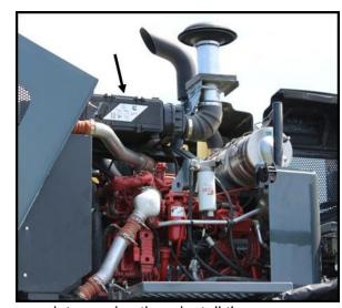
Cleaning- It is not recommended to clean the air intake filter element. However, a clean damp cloth should be used to wipe away dust and foreign material from the air cleaner housing.
