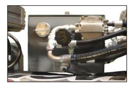
*Fill Screen*-Replace the fill screen immediately if there are any signs of a tear or break. The screen is the first defense against foreign materials entering the tank.
