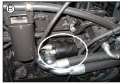
Caution: Always use caution when dealing with hydraulic circuits containing accumulators. These circuits can have trapped pressure even when some parts of the circuit are not pressurized.
