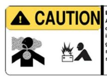
Batteries contain sulfuric acid. Avoid contact with skin, eyes, or clothing. Do not inhale fumes or ingest liquid. Batteries contain gases which can explode. Keep sparks and flame away while servicing.
