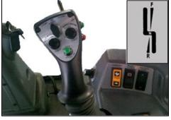
To move the machine in reverse, move the lever to the far right and slowly pull back. The farther back the lever is pulled, the faster the machine's speed.
