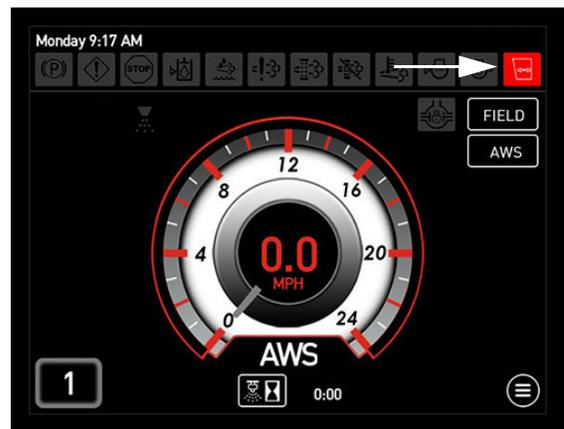
Insufficient Cab Air Pressure Indicator
