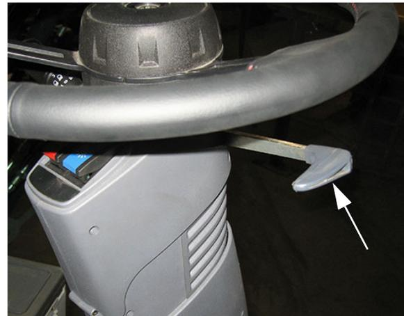
Steering Wheel Telescope Adjust Handle
