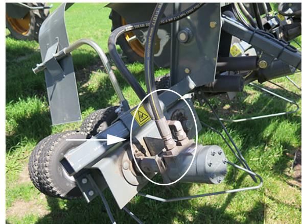
Quad Puller Hydraulic Connections
