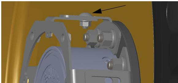
Hub Cap Adapter Bolt Installation
