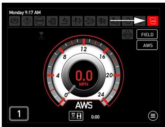
Insufficient Cab Air Pressure Indicator
