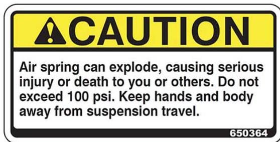
*NOTE: Visually inspect the height of each air bag daily. Measure height of each air bag (using a tape measure) every 50 hours of operation. Adjust as necessary.*
