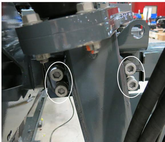
Tread Adjust Bearing Bolts - Top/Side
