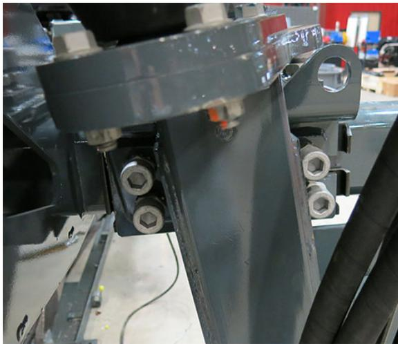
Tread Adjust Bearing Bolts - Top/Side
