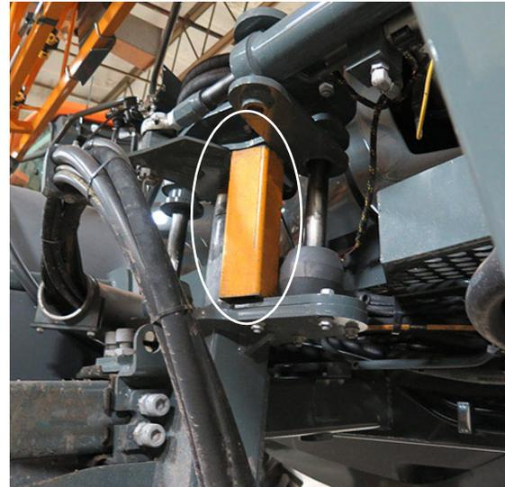
Steel Tube Installed Beneath
