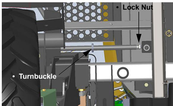
Tread Adjust Turnbuckle Rod
