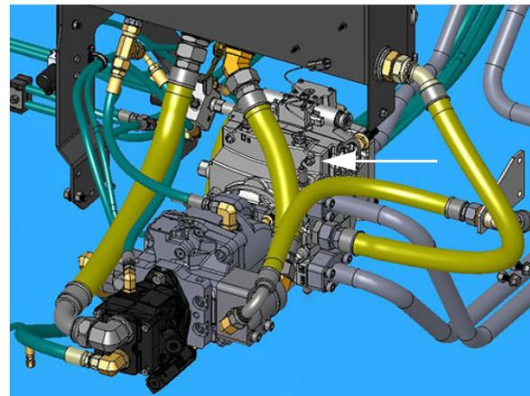
Hydrostatic Pump (Drive Pump)
