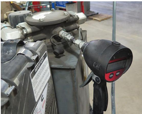
Filling Tank Through Hydraulic Oil Fill Port
