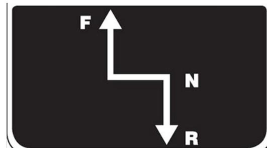
Hydrostatic Drive Control Handle
