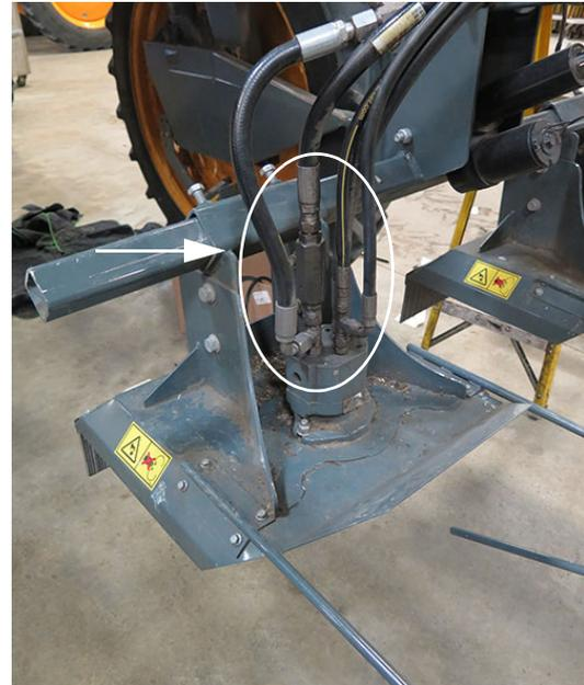
Cutter Head Hydraulic Connections
