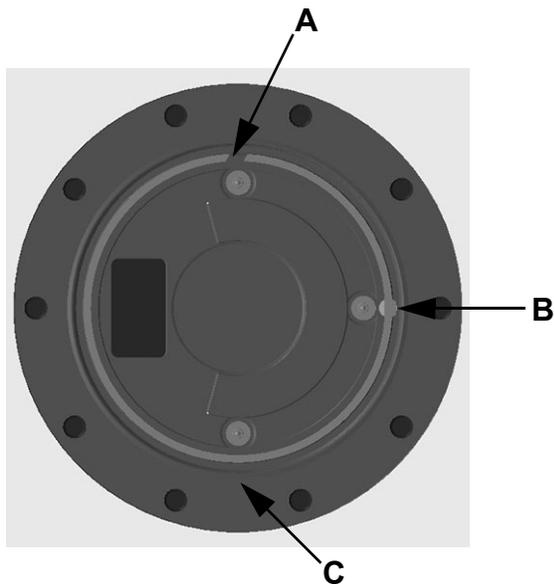
2. Using a 1/4" ball end Allen wrench, remove the 3 o'clock plug (B). If no oil comes out, proceed to Step 3.
