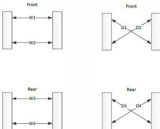
9. Continue to cycle between Steps 5-6 and 7-8 until the width measurements match and the diagonal measurements match. Then and only then are the wheels parallel to each other and the frame.
