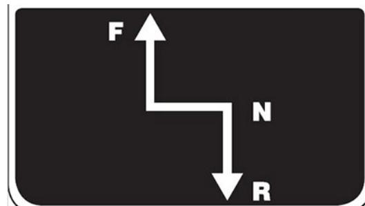
Hydrostatic Drive Control Handle
