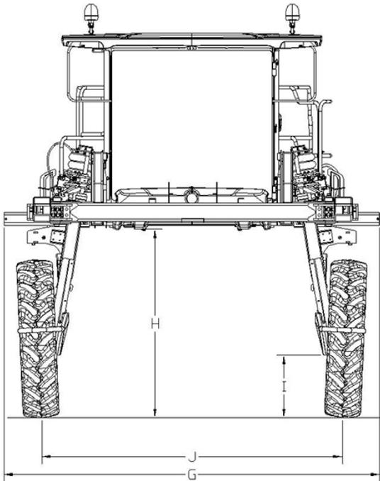
\* Tread width is measured from center of tire at ground.
