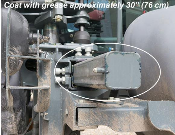
Tread Adjust Bearing Slide Path (4)
