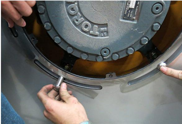
Wheel Cover Mounting Bolt Installation
