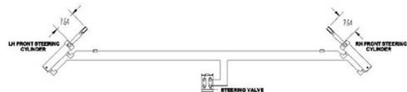
11. With the cylinders centered, adjust the tie-rods (located on the cylinder rods) until they line up with the bolt-down hole (located on the lower air bag plate).
