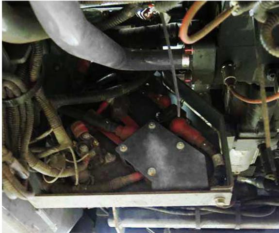
Final Tier 4 Engine Fuse/Relay Block
