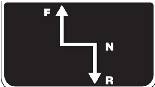
Hydrostatic Drive Control Handle
