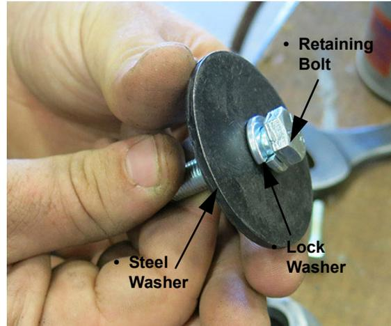
Cutter Blade Bolt/Washer Assembly
