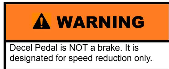
When nearing an end row and speed deceleration is desired, press the Decel Pedal (located to the lower right-hand side of the steering column) to decrease speed.
