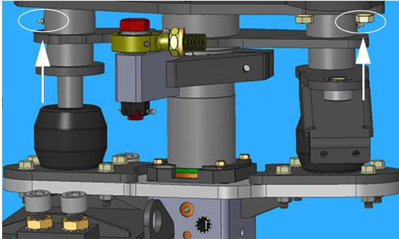
Tower Bearing Grease Zerks
