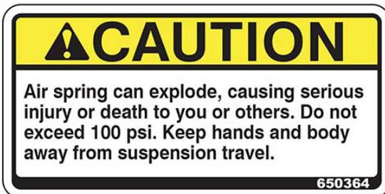
*NOTE: Inspect air bags daily for leaks and/or cracking.*
