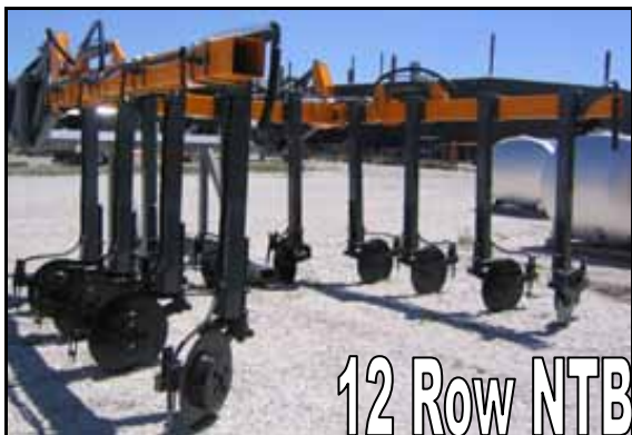
Figure 14: Folded position for 12 and 16 row NTB
