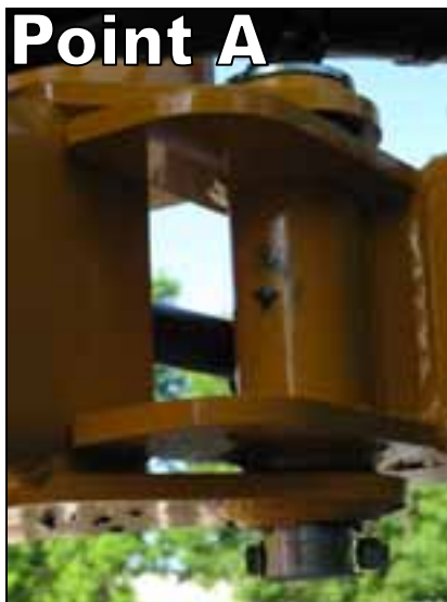
Figure 22: Grease point A -main toolbar fold
