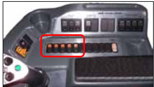
Figure 10: Spray section switches
