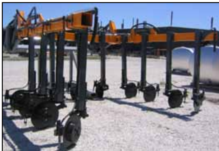
Figure 1: Folded position for 12 row NTB
