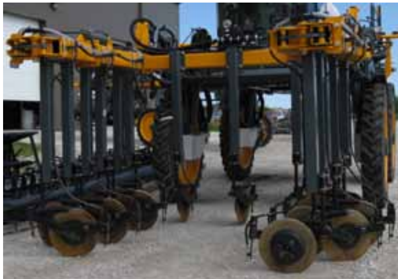
Figure 2: Folded position for 16 row NTB
