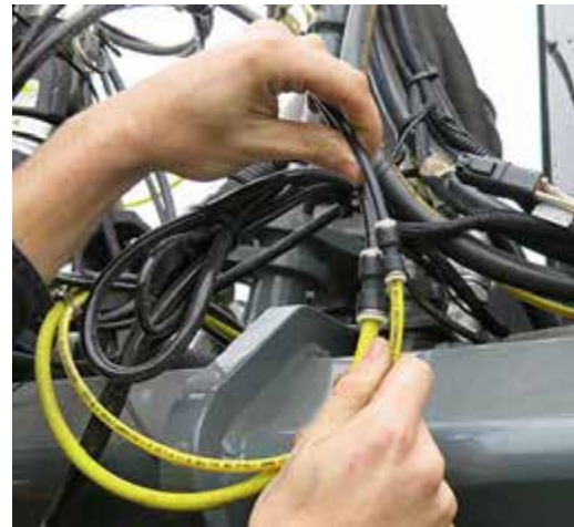
Foam Marker Connection (Located on front right-hand side of machine) -Typical View
