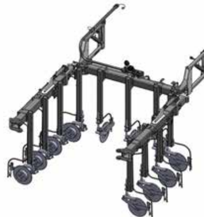
30' NTB Fold Points (Folded position shown) -Typical View
