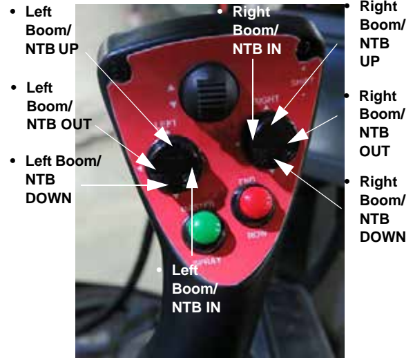
Left and Right Boom/NTB Switches (Located on the Hydrostatic Drive Control Handle) -Typical View
