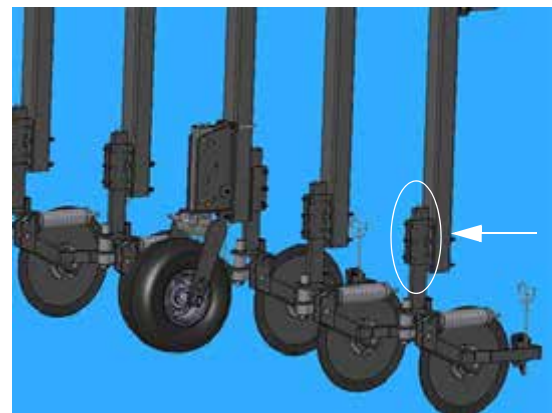
Mounting Bolts (Located on the side of the coultter mounting plate) -Typical View
