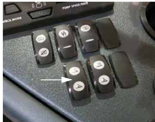
Boom/NTB Extension Switch (Located on the side console) -Typical View
