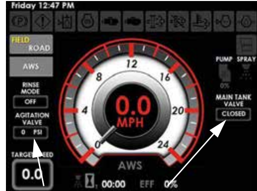
• Agitation Valve Pressure • Main Tank Valve Status
