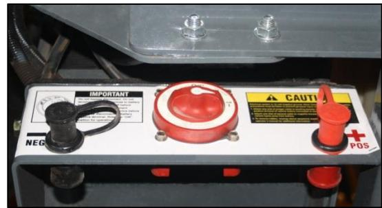
This device is also used an anti-theft safeguard. Keep the key in a safe place, out of the machine when it is not in use.
