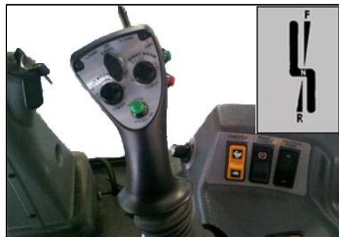
To stop the machine, or put the machine in neutral, slowly pull the lever back to the center position and move it slightly to the right. The neutral position must be met before changing direction of the machine. The machine must also be in neutral before several functions can be performed.
