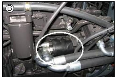
**Caution:** Always use caution when dealing with hydraulic circuits containing accumulators. These circuits can have trapped pressure even when some parts of the circuit are not pressurized.
