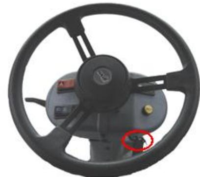
momentarily until the engine engages. If the engine does not engage after 15 seconds, turn the key to OFF. Constant cranking of the starter when an engine fails to engage will cause damage to the battery and the starting system. Refer to the section on the hydrostatic drive for more information.
