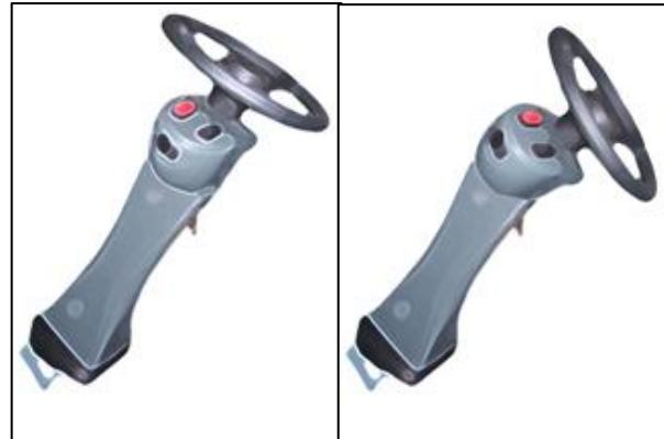
With the handle loosened, push or pull on the steering wheel until it is in a comfortable position. Hold the steering wheel in that position while tightening the adjustment handle. To tighten the handle, turn it upward (away from the operator).
