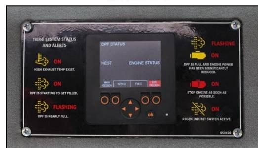
The third function is to display any engine faults that may be taking place.
