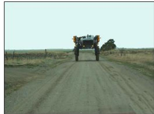
**Caution:** Hagie Manufacturing Company does not recommend any form of transportation other than driving the sprayer. Loading the sprayer onto a trailer may result in sprayer rollover.
