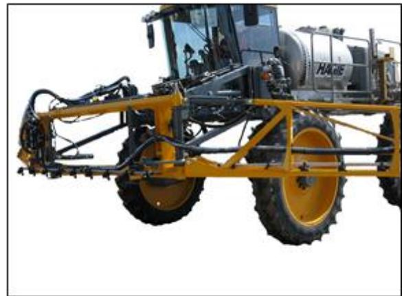
If temporarily storing the boom on a soft surface, such as grass, it may be necessary to put blocks under the stand's feet to prevent the attachment from sinking into the ground. It is not recommended that booms be stored on a soft surface for an extended period of time because of the risk of the soil settling even when blocks are used.
