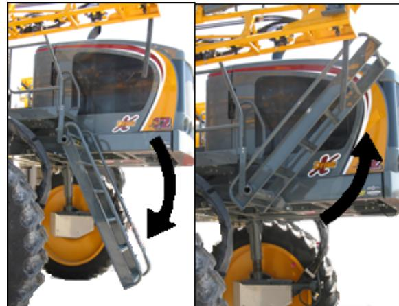
**! Caution:** Upright ladder is not a service platform or step. DO NOT step on the ladder while in upright position. DO NOT lower the ladder while anyone is on the ground near the sprayer. DO NOT attempt to lower the ladder from the ground level.
