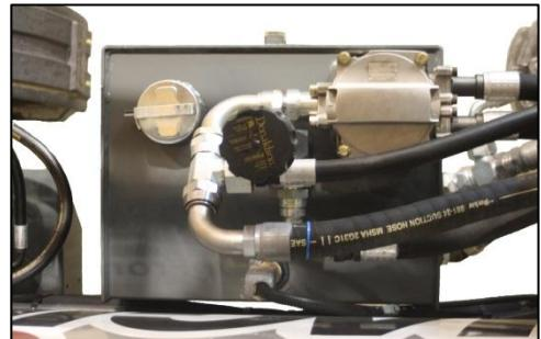
*Fill Screen*-Replace the fill screen immediately if there are any signs of a tear or break. The screen is the first defense against foreign materials entering the tank.
