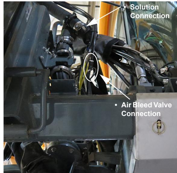
Solution and Air Bleed Valve Connections -
