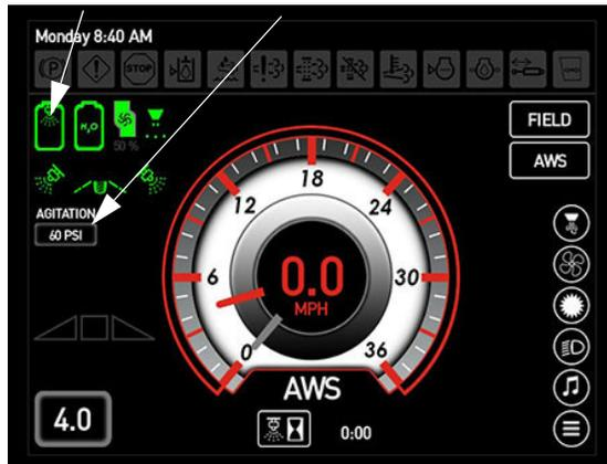
Main Tank and Agitation Valve Pressure Indicators
