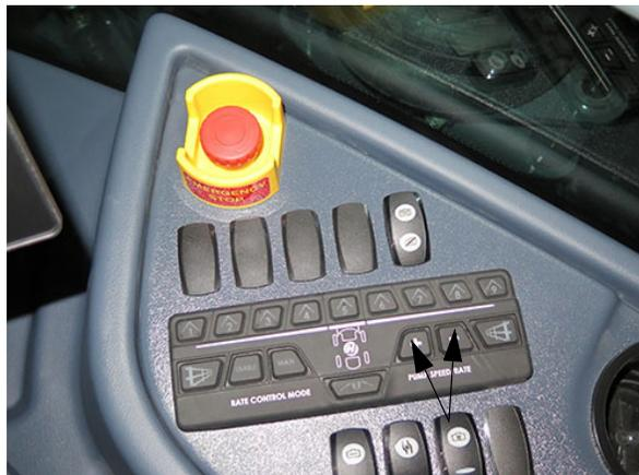
Pump Speed/Rate Switches
