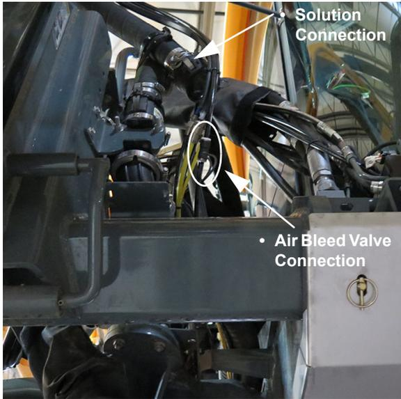
**Solution and Air Bleed Valve Connections -
