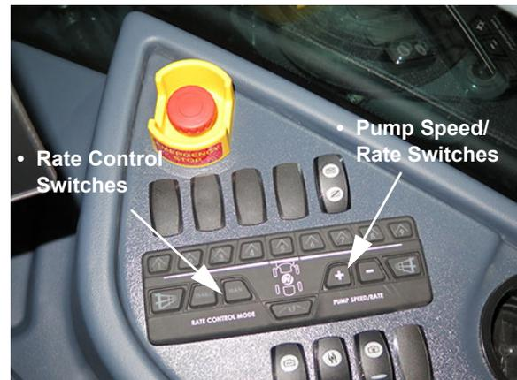
Rate Control and Pump Speed/Rate Switches
