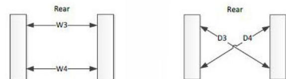
9. Continue to cycle between Steps 5-6 and 7-8 until the width measurements match and the diagonal measurements match. Then and only then are the wheels parallel to each other and the frame.
