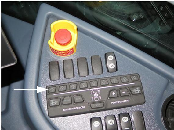
Boom Solution Valve Switches
