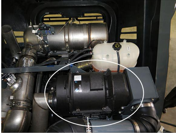
Engine Air Intake Filter - **STS10/STS12**
