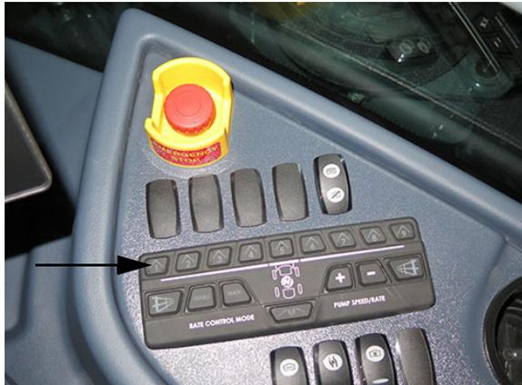
Boom Solution Valve Switches
