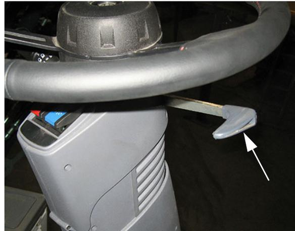
Steering Wheel Telescope Adjust Handle
