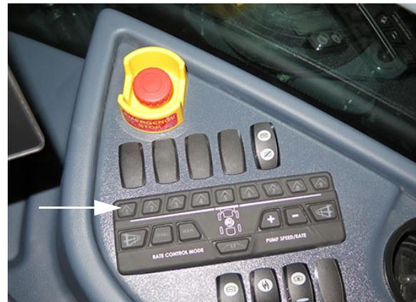
Boom Solution Valve Switches
