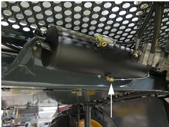
Tank Drain Valve (Main)
