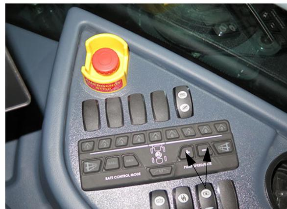
Pump Speed/Rate Switches
