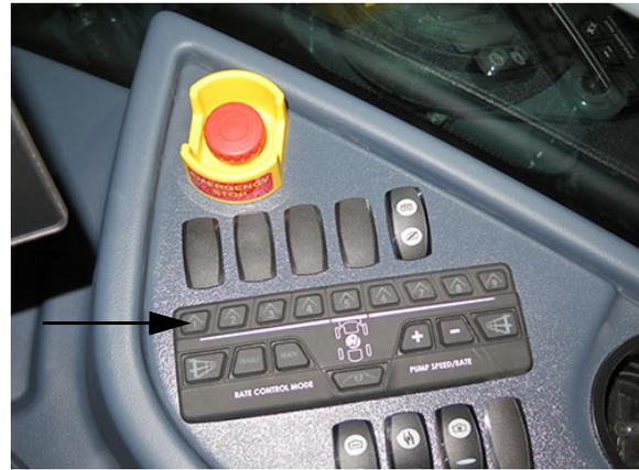
**Boom Solution Valve Switches -
