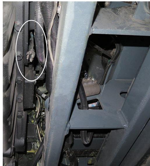
Engine Block Heater Power Cord
