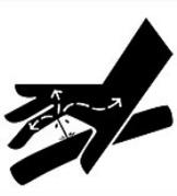
Avoid serious injury from contact with hydraulic oil and gas under pressure. Before removing hydraulic components, disassembling or changing accumulators:
