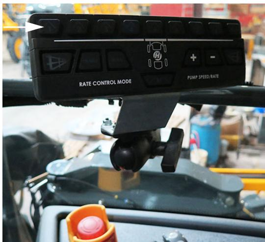
Boom Solution Valve Switches -
