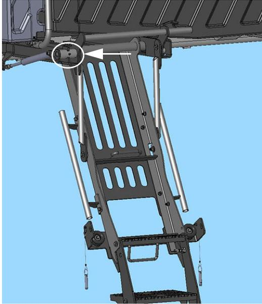
Gas Spring Axle Grease Zerk
