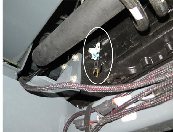
Engine Block Heater Power Cord
