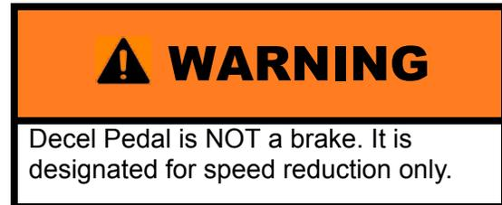
When nearing an end row and speed deceleration is desired, press the Decel Pedal (located on the lower right-hand side of the steering column) to decrease speed.
