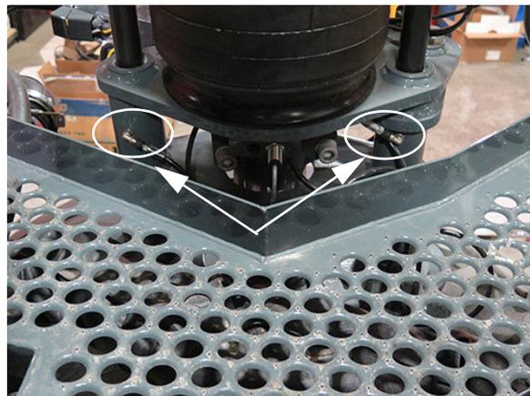
Tower Bearing Grease Zerks (8)
