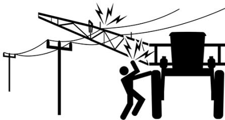
As a safety precaution, a Power Line Warning Message will appear on the Machine Display before extending the outer boom extensions. Press **ACKNOWLEDGE** showing that you have acknowledged that there are no overhead power lines or obstructions before proceeding.
