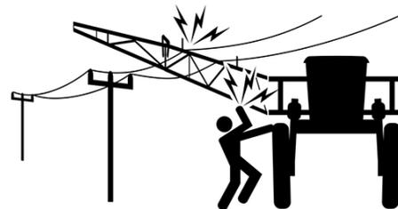
As a safety precaution, a Power Line Warning Message will appear on the Machine Display before extending the outer
