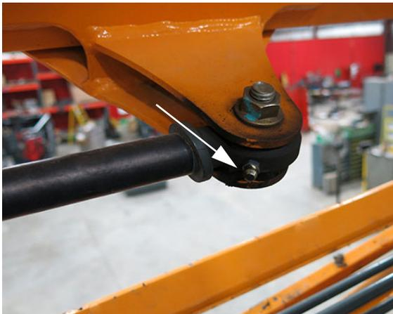
Boom Breakaway Cylinder Rod End
