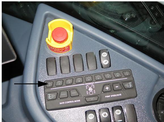
Boom Solution Valve Switches
