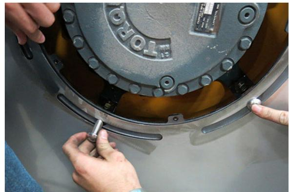
Wheel Cover Mounting Bolt Installation
