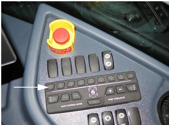
**Boom Solution Valve Switches**
