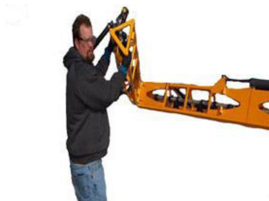
3. Secure into place with the rear Securement Bolt.
