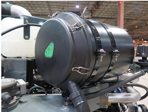
Engine Air Intake Filter - **STS14/STS16**
