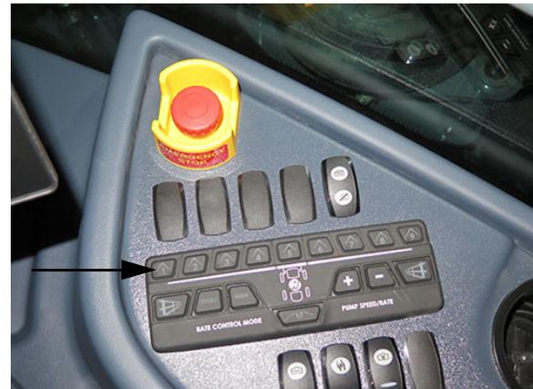
Boom Solution Valve Switches -
