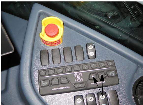
**Pump Speed/Rate Switches**
