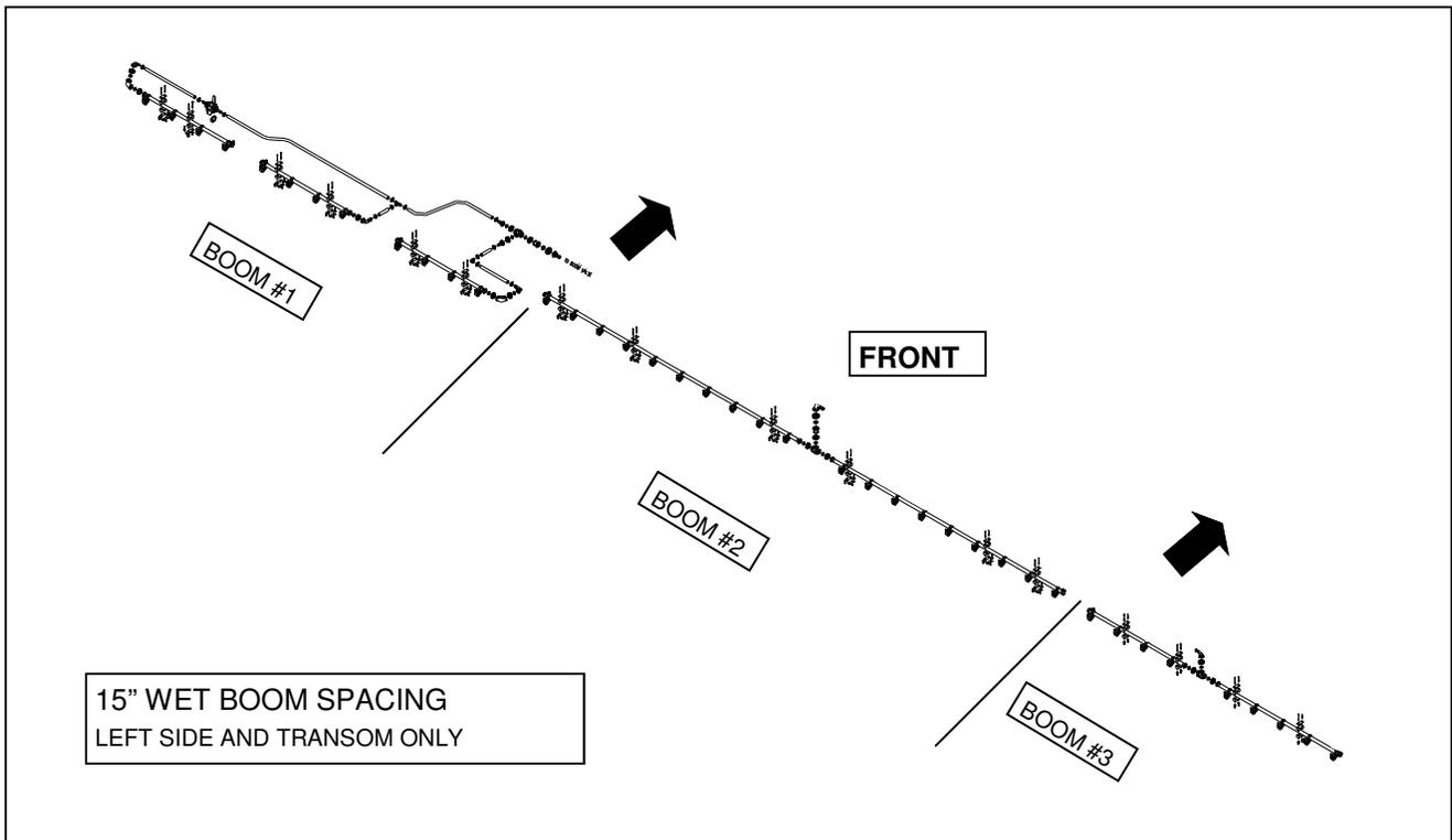
The difference between the dry boom (previous page) and the wet boom is that the dry boom's section 3 includes 4 nozzles on either side of the transom that are not included in the in the same section of a wet boom.
