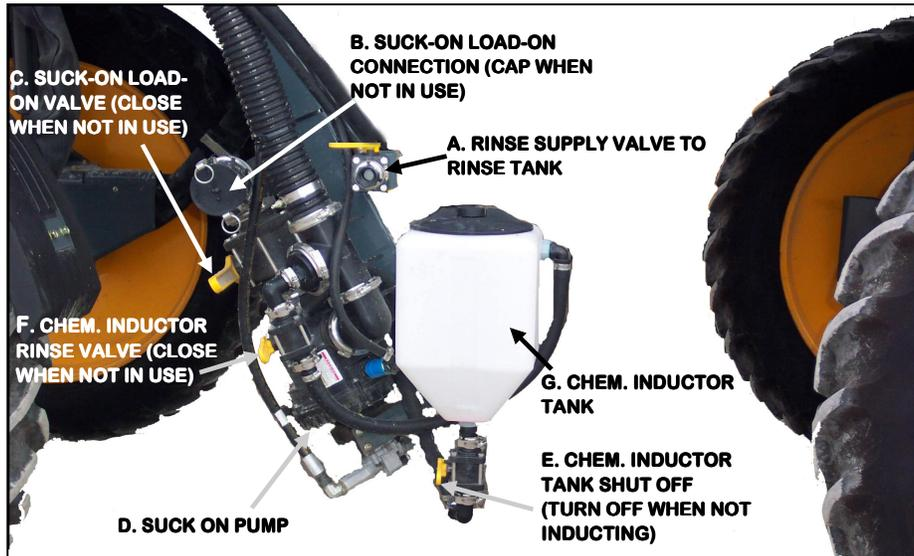
With the engine running and the parking brake set, flip the lock switch up (H). Lower the inductor assembly with the inductor control box switch (I). If filling with the suck-on attachment, leave the engine running. If filling with the push-on attachment, turn the engine off.
