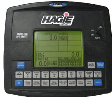
Enter the speed that you wish to simulate using the 1-0 keys. Verify the speed in the lower corner of the display. The self test speed will clear itself when motion of the vehicle is detected. A speed cal value of 900 or greater is recommended when operating in this mode.
