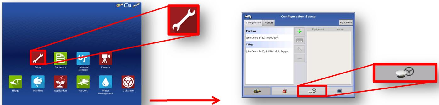
3. Plug USB memory stick into Ag Leader Integra/Versa/Compass v6.8+ and select the “Double ended wrench” icon from the Home screen. Then, select the “GPS/Guidance Setup” icon.
