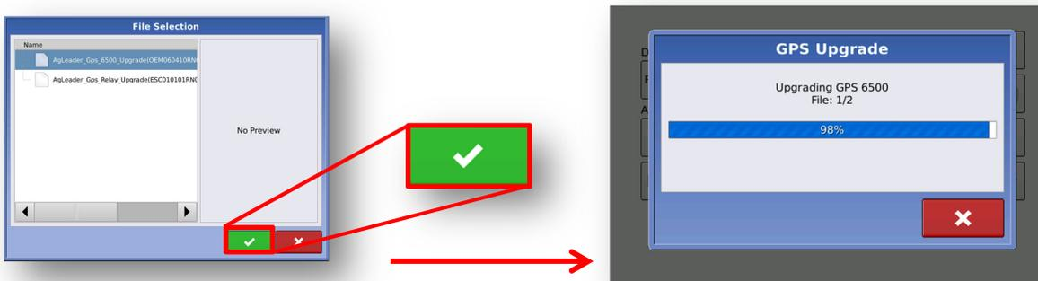
7. Access the File Selection page to start the Relay upgrade process (as seen in step 4). Locate and highlight blue “AgLeader\_Gps\_Relay\_Upgrade(ESCXXXXXXXXXXXXX\_inc).fw3” file. Continue file selection and begin the Relay upgrade process by selecting the “Green Check” icon. To exit File Selection, select the “Red X” icon. (Note: This upgrade process will take approximately 40 minutes to complete.)
