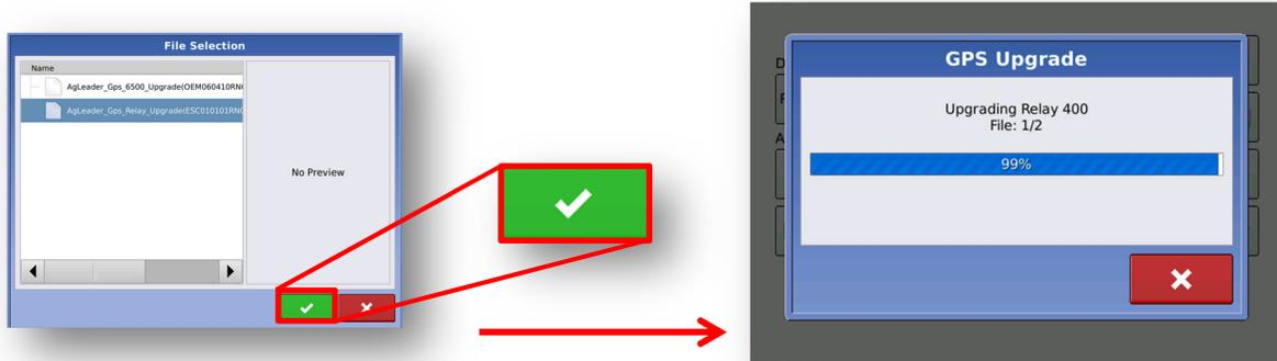
8. Once both upgrades are complete, the GPS 6500 and Relay are now updated, but will need to be “Reset to Defaults.” This will reset the GPS 6500 Relay back to default settings. “Reset to Defaults” is required for the GPS 6500 function properly after upgrade (must be on 6.8+ firmware).
