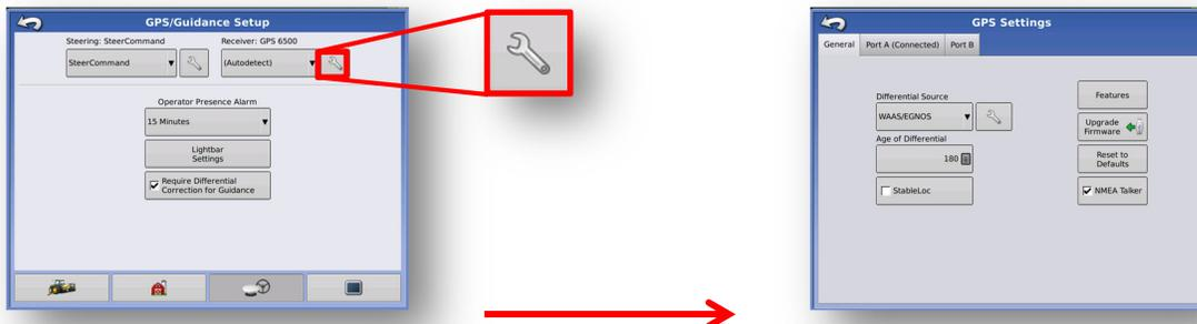
5. From the GPS Settings page, select the “Upgrade Firmware” button to upgrade the GPS 6500 and Relay. File Selection Screen will now populate. (Note: If “Upgrade Firmware” button is not accessible, USB memory stick is not recognized by display.)
