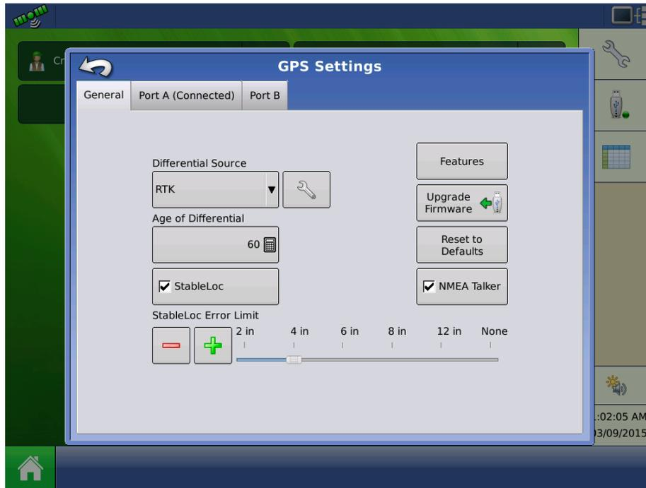
Figure 1 - StableLoc Error Limit Setting
